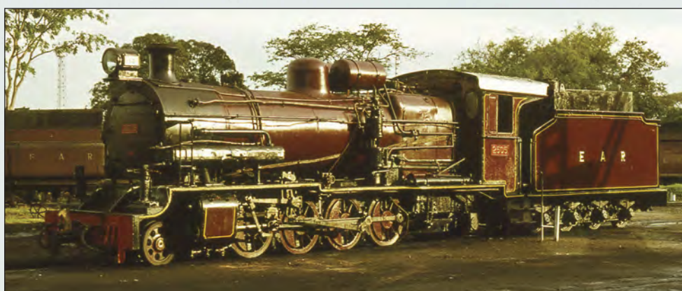
Top: Class 56 no 5603 outside the shed at Dar es Salaam, showing the full splendour of Dar works painting and lining. The 4-8-2+2-8-4 Garratt was built by Beyer Peacock in 1949. The Class 56 was generally held to be the best class on East African Railways. December 1969.
