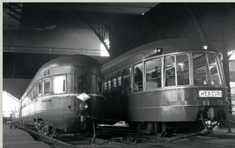
STREAMLINER CONTRASTS: The observation cars of IC's Green Diamond (left) and NYC's Chicago Mercury stand in the old trainshed at IC's Central Station on November 4, 1939. Although both designs dated from 1936, the IC train consisted of all-new articulated lightweight cars, while the Mercury was rebuilt from heavyweight coaches.
