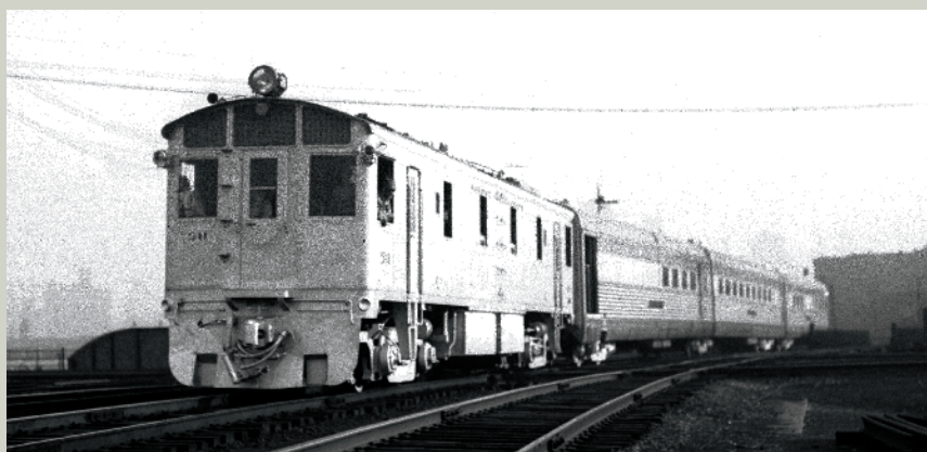
DEMO ON A SPECIAL: The first of Electro-Motive's five box-cab passenger diesels of 1935 were Nos. 511 and 512, which the builder used for testing and as demonstrators. Here the 511 is outbound on the Rock Island at 16th Street with a special train of three Rocket cars.
