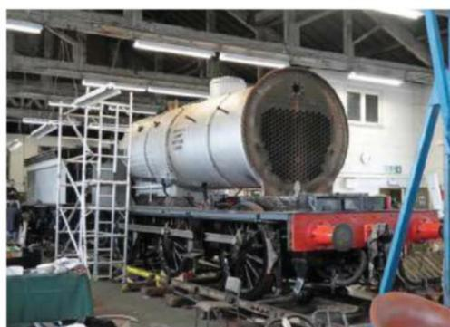
← **'J27' 0-6-0 No. 65894 with its boiler back in the frames at NELPG's Darlington Hopetown Works on July 15.**
