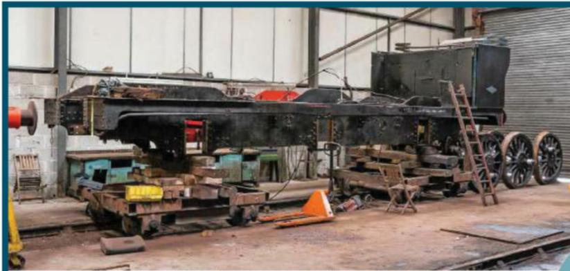
← Being lined up for a return to steam next year, No. 47357 is under overhaul at the Midland Railway - Butterley on July 14. Note the distinctive diamond-shaped North British worksplate on the bunker. ALAN WEAVER
