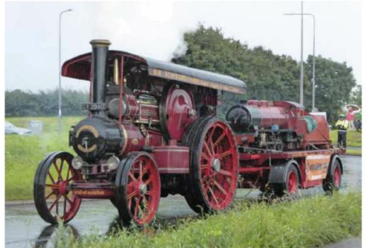
With *Whillan Beck* in tow, Fowler road locomotive *Providence* battles driving rain as it joins the A596 on the first leg of its journey to Ravenglass. The traction engine would later be stopped with leaking boiler tubes, the same problem that afflicted the machine 51 years previously when delivering *River Mite* to the RER. KEITH HERBERT
