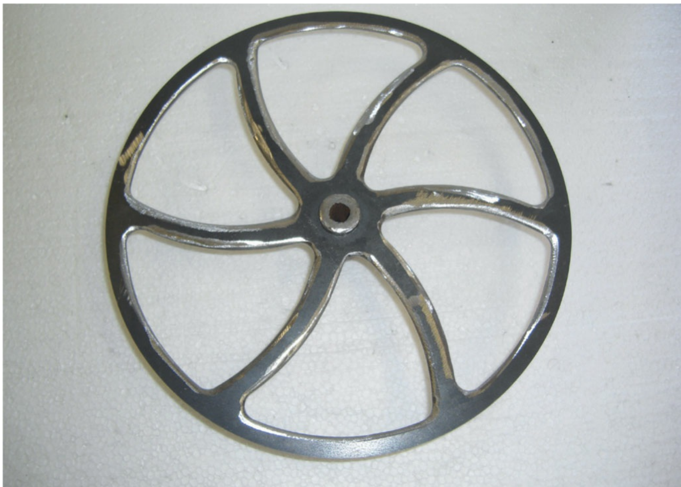
Spokes carefully dressed with an angle grinder
