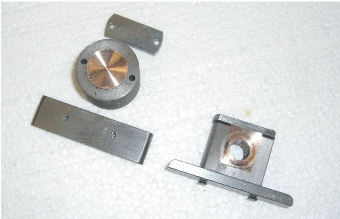
Crankshaft bearings.
