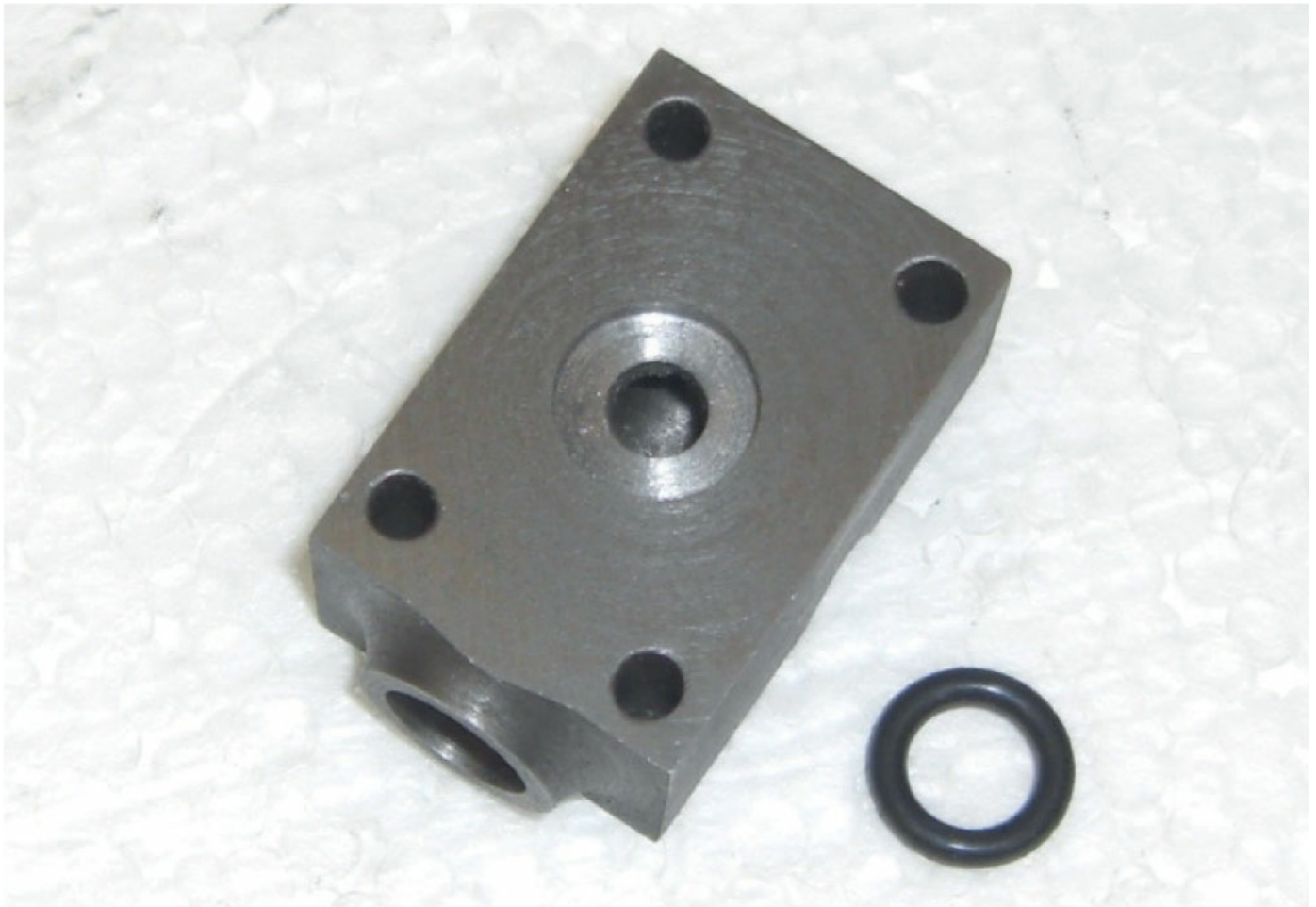
Passages in regulator chamber counterbored for 'O' rings
