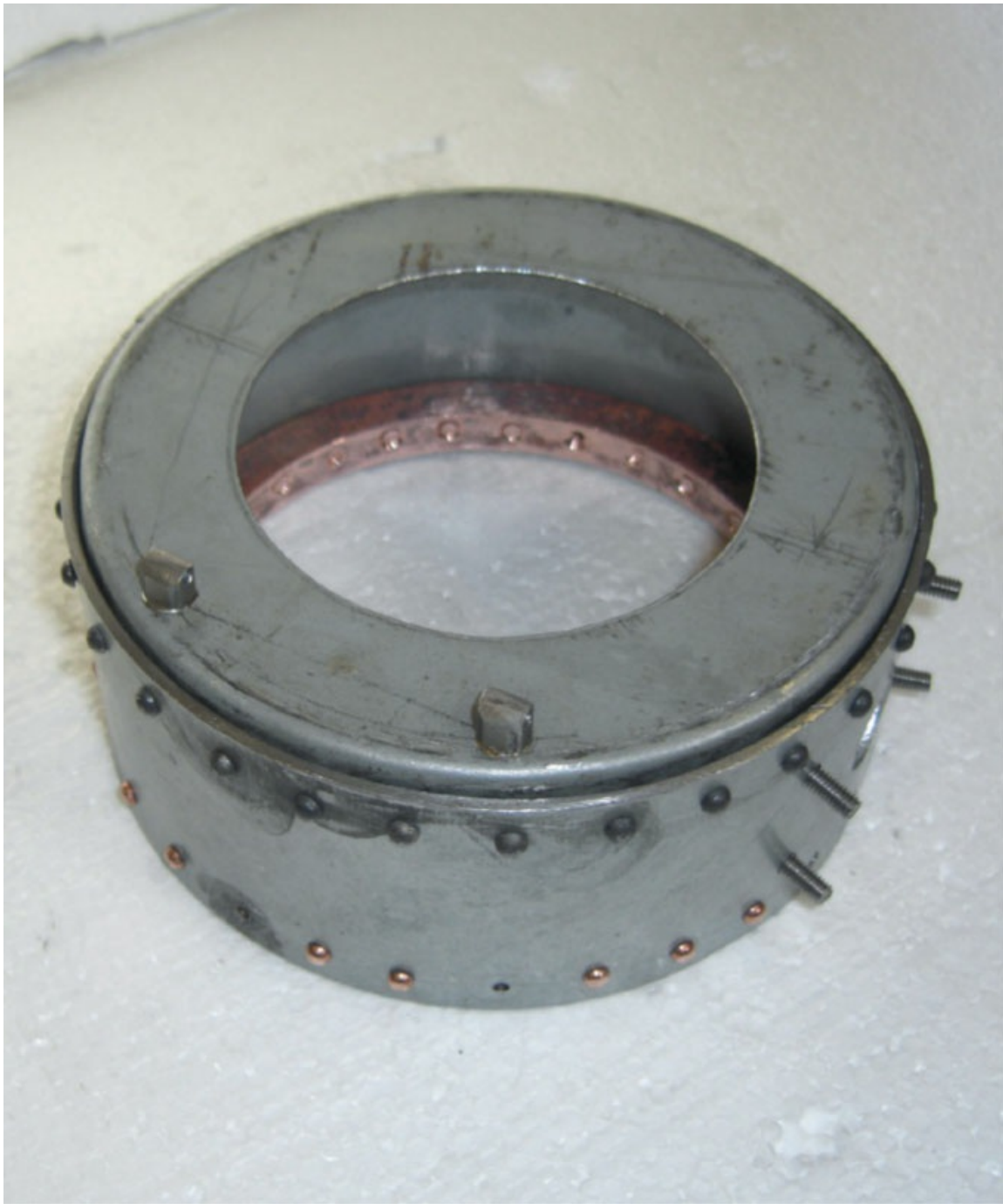
Front plate riveted to smokebox.
