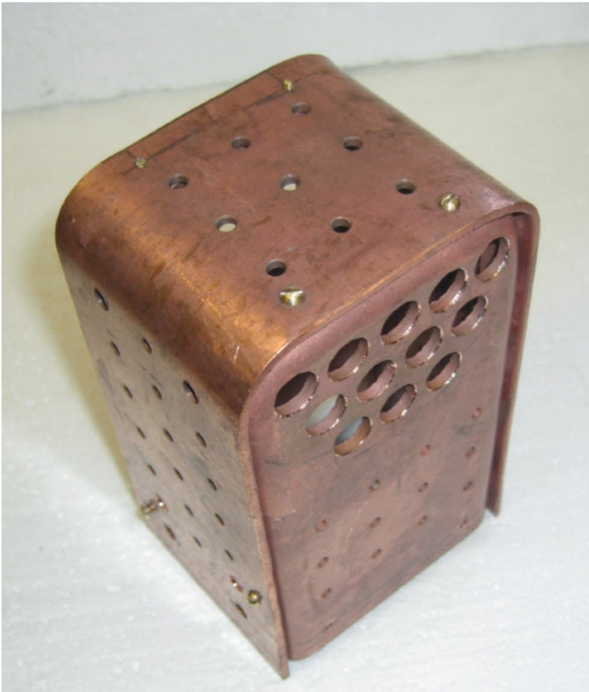
Firebox wrapper and tube plate.
