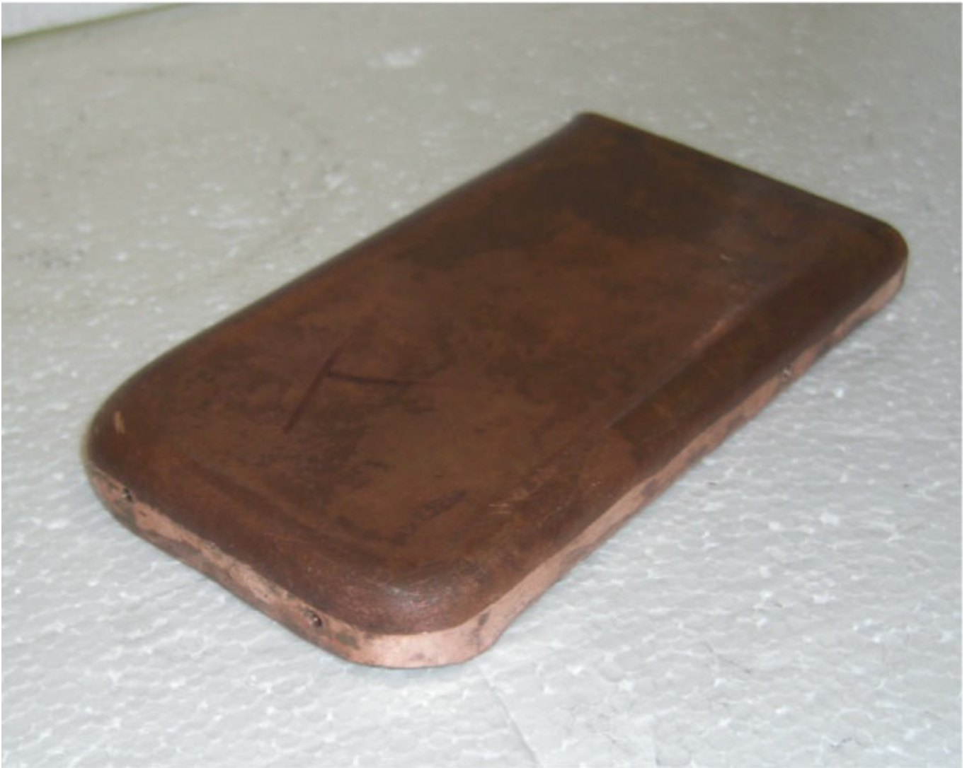
Inner firebox door-plate.
