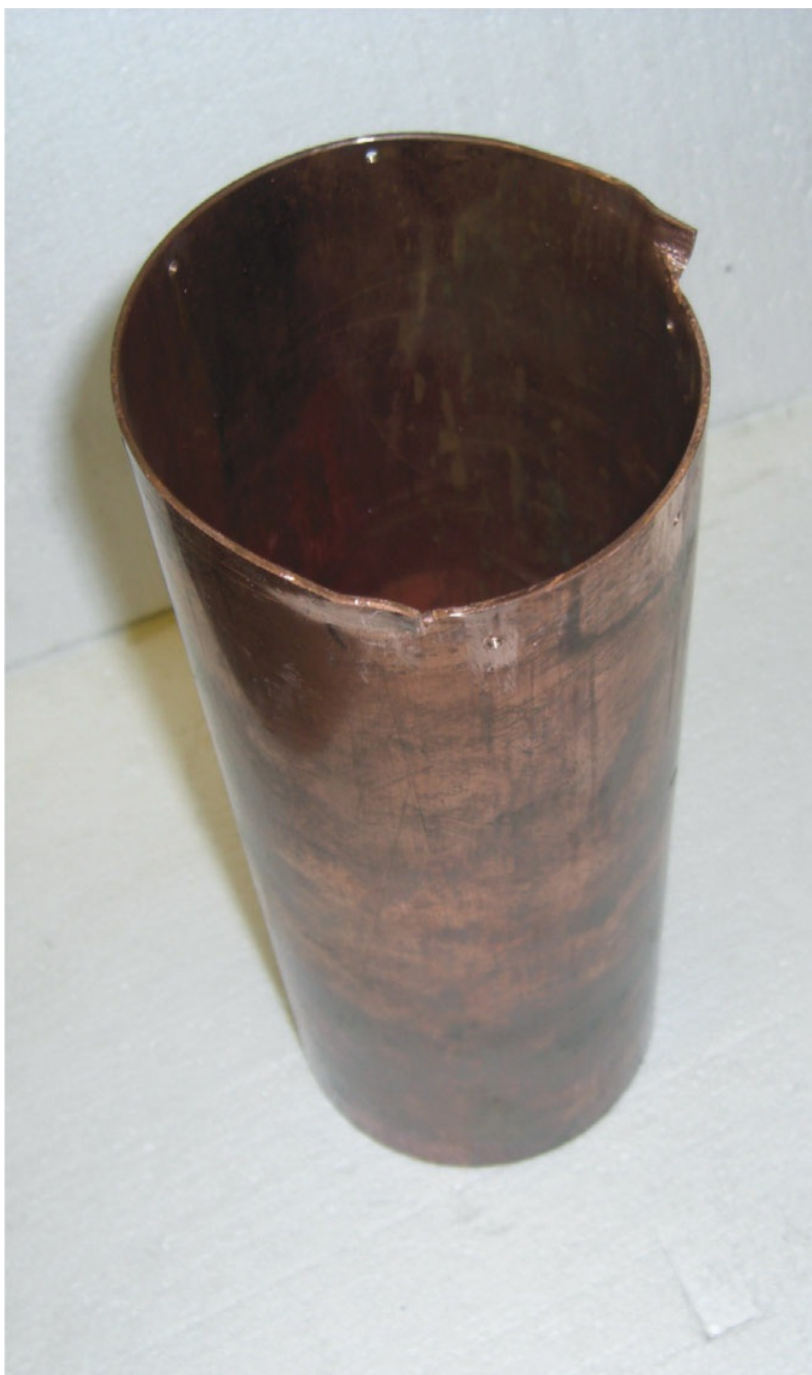
End of barrel tube cut back and shaped on trial assembly.
