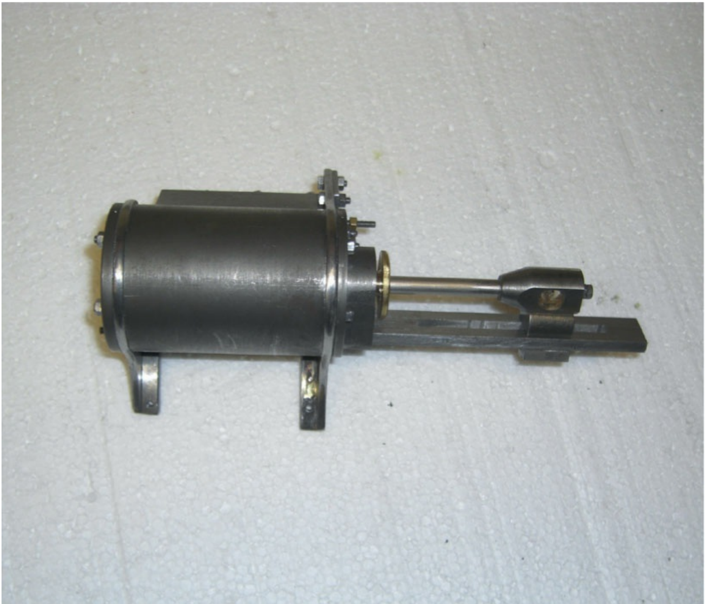
Cylinder assembled with crosshead.
