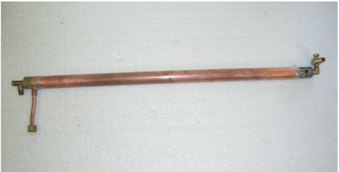
Complete feed-water heater.
