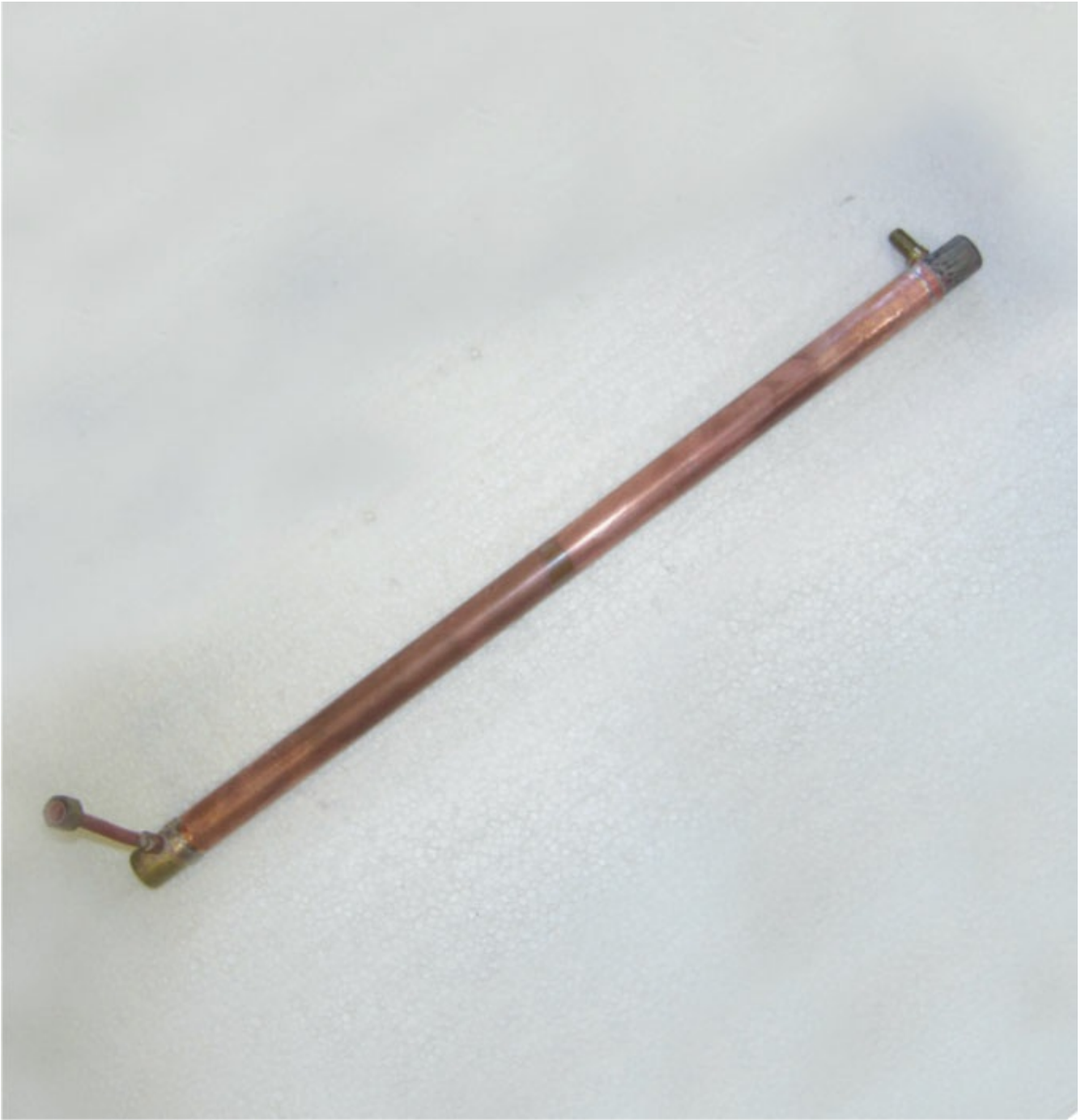
Feed-water heater outer tube.
