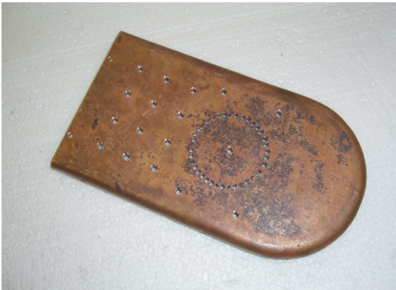
Door-plate with fire-hole chain drilled.
