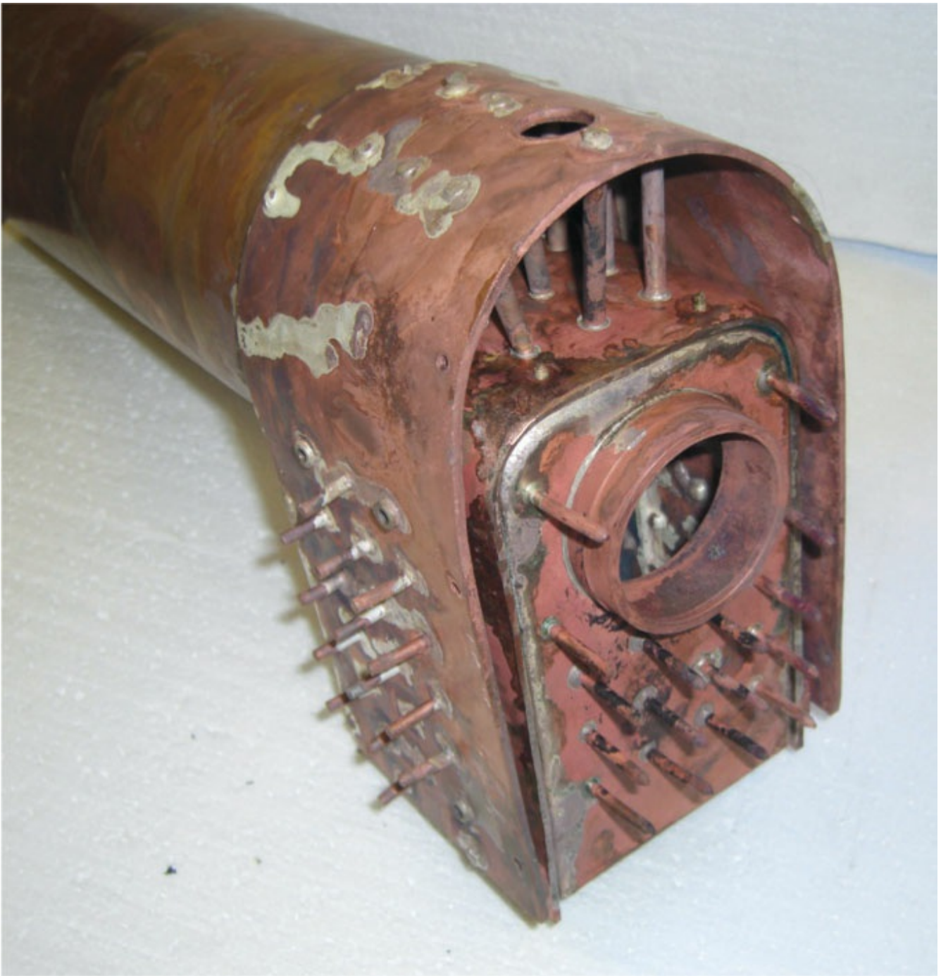
Firebox door-plate silver soldered in place.
