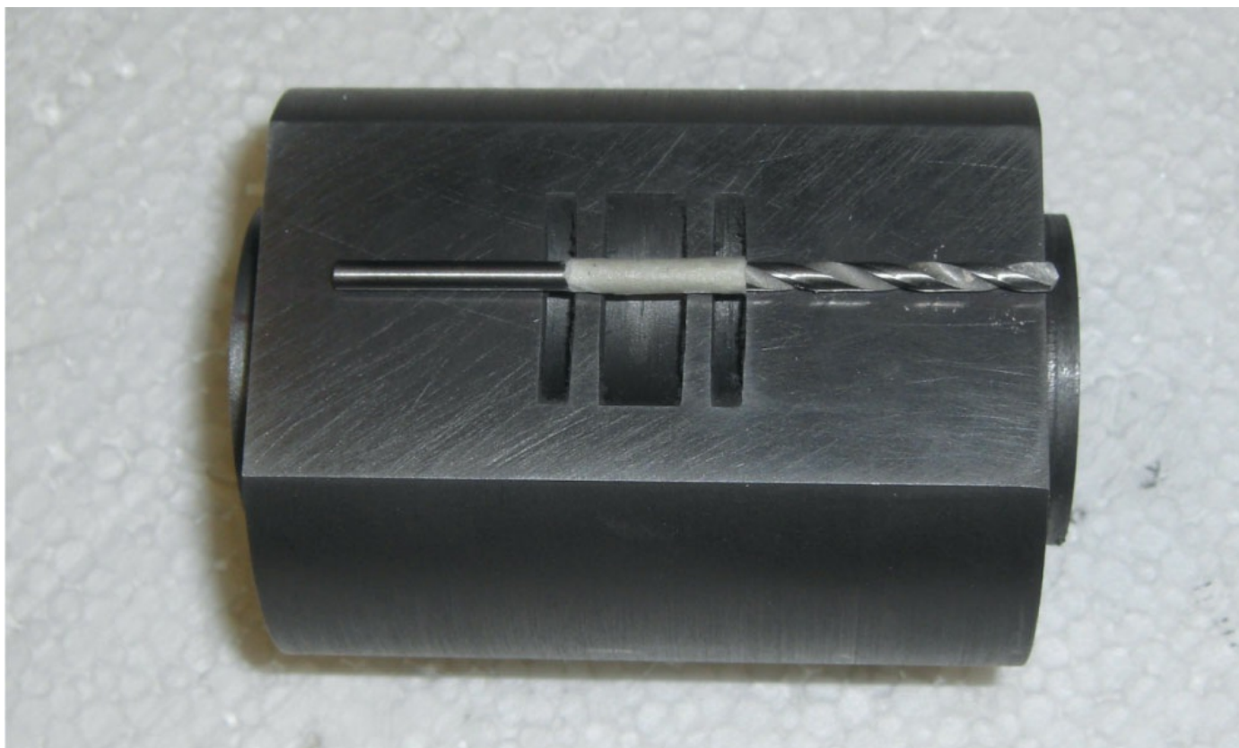
Checking drill length.
