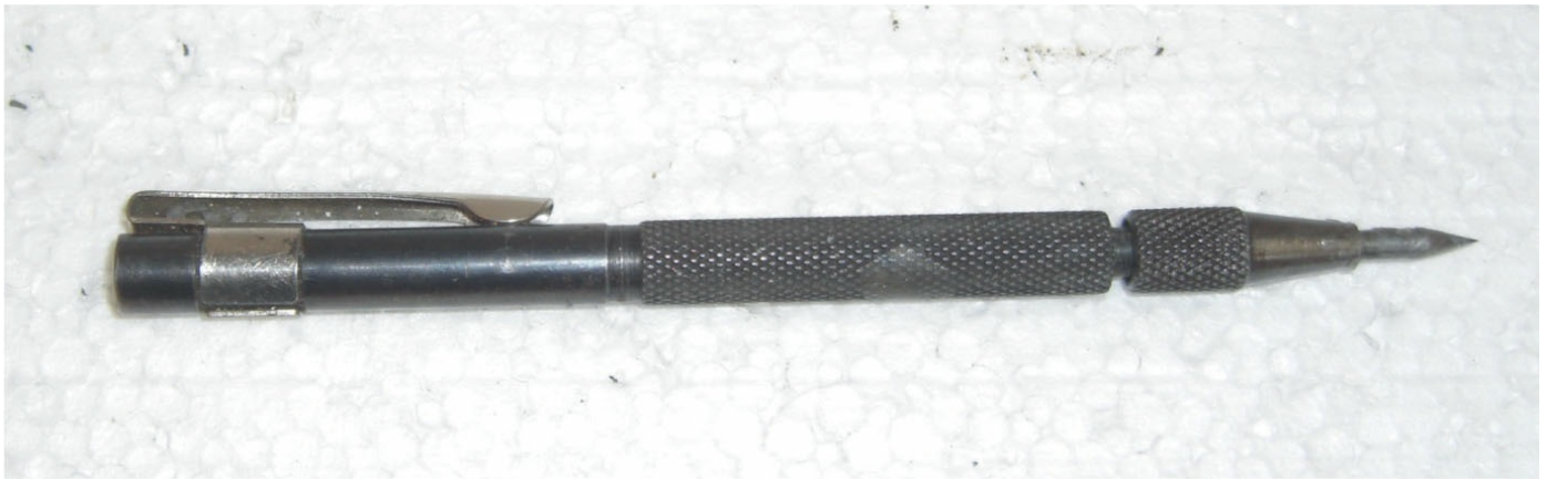
Scriber with replaceable tip.
