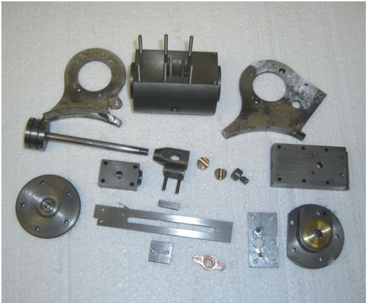
Cylinder components.
