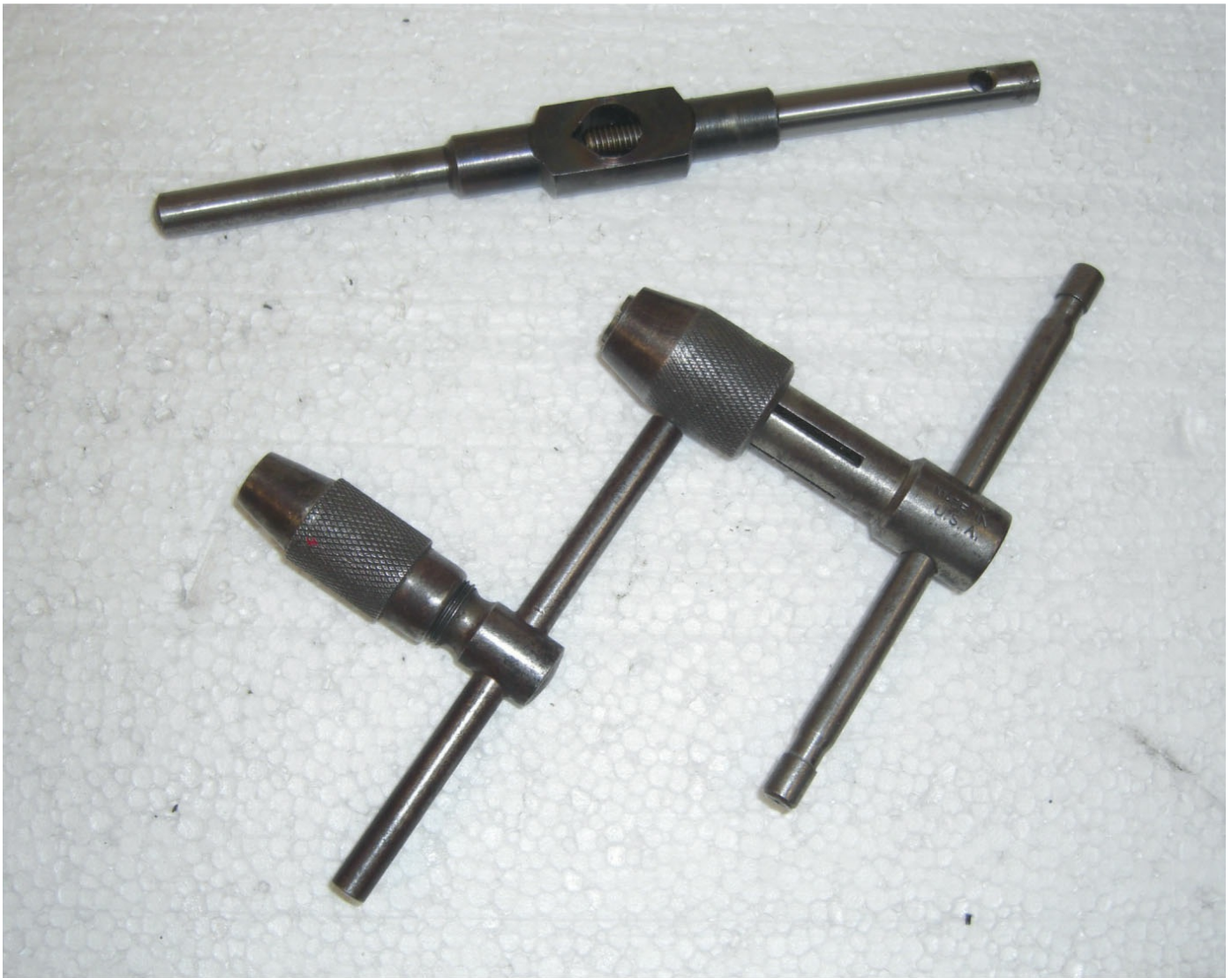
Straight and chuck-type tap wrench.
