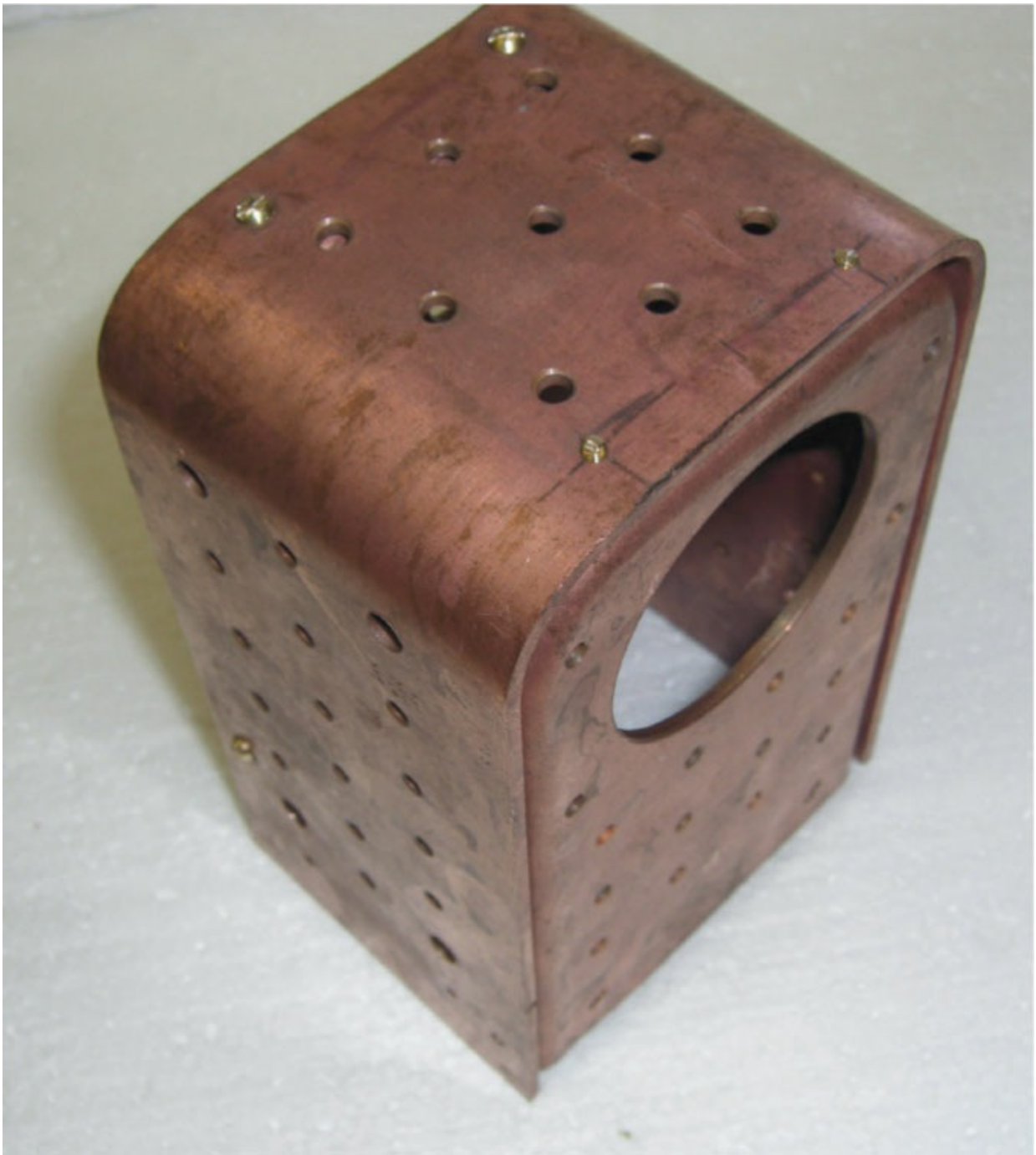
Firebox wrapper and door-plate.
