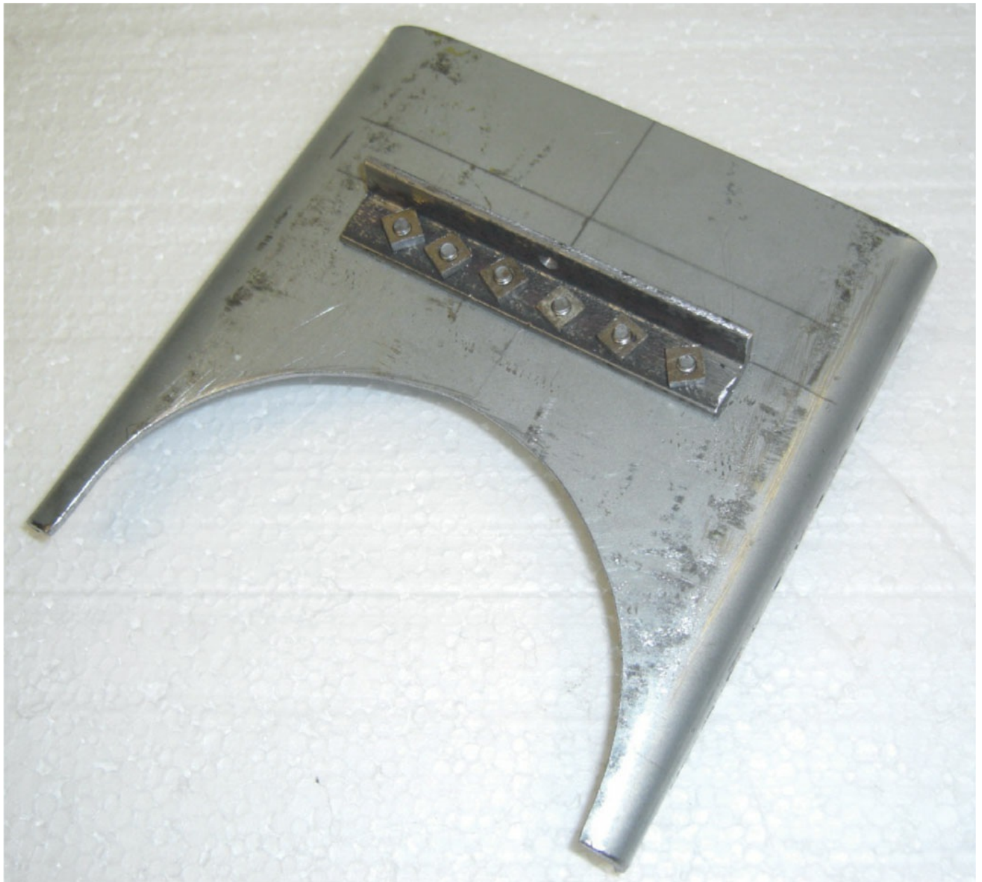
Rear axle support angle on throat plate.
