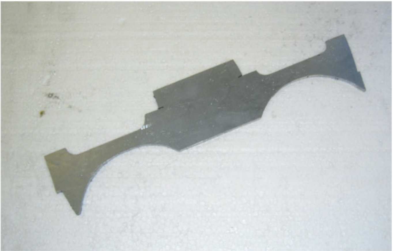
Development of sides of crankshaft bearing bracket.
