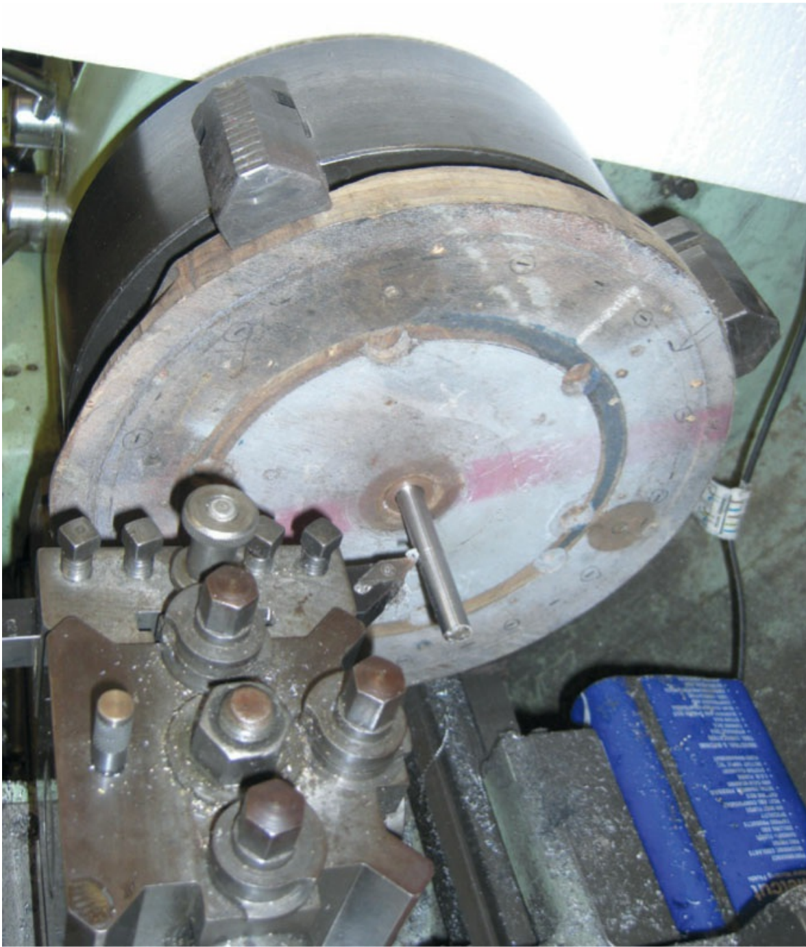
Truing dummy axle on assembly jig.
