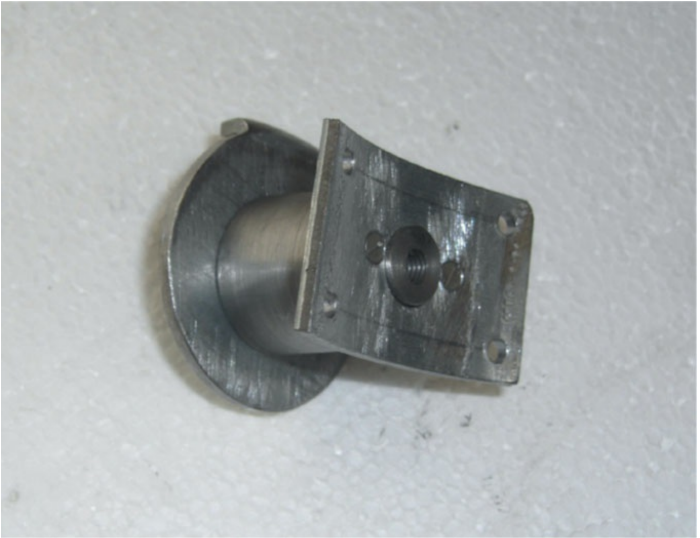
Perch bracket top plate.
