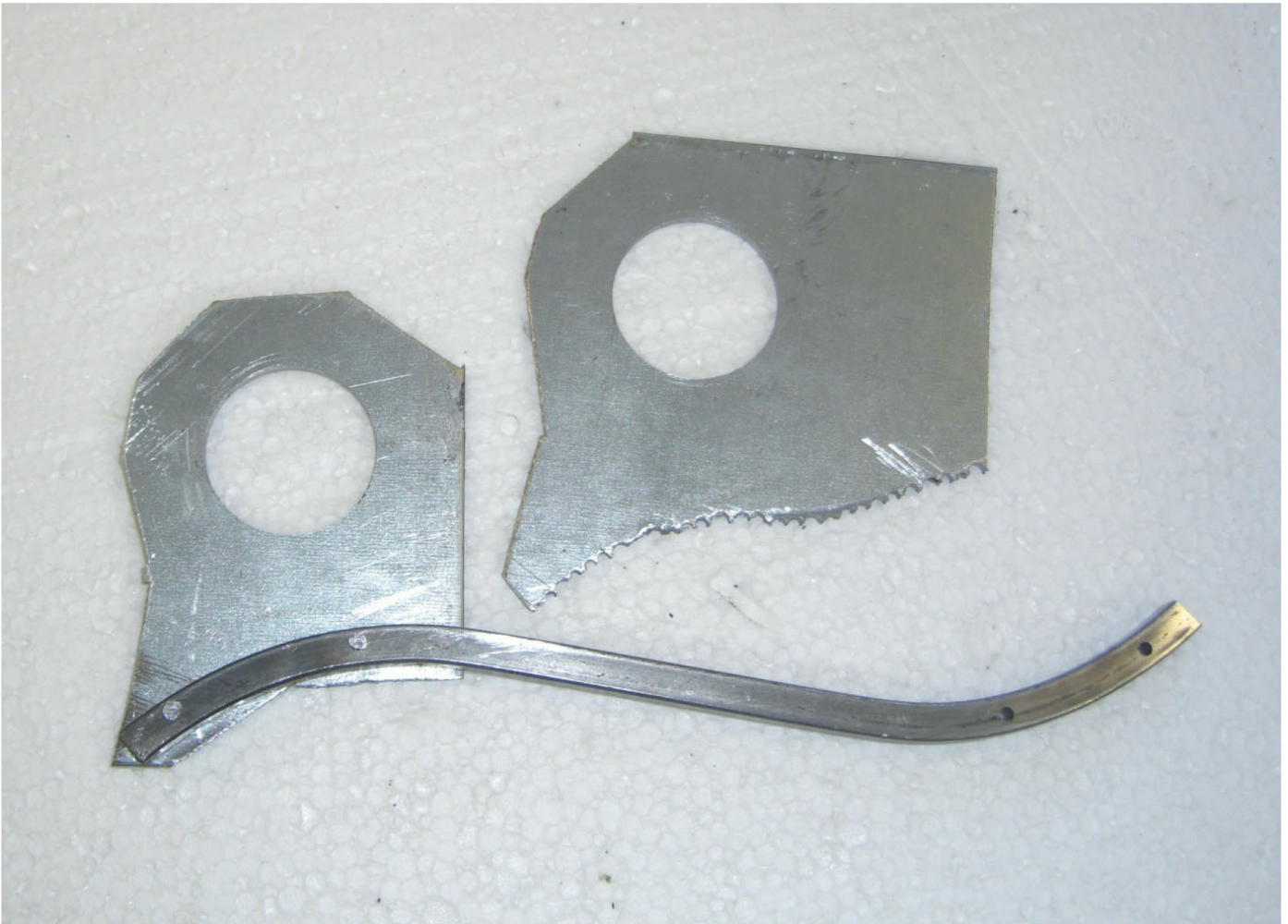
Cylinder mounting plates and flanges.
