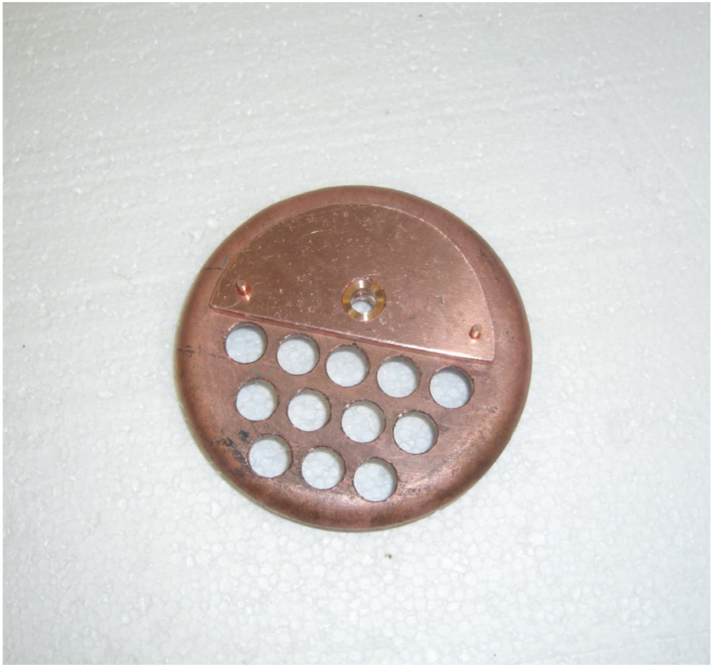
Reinforcing plate riveted on before silver soldering.
