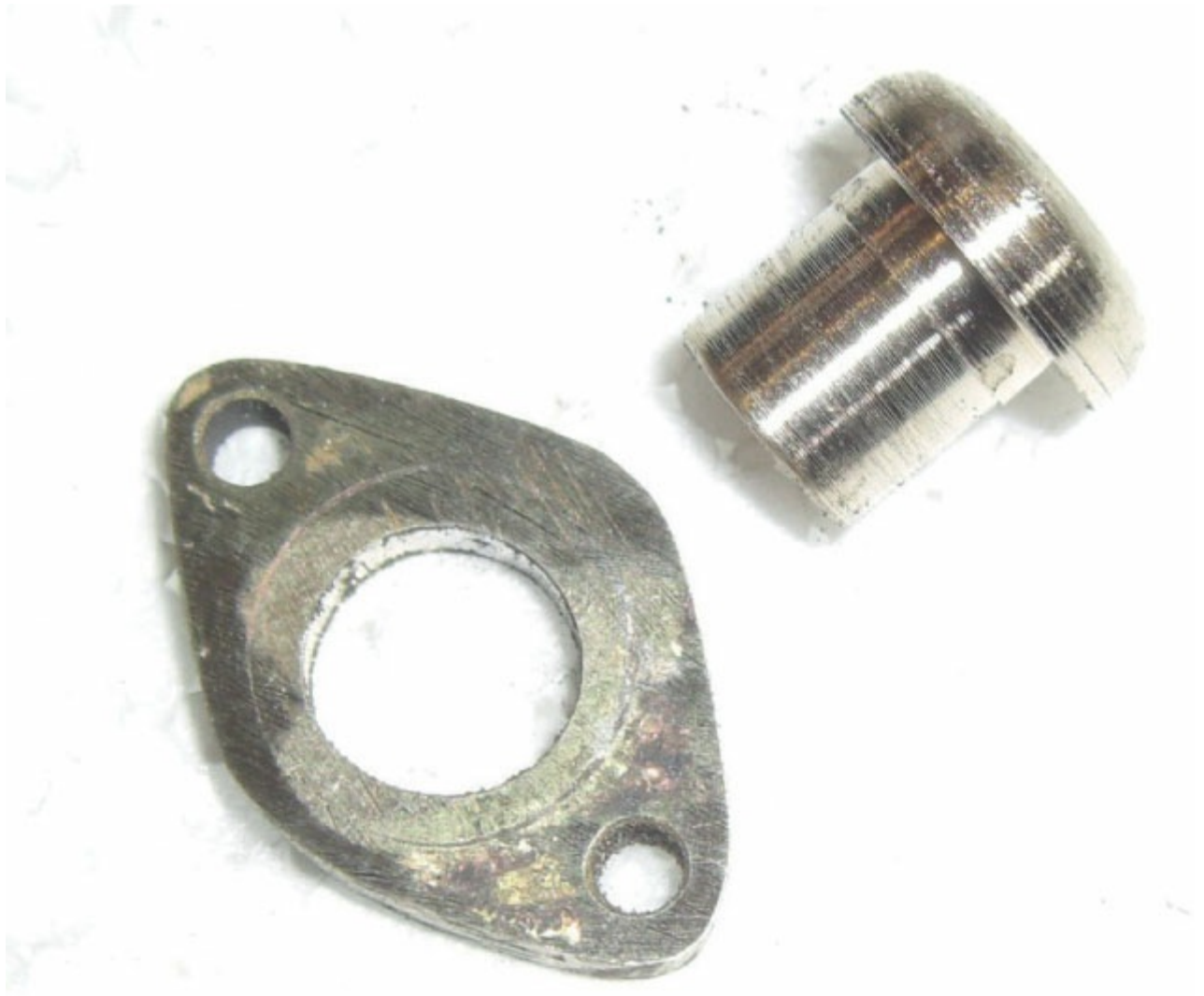
Pump gland components.
