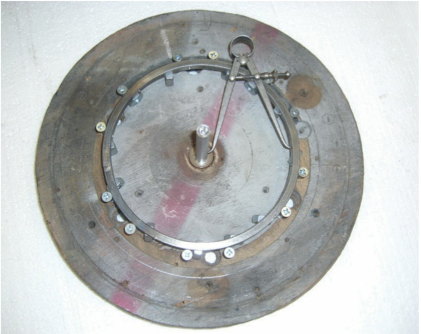
Checking rim is concentric to dummy axle.
