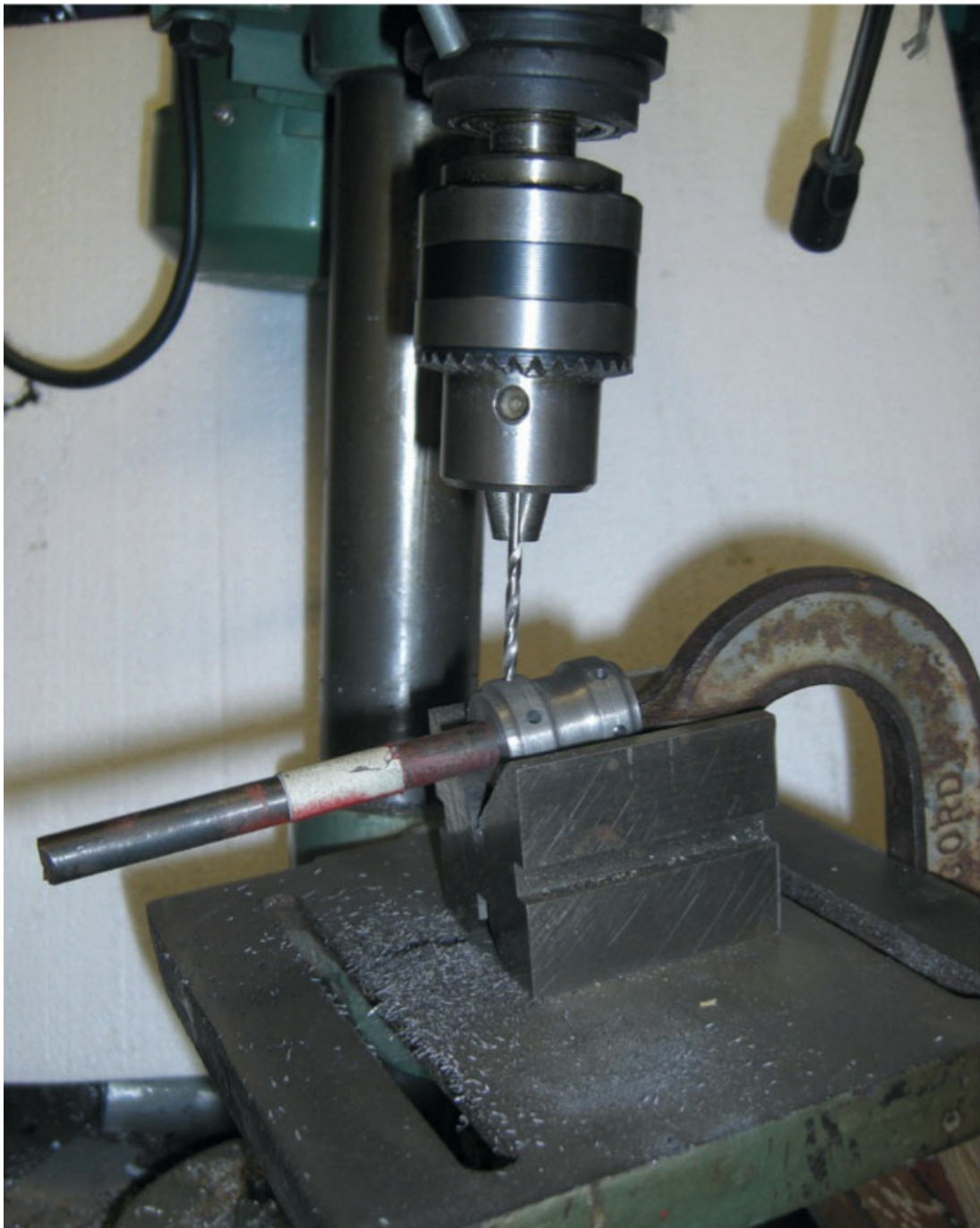
Drilling the spoke holes at an angle.
