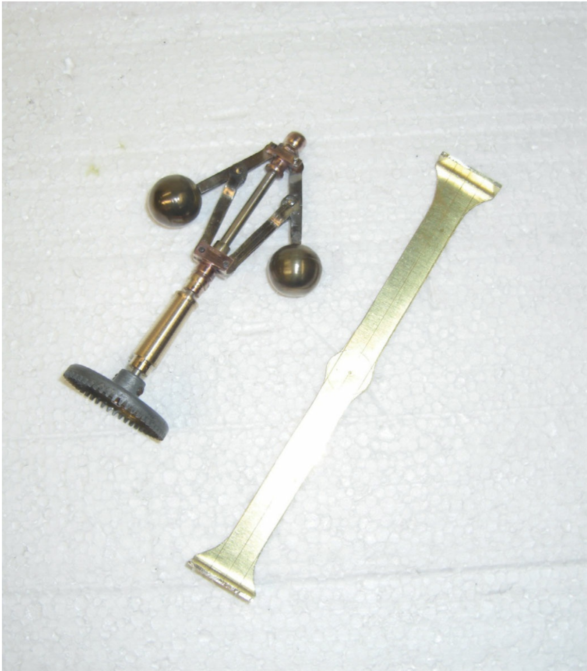
Governor, down, with bracket material.
