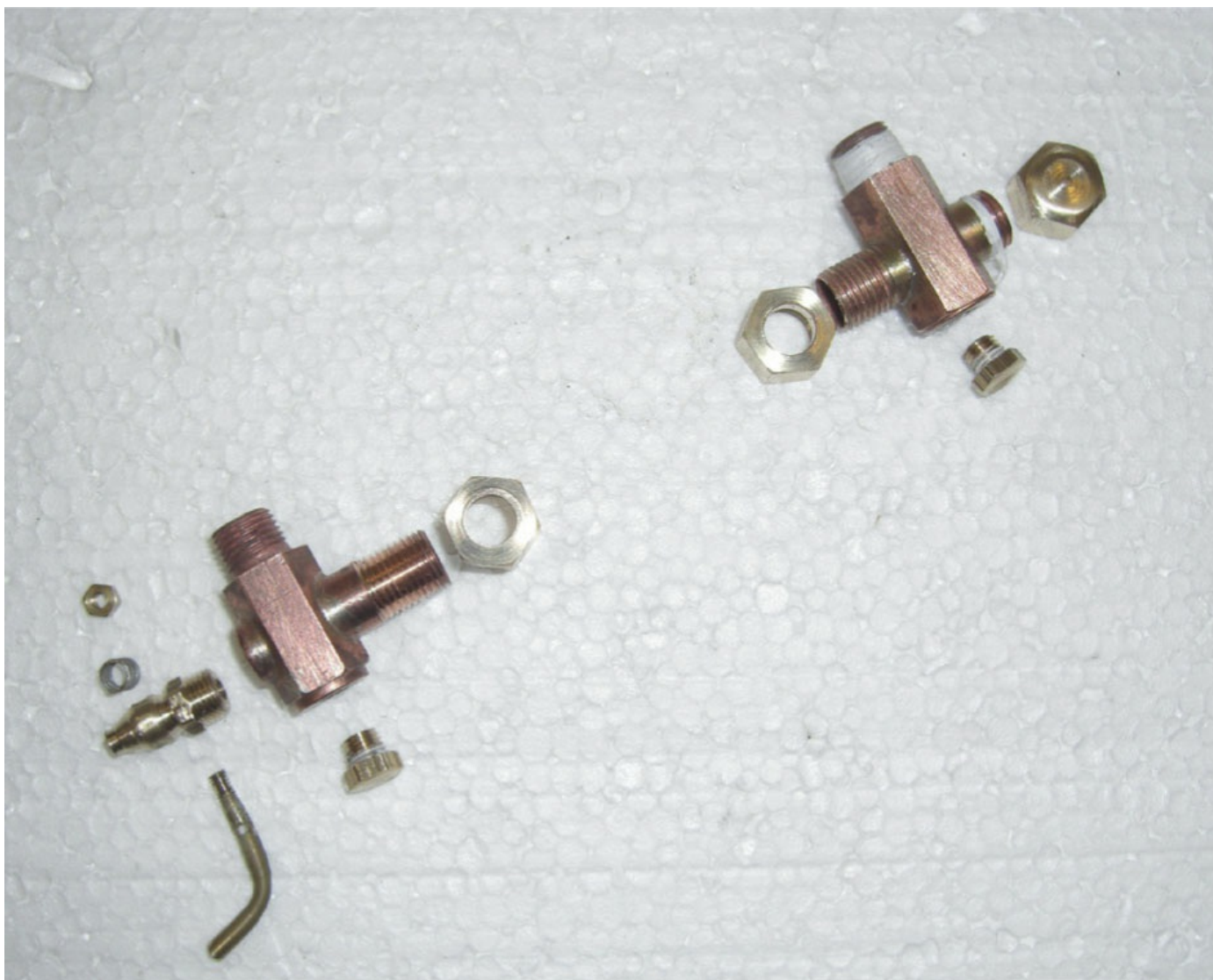
Water level gauge components.
