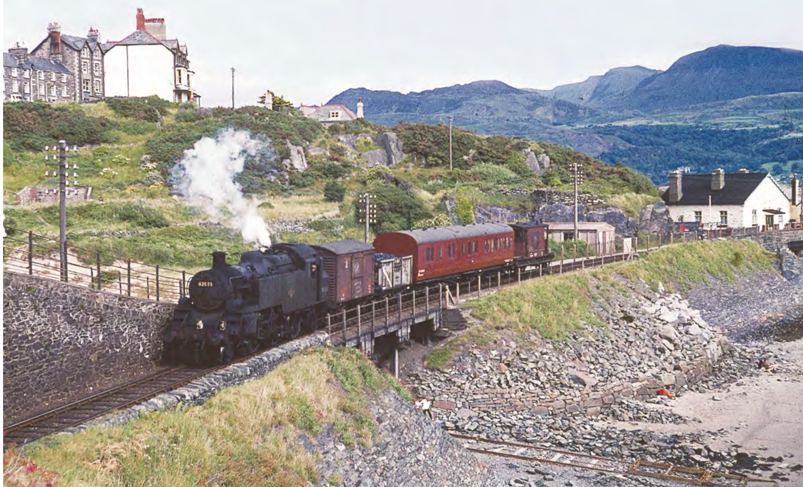
On 7 August 1963 BR Standard '3MT' 2-6-2T No 82033 runs off Barmouth bridge in charge of a northbound pick-up freight consisting of a single box van, a loaded 16 ton coal wagon, a departmental coach, and a brake van. The first two wagons are on the bridge that spans the lifeboat station ramp. The toll house for the public footpath across the bridge can just be seen on the right-hand side of the photograph, along with the associated tied cottage. The Cader Idris massif dominates the southern skyline. Tom Boustead
