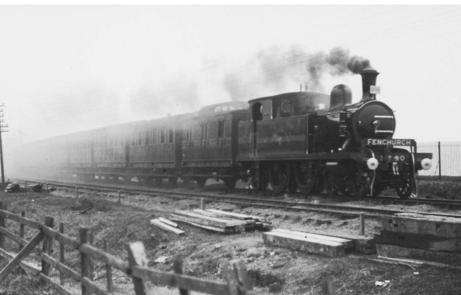
Despite the passage of ten more months, about 20 miles further west, in Westcliff-on-Sea, the 25kV electrification process is less advanced, with only masts in place on 26 June 1960 as Kentish Town-allocated Fairburn '4MT' 2-6-4T No 42237 steams alongside Leonard Road heading to Southend with an early morning seven-coach train. The electrification of public services of the LT&S lines was still two years away. Kentish Town's smart looking No 42237 contrasts with the usual appearance of unkempt Shoburyness-based 2-6-4Ts. R. Patterson/Colour-Rail.com/314441
