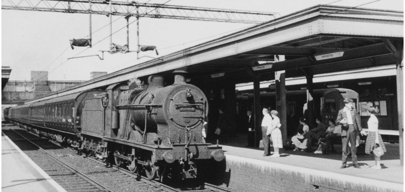
Electrification of the ex-LT&SR line through Upminster station is seen at an advanced, though still incomplete stage on 16 August 1959 as a Midland Division excursion to Southend passes through in the charge of Kentish Town shed's ex-Midland Railway ATC-fitted '3835' (LMS '4F') class 0-6-0 No 43964, coupled to an LMS-era Fowler straight-sided tender. In contrast, on the north side of the station is a London Transport District Line train of 'Q' stock at Platform 3 awaiting return to central London. No 43964 was a long-term resident of Kentish Town in British Railways days, until transferred across London to Cricklewood shed in June 1962. Bill Aves
