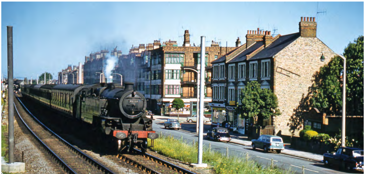
Despite the passage of ten more months, about 20 miles further west, in Westcliff-on-Sea, the 25kV electrification process is less advanced, with only masts in place on 26 June 1960 as Kentish Town-allocated Fairburn '4MT' 2-6-4T No 42237 steams alongside Leonard Road heading to Southend with an early morning seven-coach train. The electrification of public services of the LT&S lines was still two years away. Kentish Town's smart looking No 42237 contrasts with the usual appearance of unkempt Shoburyness-based 2-6-4Ts. R. Patterson/Colour-Rail.com/314441
