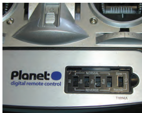
The Planet 5 DIL switches. I have removed the hinged window. The switches need a small screwdriver to operate them. The right hand switch is for the normal-slow selection for channel 5.
