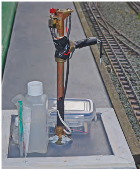
The smoke unit, switch and charging socket are mounted on a post which sits inside the building and are seen here along with the batteries in a plastic box and the bottle of smoke oil
