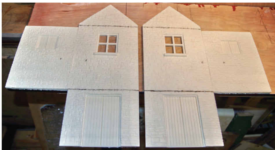
Marking out the cutting lines to make the sides of the Malthouse from the Modeltown parts
