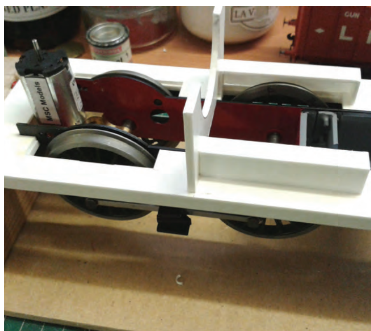
The footplate added in 3mm plastic, when attached to the brass angle it gives a very robust platform on which to build the body. Where you can't see the thickness, I've used 3mm plastic for a strong model.
