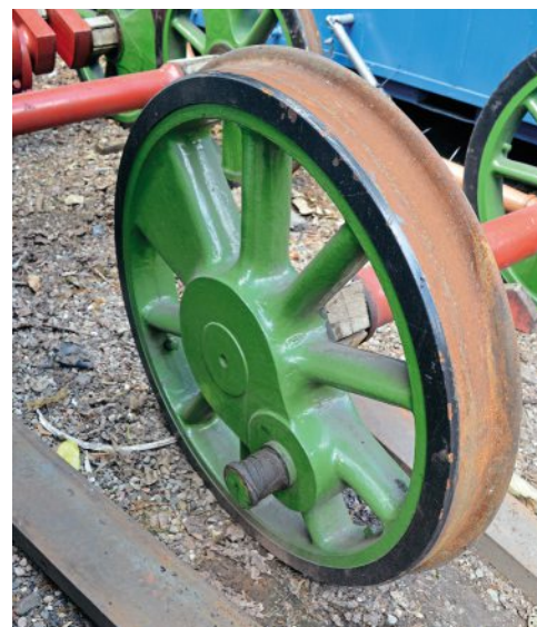
Most early Manning Wardle locomotives had cast-iron wheel centres with their familiar double-crank boss configuration, but these were superseded by a more conventional pattern during the first decade of the 20th century. Close examination of Warwickshire's wheel centres, particularly the balance weight configuration, still shows its descent from the earlier design, however.
