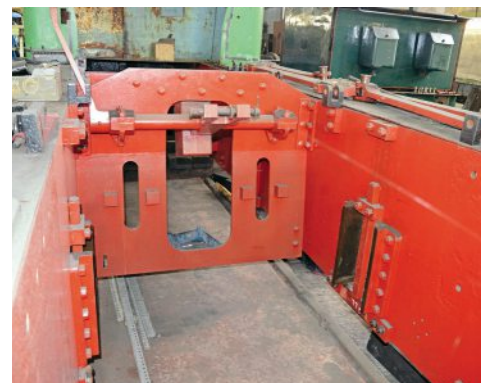
The area between the mainframes looking backwards from the rear of the cylinders to the motion stretcher. The weighshaft is fitted with a single 'Y'-ended bellcrank which raises or lowers the drop-links to produce the requisite forward/reverse and cut-off settings. Note the degree of protrusion of the stretcher above upper frame level, an indication of the raised boiler pitch necessitated by the position of the firebox.
