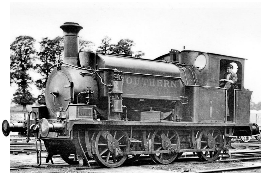
A future prize worth having! Later standard Q class celebrity SR W1 Medina (No. 1555 of 1902) could one day be recreated using, in part, the expertise (and cylinder patterns) currently being used to restore Warwickshire . This is the left-hand side of the engine, with the Westinghouse pump and foreshortened tank handrail visible.
