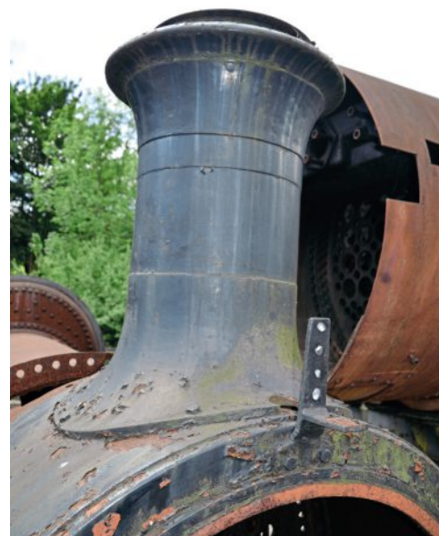
By the early 20th century, the cast-iron chimney had superseded earlier fabricated items as standard for most Manning Wardle products, and Warwickshire's chimney conformed to this trend. Currently deemed repairable, it is still mounted on the life-expired smokebox in Bridgnorth yard. A copper band was riveted on to the lower part of the chimney cap but this is currently painted black.
