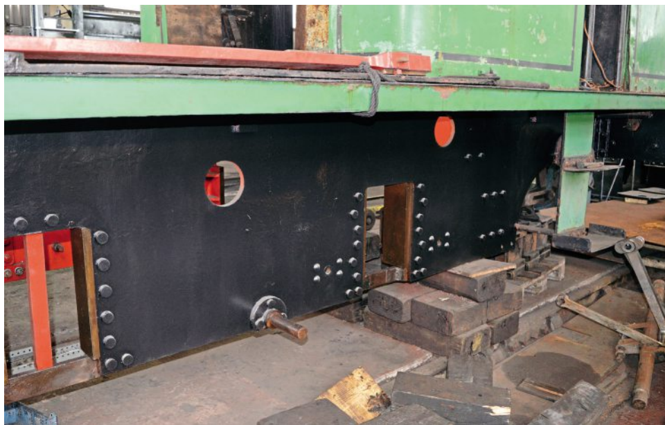
The rear left-hand mainframe area, emphasising the closeness of the spacing of the intermediate and rear axles on Warwickshire when compared with the standard Q class. The rear brake hanger pivot is also shown. In this Manning Wardle design the brake hangers were inverted and their pivots located near to the bottom of the mainframes, a configuration also found on Dolobran (No. 1762 of 1910) and its sisters.
