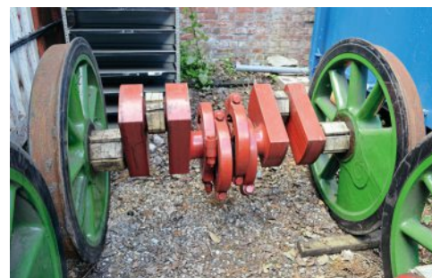
The driving wheelset with crankshaft and eccentrics, in the yard at Bridgnorth, with the newly overhauled crank and axle journals being protected from corrosion by the obligatory grease, cloths and wooden cladding.
