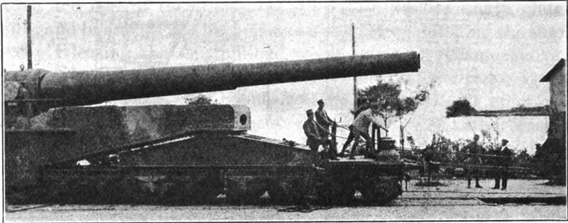
TRANSLATING MOUNT WITH HAND WINCH AND CABLE.
