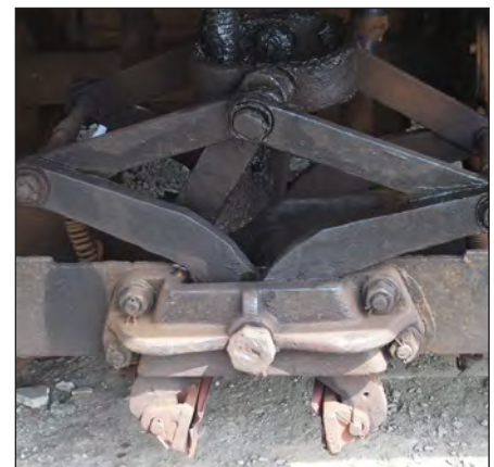
The 1895-fitted Fell brake saved the tram after its electric braking system failed.
