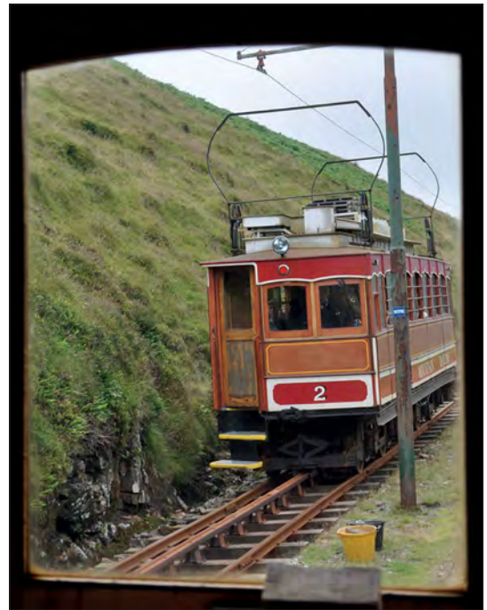
Above: Tram 2 was pictured by Phil Parker on 25th July, 10 days before it suffered brake failure. The Fell Rail can be seen in the centre of the track.
