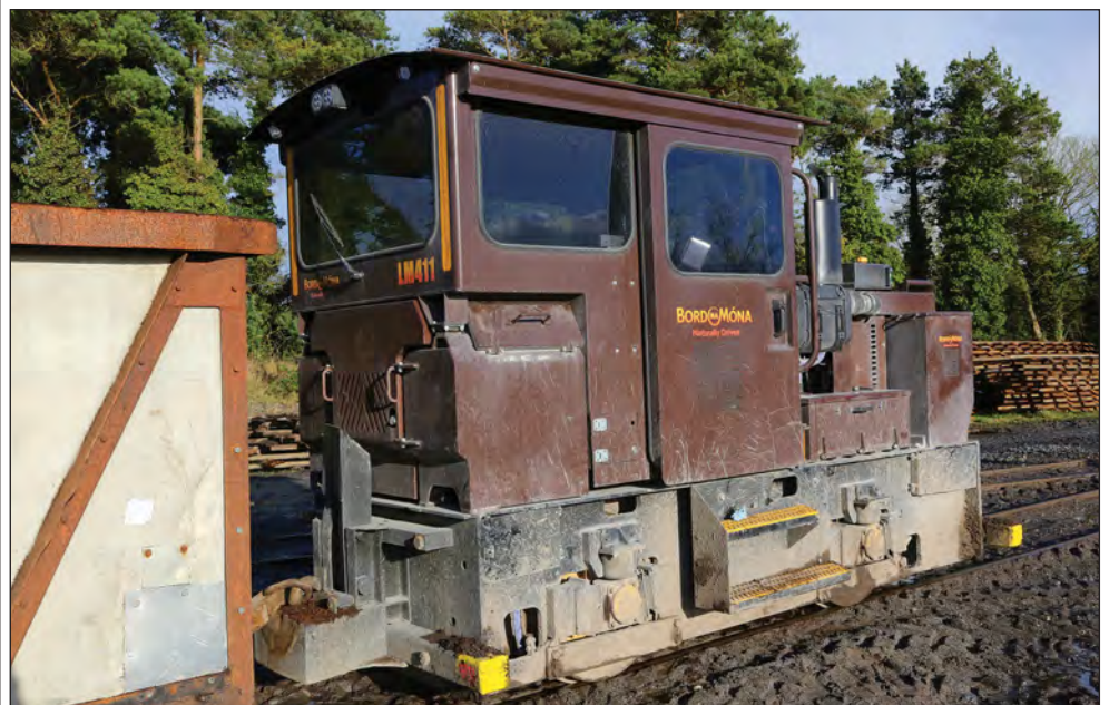
Below: LM411 awaits the start of the second shift at West Offaly in March 2017. Note the massive sandboxes, tinted windows and the buffing gear to allow automatic tipping of the loaded wagons.
