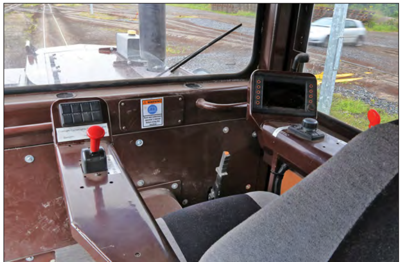
Right: Inside LM425. On the left armrest are touch controls for the LED lights and the red brake lever. The handbrake is on the floor, just visible at right is the red throttle.
