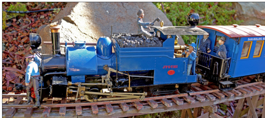
This Roundhouse engineering Darjeeling Class B 0-4-0T pulled 100% of its own weight up the grade.
