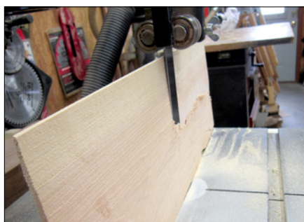
1. A bandsaw with a resaw blade is used to remove some of the thickness from a piece of full-size cedar siding.
