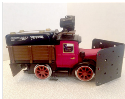
6. Railtruck with battery installed. The weight of the battery provides extra traction.
