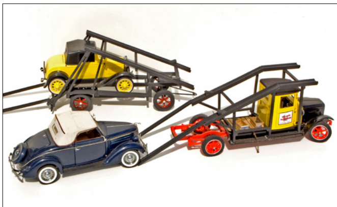
7. To load and unload this type of transporter, the trailer must be disconnected and the autos are driven on or off by means of a ramp. This was a lot more work than on modern hydraulic transporters.
