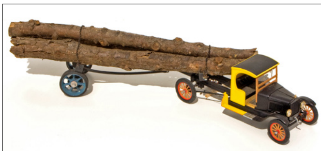
4. This type of logging truck used a dolly and a drawbar. The log bunk on the truck end of the log pivots to allow the truck to turn.
