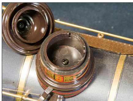
9. Manufacturers make extensive use of press-fit details to hide screws that attach other details. In this case, the lid of the sand dome comes off to allow access to the screw that holds the dome to the boiler.
