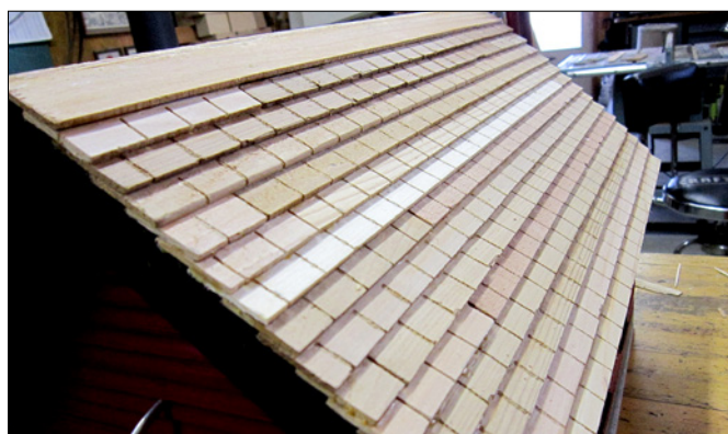
12. Blank strips, 1/2" wide, are used for the roof cap.
