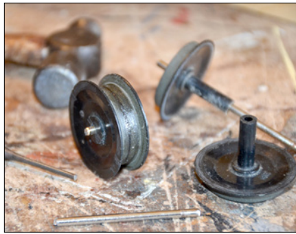
2. Pulleys made from plastic wheels—see figure 1.
