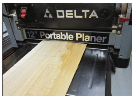
2. The board is put through a planer to ensure uniform thickness.
