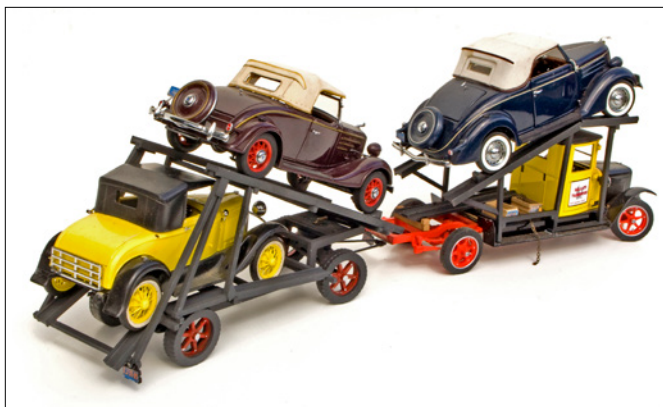
6. Three automobiles can be transported on this type of carrier—one over the cab and two on the trailer.
