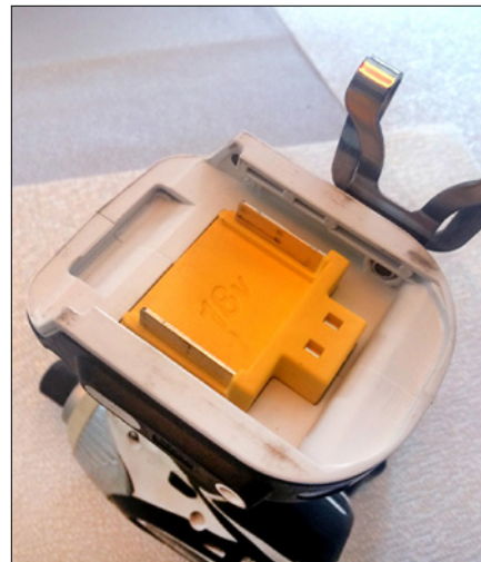
4. This shoe, seen here on the bottom of the drill, provides the connection to the battery.
