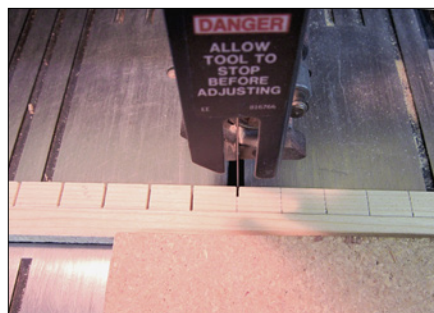
6. Shingles are then individually cut on the bandsaw.
