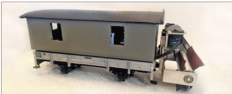
13. With the body in place, access to the battery is limited, which is why the control switch was located outside.
