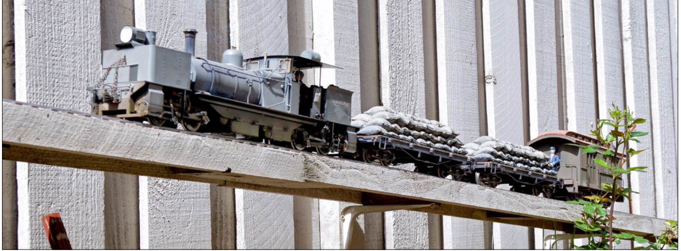
On the 8% grade, the Roundhouse Darjeeling Garratt 0-4-0+0-4-0 was able to lift a train weighing 94% of its own weight.
