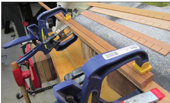
9. The strip is clamped in place over the starter strip.
