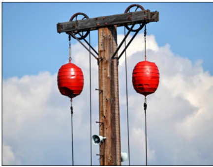
1. The full size, double-ball signal at the Conway Scenic Railroad in New Hampshire.
