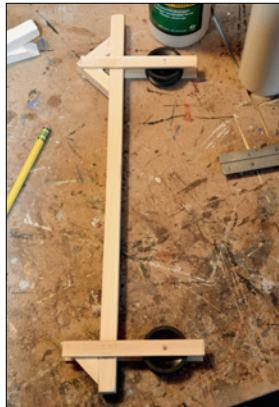
4. The finished mast, with pulleys and additional bracing for the arms.
