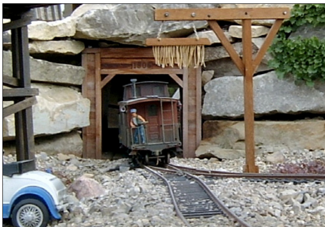
3. This telltale on the author's railroad alerts brakemen on top of railcars of an approaching low overhead clearance.
