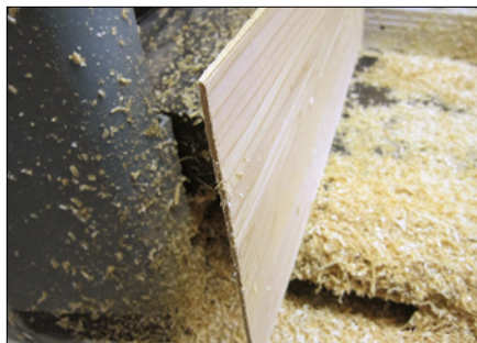
3. A thickness of \frac{3}{32} " is used for the author's miniature shingles.
