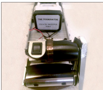
12. The on-off rocker switch located near the sweeper's motor. The switch turns on the rotating sweeper.
