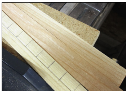
5. Each strip is longitudinally divided by a line at the \frac{1}{2} " mark, then individual shingles are marked off at \frac{3}{4} " spacing.
