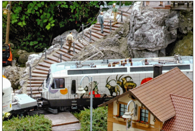
5. Marcus and Vanessa Kollmann's Landschaft Gartenbahn models the elegance of European rail travel. Tile has been glued (exterior glue or thinset mortar) and stacked on a bed of mortar that extends to surrounding boulders. Note the impressive railing posts. Marcus Kollmann
