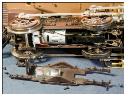
10. The wheels are held into the frame of the Bachmann Mogul by a retaining plate that attaches to the bottom of the chassis. If you remove this, the wheels will drop out.
