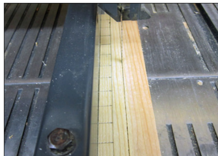
4. The \frac{3}{32} " board is cut into 1"-wide strips on the bandsaw.
