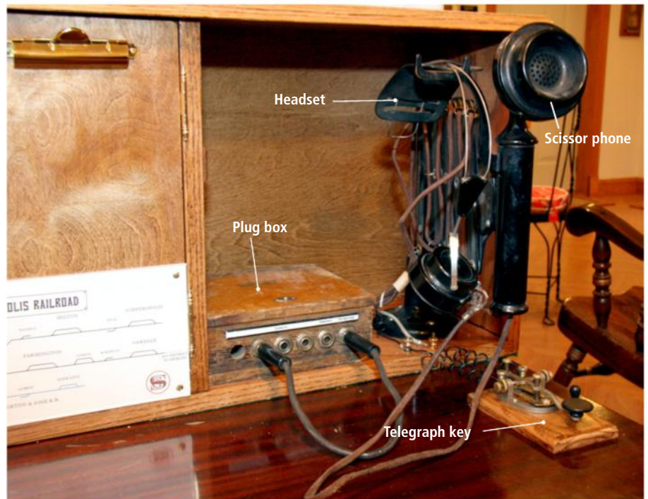
5 Lines of communication. The scissors phone mounts to the bottom of the console. Don attached felt to the bottom of the phone to prevent scratching the desk top. The small box to the left of the phone is a plug box to select whether the dispatcher will use the scissor phone and headset or a breastplate microphone with headset.
