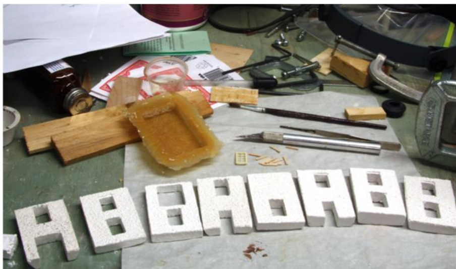
5 The eight wall castings in order. Each wall shows the combination of doors and windows needed for that particular wall. Raymond made 15 castings from the mold, seen above the walls, before he produced the eight needed sides.
