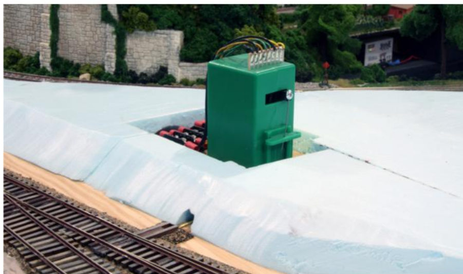
❶ Tortoise needs a shell. Raymond installed a Tortoise by Circuitron switch motor on the surface of his layout to clear a track that runs beneath. The blacksmith shop will conceal it from view.
