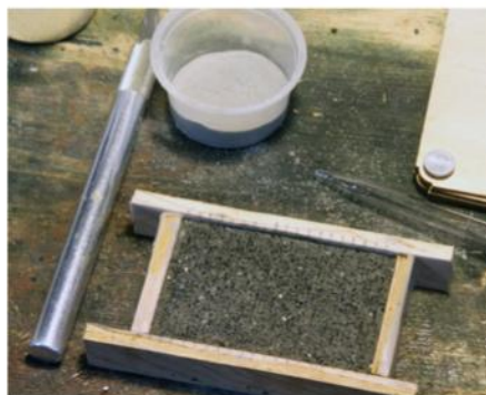
❸ Making a master. Raymond built his master on a piece of plywood. He glued individual pebbles to the wood with white glue, then added rock dust and secured it with thinned glue after wetting the surface with alcohol.
