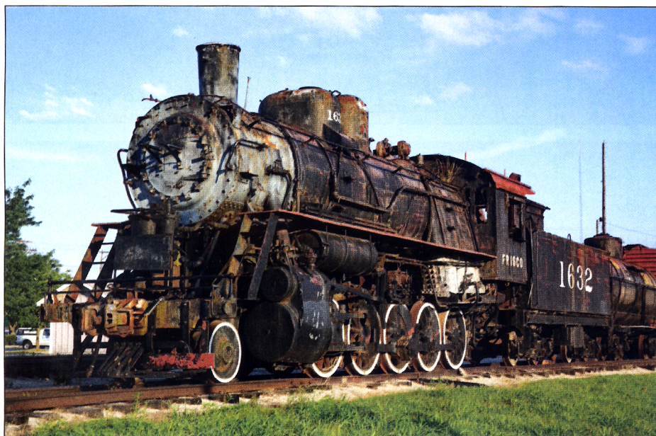
ABOVE: SLSF No. 1632 is at Belton, Mo., on July 30, 2016, on the Belton, Grandview & Kansas City Railroad. The shield over the compressor was added by Eagle-Picher, and protected the pump from flying ore debris when the locomotive was switching cars. JEFF TERRY PHOTO
