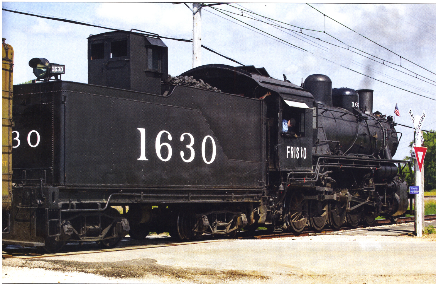
ABOVE: Illinois Railway Museum's 2-10-0 No. 1630 is backing up toward Union after making a passenger run to Kishwaukee Grove on July 3, 2016. It took a tremendous amount of work to return the tender to its 1940s appearance; this involved rebuilding the coal bunker after it had been cut down by Eagle-Picher. The doghouse is a faithful replica of the type used on SLSF steam locomotives. JEFF TERRY PHOTO
