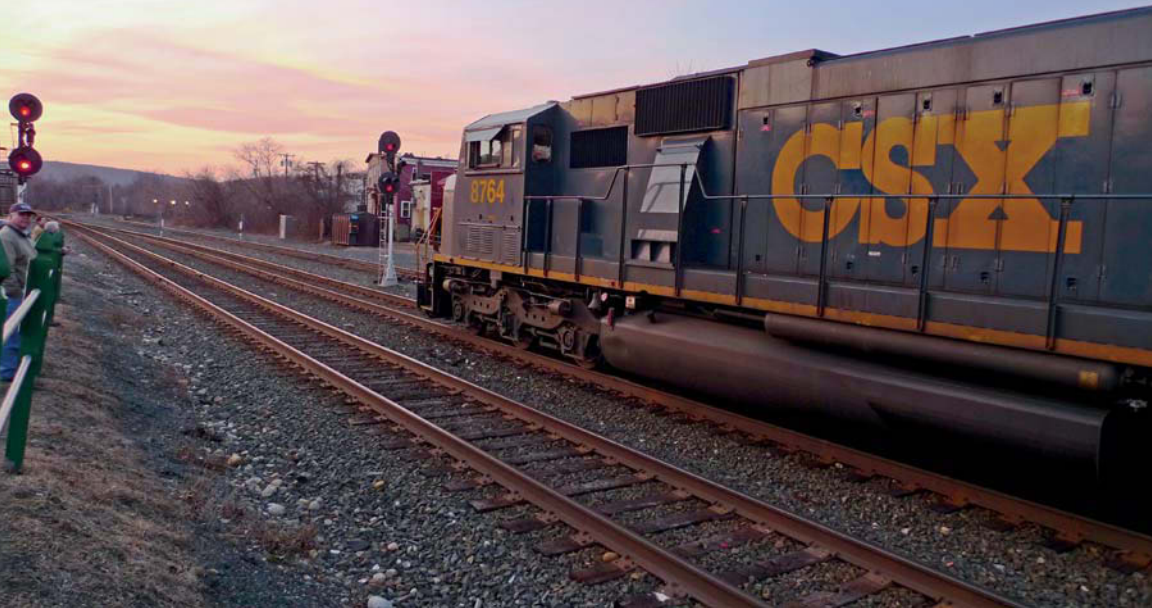
A CSXT SD60M at Palmer, Massachusetts: this westward freight holds for a red signal at the end of the controlled siding at CP83 (dispatcher controlled point 83 miles from South Station, Boston) waiting for an eastbound train. Brian Solomon
