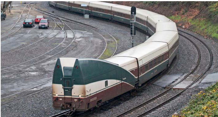
Amtrak's Cascades tilting TALGO trains feature large fiberglass fins designed to allow a visual transition between EMD F59PHI diesels and these unusually low profile cars. Scott Lothes
