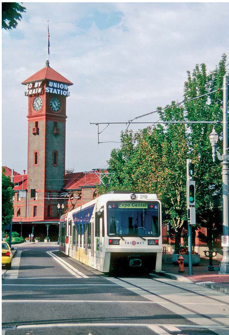
Portland's MAX light-rail network began operations in 1986. In 1998 and 2004, it bought fleets of Siemens SD660 light-rail cars (201 to 252 and 301 to 327), such as this one seen at Portland Union Station. Jack May
