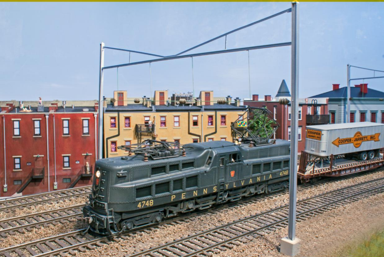
9 A PRR P5a electric pulls a Truc-Train of piggyback flatcars past the town of New Brunswick. The locomotive and cars are three-rail O gauge models converted to run on two-rail O scale track.
