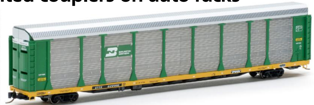
Jim converted this Micro-Trains auto rack to body-mounted couplers. It and its companions run just fine on his 18" minimum-radius mainline curves. Bill Zuback photos
