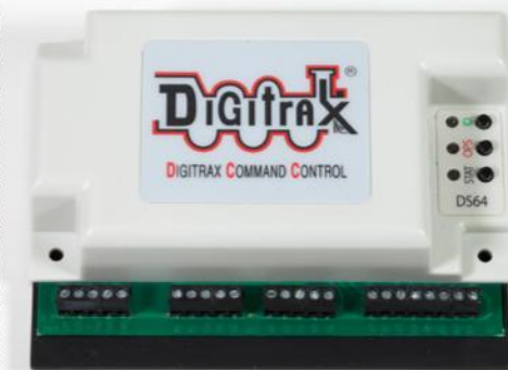
4 Route machine. The Digitrax DS64 comes in a plastic enclosure with screw terminals for easy hookup to switch machines, accessories, or pushbutton inputs. It can be programmed to align turnout routes for up to four turnouts. Several can be connected together if they're attached to a Digitrax LocoNet.
