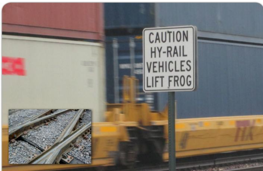
Above: This sign in Santa Fe Springs, Calif., warns drivers of high-rail vehicles that a frog is coming up that requires special care to cross. Jay Michalsky photo Inset: A lift frog, or flange-bearing frog, lifts wheels on the diverging route over the flangeway of the main to give that route a smoother ride. The small wheels of high-rail vehicles could have trouble crossing the gap. J. David Ingles photo
