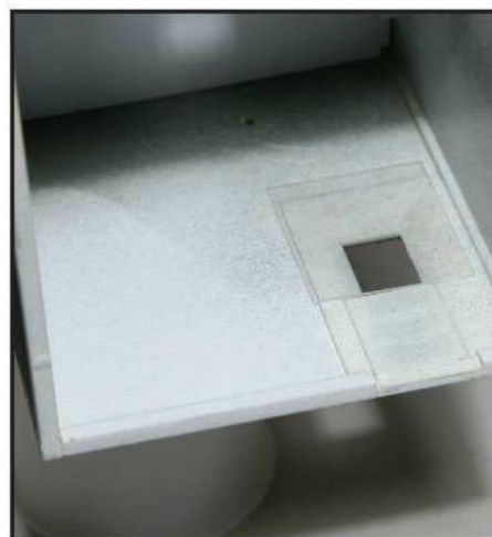
26 Here's an interior view of the door shown in fig. 24, with clear sheet styrene window glazing.
