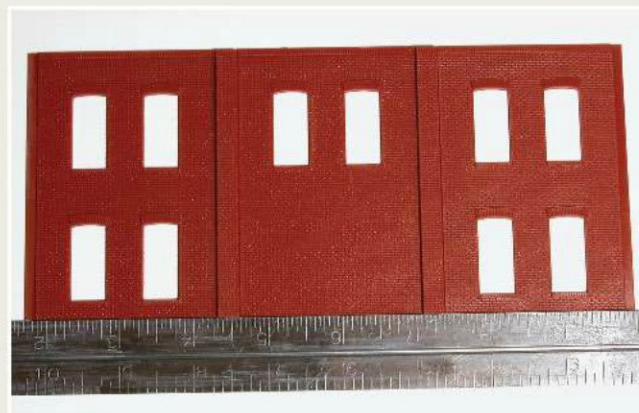
A steel straightedge works well for keeping wall sections aligned while gluing them together.
