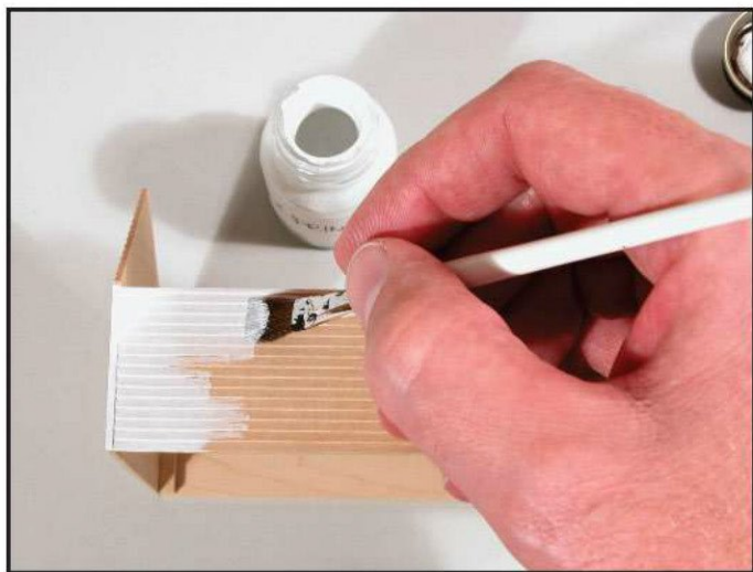
23 Primer goes on well with a brush. Make sure all areas of the structure are covered.
