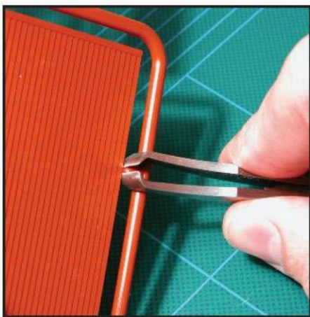
5 Sprue cutters do an excellent job of neatly separating parts from their sprues. If this is done properly, little cleaning up is necessary.
