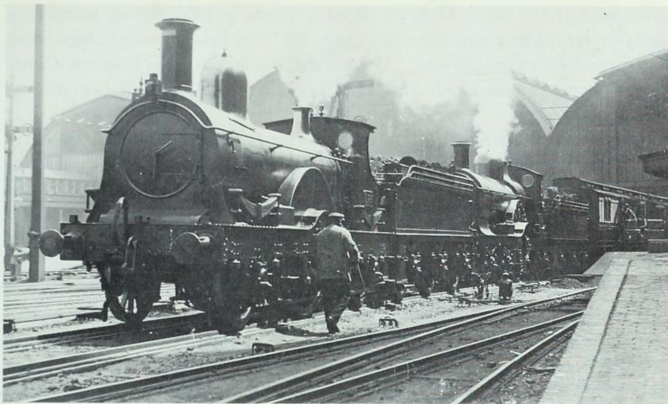
The Flying Dutchman too heavy for one engine. One of the Dean 7 ft 8 in 4-2-2s piloted by a 2-2-2 No. 1124 at Paddington.
