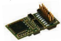
Decoder with 16-pole plug; can be updated; multiprotocol operation possible; motor control; braking tracks supported; locomotive addresses programmable; NMRA-compatible; comfortable change of operating parameters possible: i.e. the locomotive does not have to be opened; overcurrent protection; RailCom \*\*
