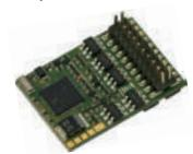
Decoder with 22-pole plug; can be updated; multiprotocol operation possible; motor control; braking tracks supported; locomotive addresses programmable; NMRA-compatible; comfortable change of operating parameters possible: i.e. the locomotive does not have to be opened; overcurrent protection; RailCom \*\*
