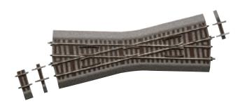
Crossing K15, length 230mm, crossing angle 15 deg.; the frogs can be polarized with a 10019 relay, crossing can be integrated in a track protection arrangement like a normal magnetic item. The crossing railway tracks are not electrically separated. For the installation of diagonals, two off D4 and one off D12 are enclosed. With bedding.
