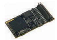
Sound decoder with 22-pole plug; can be updated; multiprotocol operation possible; motor control; braking tracks supported; locomotive addresses programmable; NMRA-compatible; comfortable change of operating parameters possible: i.e. the locomotive does not have to be opened; overcurrent protection; RailCom \*\*
