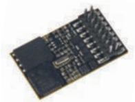
Sound decoder with 16-pole plug; can be updated; multiprotocol operation possible; motor control; braking tracks supported; locomotive addresses programmable; NMRA-compatible; comfortable change of operating parameters possible: i.e. the locomotive does not have to be opened; overcurrent protection; RailCom \*\*
