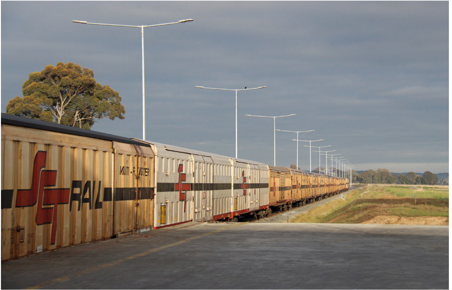
Unlike other Australian intermodal rail operators the backbone of SCT’s rail activity is not container movement but its fleet of vans, which are used to convey palletised freight between its terminals. The vans’ large doorway area facilitates easy access to load or unload the vans with a fork lift. In this Monday, 19 June view a line of the company’s vans occupy the main siding leading in to the cross-docking shed at the Barnawartha terminal.
