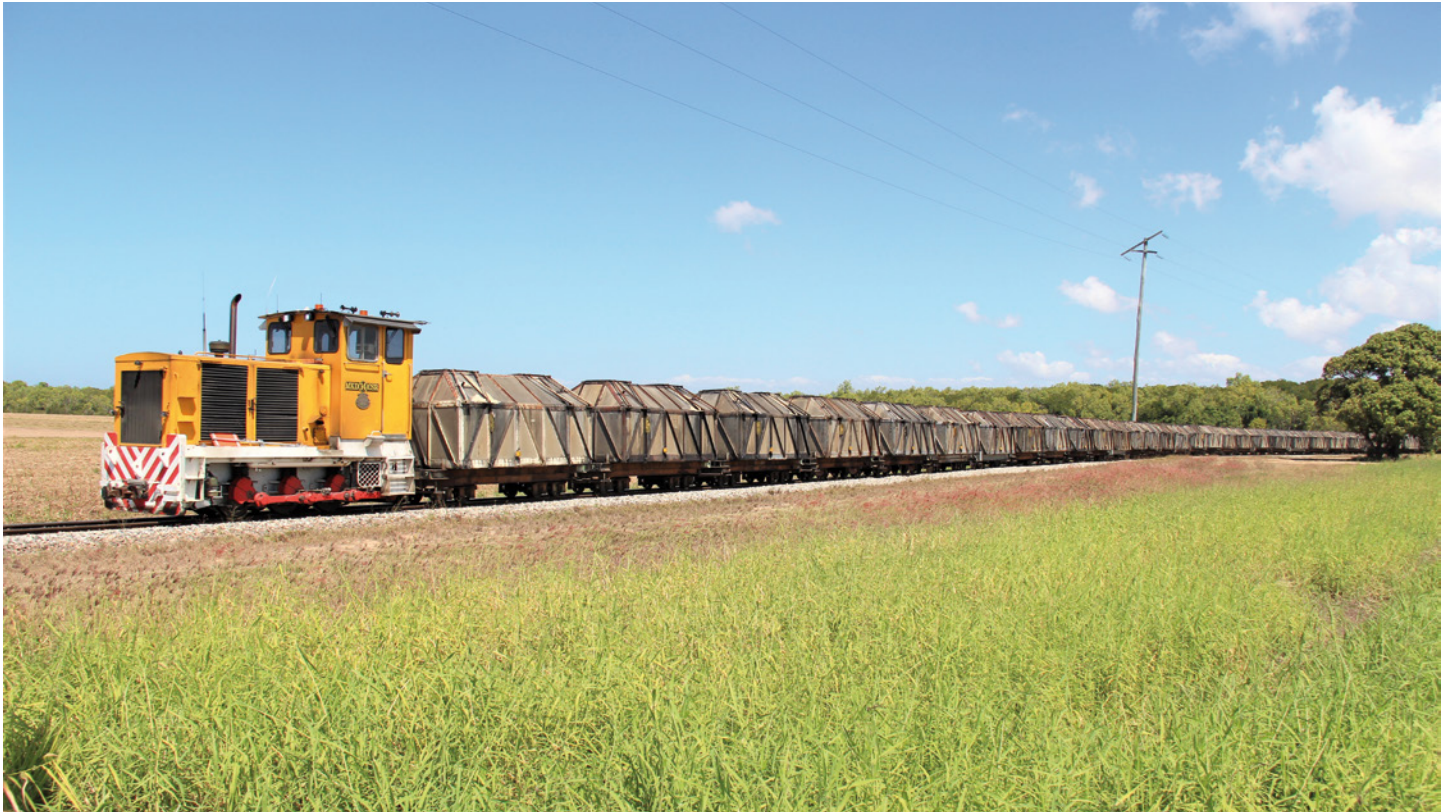
In contrast to other North Queensland sugar mills that use Queensland Rail's network or road transport, Wilmar's Victoria and Macknade sugar mills, near Ingham, export their raw sugar through the port of Lucinda using a line from their 610 mm gauge system that links the two mills. In this Sunday, 27 August view 1968-vintage EM Baldwin 0-6-0DH unit No.14 hauls a load of bogie wagons loaded with sugar near Gentle Annie Creek, not far from Lucinda. John Hoyle
