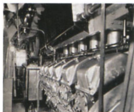
Looking along the Zephyr's 1800-horsepower Diesel engine toward the broad-windowed engineer's cab.
