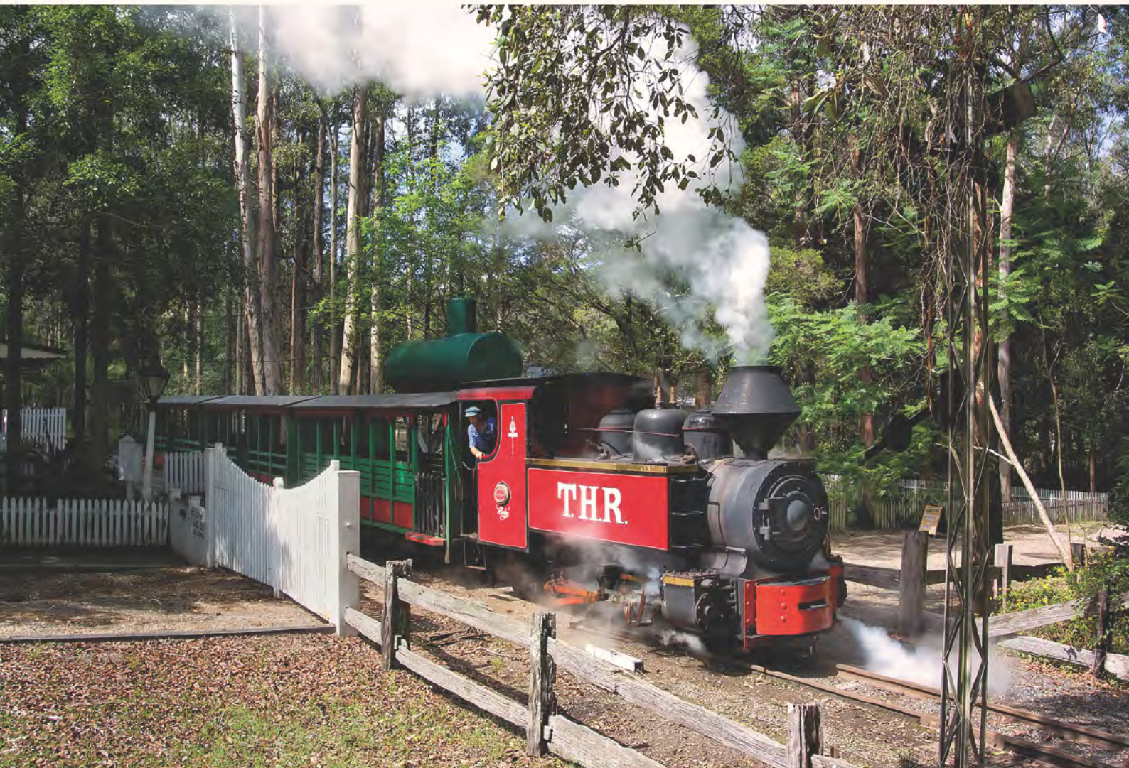
Former South Johnstone Mill John Fowler 0-4-2T tank locomotive No.10 (built 1928, builder's number 17881) departs "Timbertown Station" at Wauchope, NSW, at 2pm with the final of four public shuttles of the day, Sunday 26 March. This locomotive operates four, hourly trips (11am, 12pm, 1pm and 2pm) most days on the heritage park's two-kilometre, 610mm-gauge circuit track, taking passengers on an 8-10 minute, anti-clockwise run around the 39-hectare site. Chris Walters
