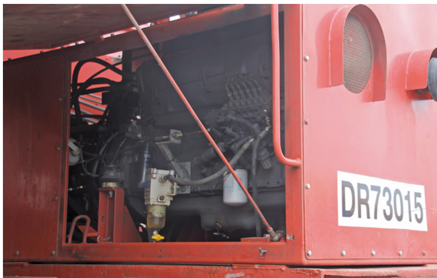
Left: The Deutz 353 kilowatt engine on wagon DR 73015 (Sammps 99 81 9353 037-0 A-RTS) under the conveyer belt of an adjacent wagon at East Greta Junction in Maitland on Wednesday 14 December 2016.
