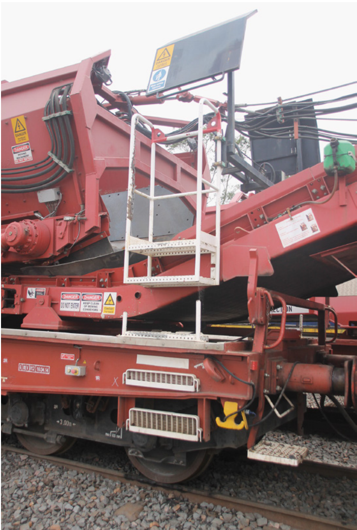
Right and Below: The conveyer system between two Sammps wagons. The operator stands on the frame and is strapped to the top of the ladder assembly to avoid falling. As the condition of the ballast is unknown until it is dug out the spoil has to be continually monitored while the ballast is being moved to prevent clogging or overloading of the conveyer belt. When a wagon is at the head of a wagon set the conveyer belt unit can be swung up to 45 degrees either side of the wagon for unloading onto the ground or other wagons. Photographed at East Greta Junction on Wednesday 14 December 2016.
