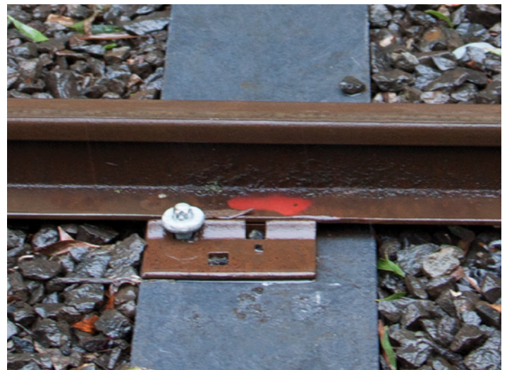
An AJAX M19 double thread Dog Screw in use on a test sleeper. Adrian Ponton
