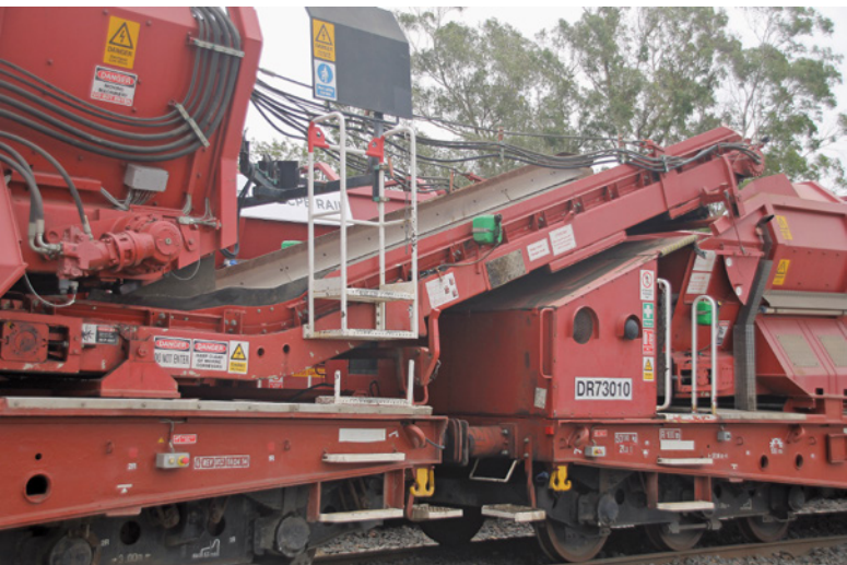
Right and Below: The conveyer system between two Sammps wagons. The operator stands on the frame and is strapped to the top of the ladder assembly to avoid falling. As the condition of the ballast is unknown until it is dug out the spoil has to be continually monitored while the ballast is being moved to prevent clogging or overloading of the conveyer belt. When a wagon is at the head of a wagon set the conveyer belt unit can be swung up to 45 degrees either side of the wagon for unloading onto the ground or other wagons. Photographed at East Greta Junction on Wednesday 14 December 2016.
