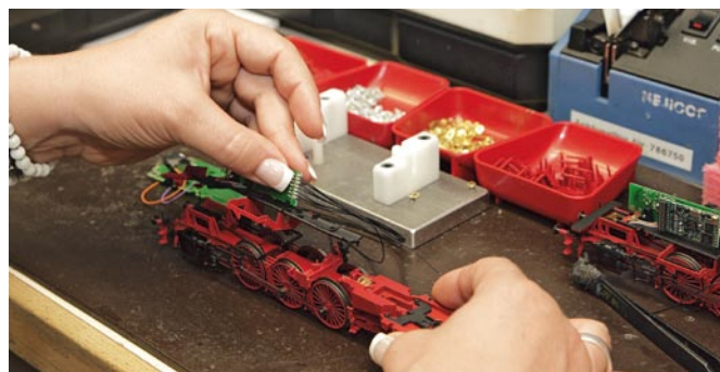
The circuit board with the electronics is carefully fitted to the lower section.
