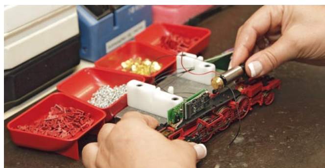
The bell-armature motor is then underneath the diecast boiler.
