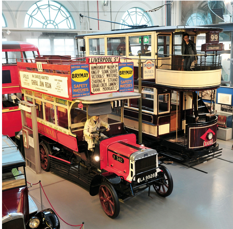
Competitors on the streets in 1910 on display together in the London Transport Museum a century later: a B-type motor bus (left) and a West Ham Corporation tram (right). Trams often had twice the capacity of early motor buses and were more reliable, but buses were more flexible and cheaper to run.
