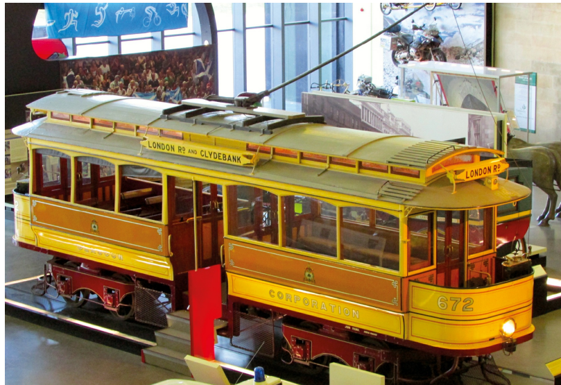
One of the first electric cars introduced by Glasgow Corporation in 1898 is now on display in the city's Riverside Museum. These early single deck trams with a central entrance/exit and an open balcony at both ends were known to Glaswegians as 'room and kitchen' cars.
