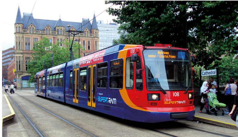
A Stagecoach Supertram at the Cathedral stop in Sheffield city centre. The original light rail system completed in 1995 is being extended over National Rail tracks to Rotherham using new tram/train units that can work with both the different operating and safety systems.
