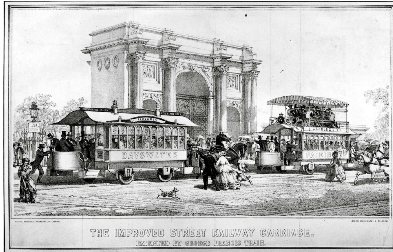
An artist's impression of George Train's first proposed street railway in London, 1860. Train's tramway was authorised as a 'temporary concession' but removed after only a few months. The vehicle design is an ornately decorated version of early American horsecars.
