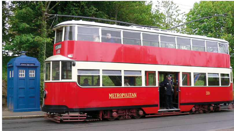
An experimental metal-bodied Feltham car with centre doors built for London's Metropolitan Electric Tramways in 1930. Tram development was abandoned soon afterwards in favour of trolleybuses. This car was sold on to Sunderland in 1950 and now runs at the National Tramway Museum, Crich.
