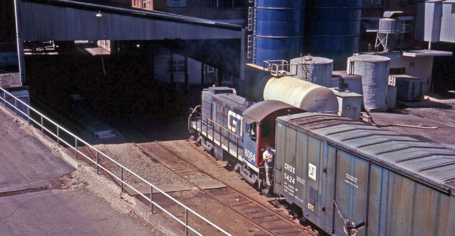
S-4 8084 pulls a load from 29 Building; CRDX 5424 is leased by General Foods for cereal loading only. To the left is 4 Building; 20 Building is at right. The GATX tank car at spot 81 probably holds vegetable oil for the “fat tanks” to the right. The blue silos hold corn and oat flour. L.R. Bolton photo
