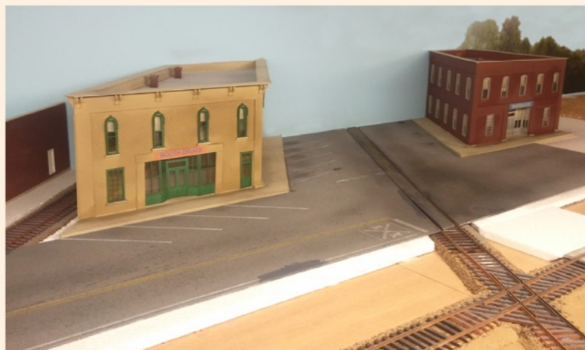
5. Dennis uses styrene sheet to elevate the street to match the rail height.
