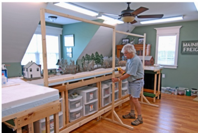
The original Strong benchwork was made using Woodland Scenics Mod-U-Rail components. Lou salvaged lumber from his HO layout and purchased new lumber for the remaining benchwork. All legs have leveling screws.
