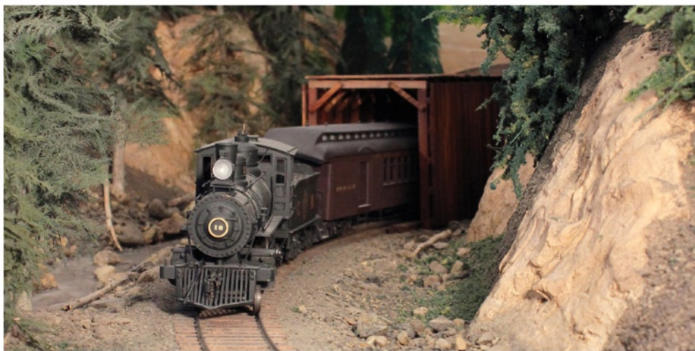
6. The prototypical wheel width and contour used on Andrew's O scale trains is evident in this photo of Ten-Wheeler no. 18 on an eastbound passenger train negotiating a 48"-radius curve approaching Arkansas Junction.
