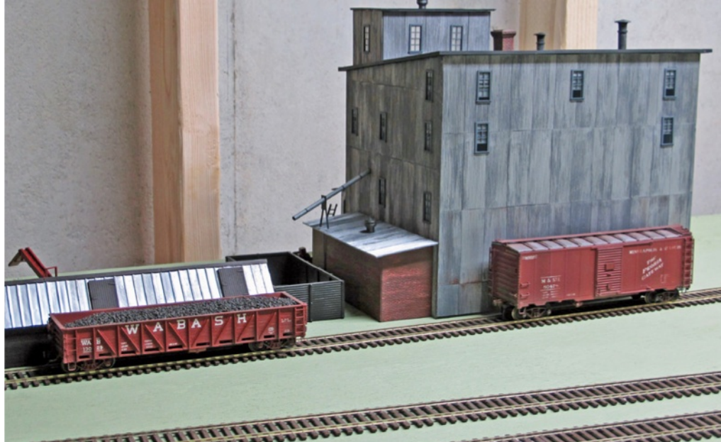
4. John began constructing industries during the planning stage. This is the Roosevelt Bros. Contracting Co., formerly a flour mill. From right to left, the scratchbuilt complex includes the main building, a power house annex, an open-topped bin for catching corn cobs, and a coal bin. In this era, coal was delivered to customers in boxcars or high-side gondolas unloaded by hand.
