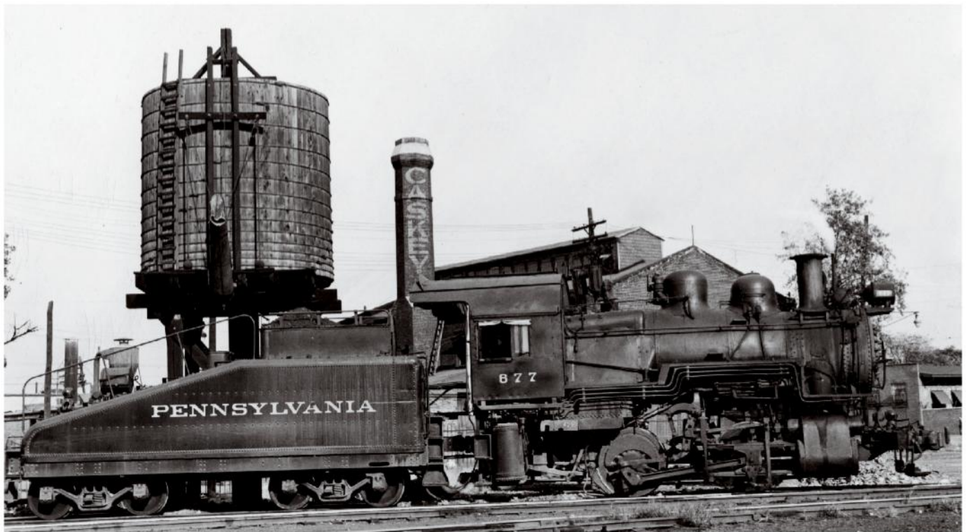
On Saturday, June 28, 1947, Pennsylvania RR no. 677 stands ready in front of the water tank at a small yard located near Richmond and Cumberland streets on the Delaware Avenue Branch. The class A5 0-4-0 switcher was the most common power used along the Philadelphia waterfront during the late steam era. Leslie R. Ross photo
