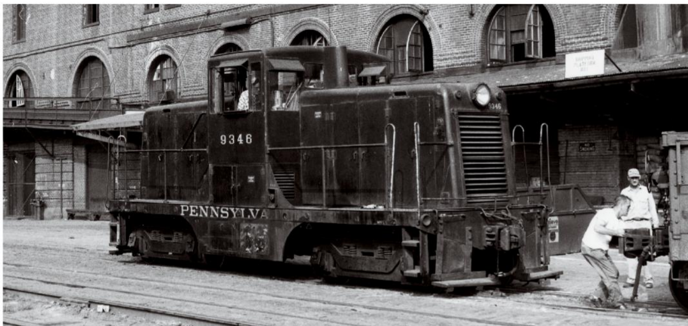
By the diesel era, General Electric 44-tonners worked the industries on the Delaware Avenue Branch. In this photo from the early 1960s, a brakeman adjusts a gondola's coupler for a push move. The engine crew will use the switcher's end sills to shove the gon along a tightly curving spur into the building. Ken Douglas photo
