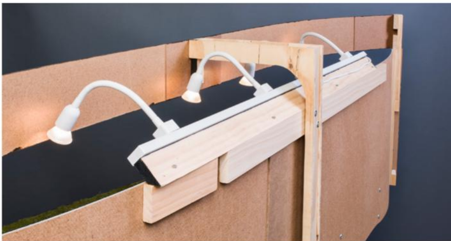
The layout has its own backdrop and light valance. David used common track-light components and gooseneck fixtures to illuminate the railroad with soft pools of light reminiscent of a partly cloudy day.
