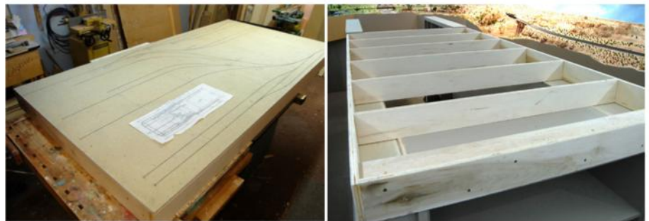
These photos show the track plan being transferred to the Homasote roadbed and the basic framework that supports the roadbed.
