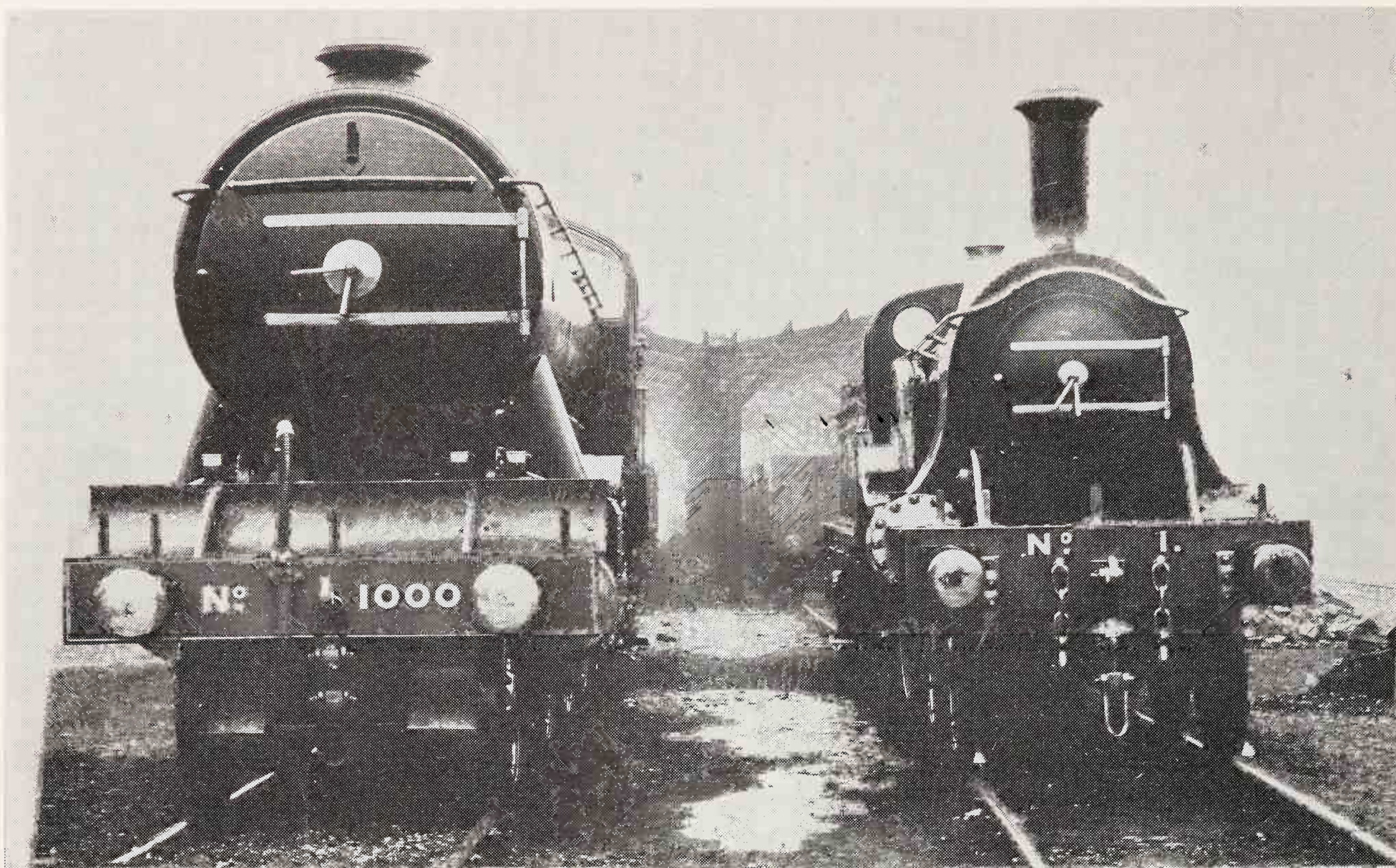
A contrast in boiler proportions: the first of the 3-cylinder 2—6—0s alongside the Stirling eight-footer No 1
