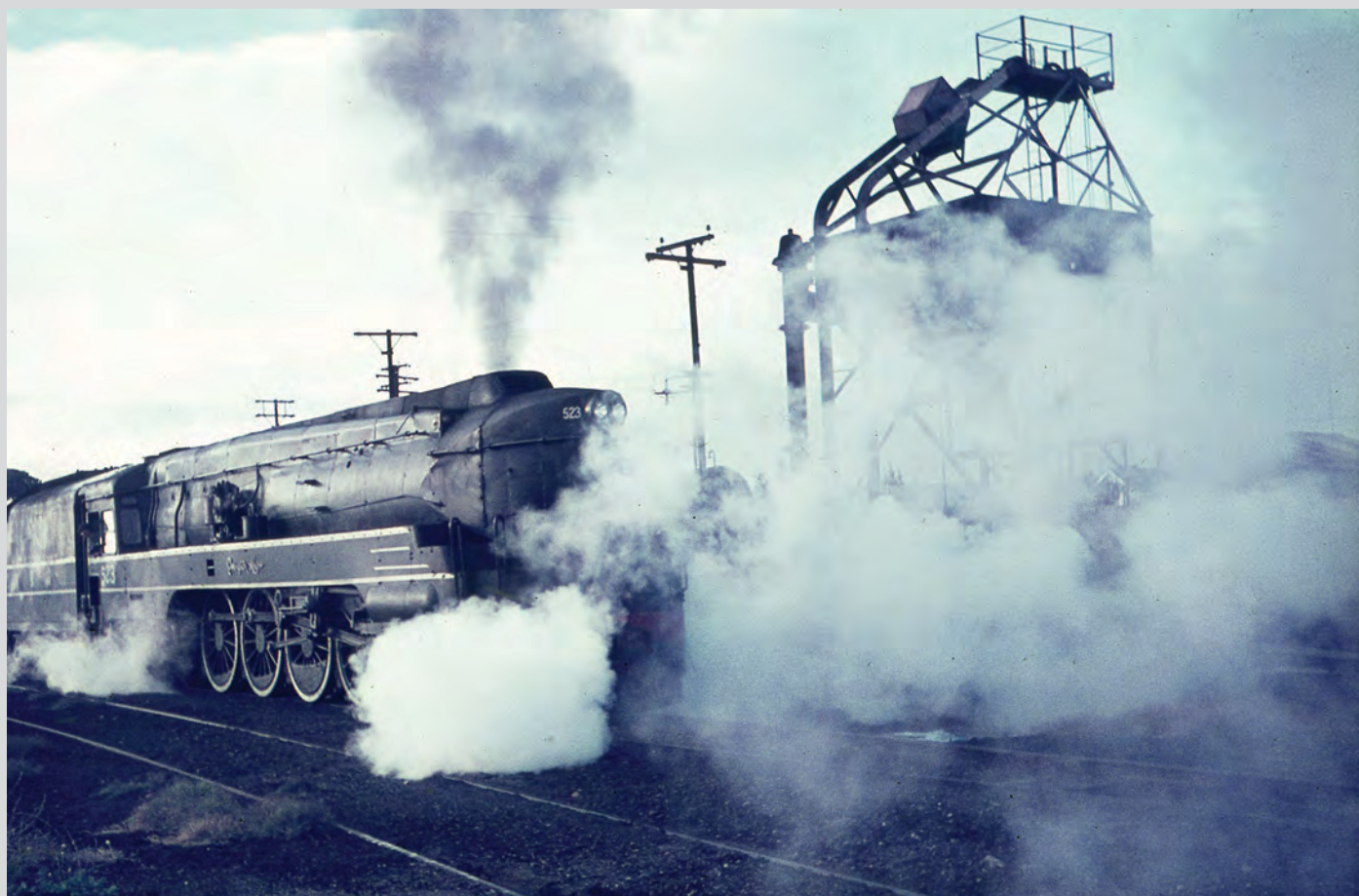
SAR 520 Class 4-8-4 streamlined locomotive 523, Essington Lewis , blows down adjacent to the 45-ton coaling plant at Mount Gambier locomotive depot in April 1966 as it is prepared to work an ANZAC Day ARHS tour train back to Adelaide. RODNEY BARRINGTON PHOTO
