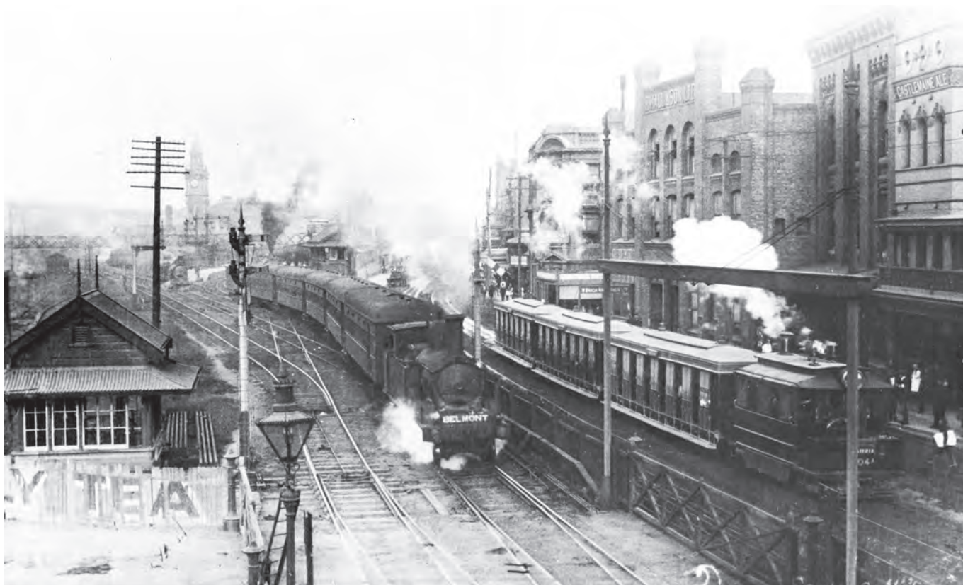
E Class 2-6-4 locomotive No. 533 heads a Newcastle suburban train approaching the Market Street level crossing with a 'BELMONT' destination board as it passes steam tram motor No. 104A heading three trailers to Mayfield.
