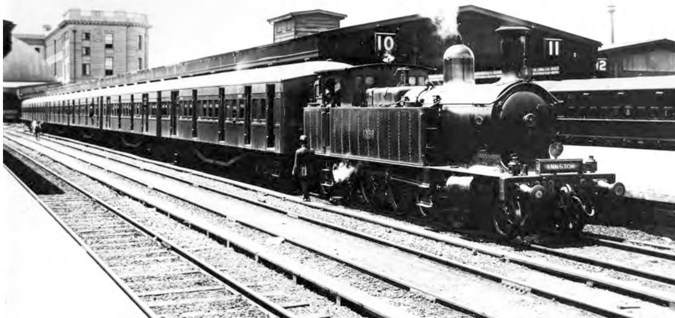
S1238 prepares to head a six-car 'Bradfield' set out of Sydney No.10 Platform for Bankstown in 1921 or 1922. The roller blind indicator shows 'BANKSTOWN' and the white discs under the funnel and centre of buffer beam are the headcode at the time for Bankstown trains. ARHSNSW RAILWAY RESOURCE CENTRE, 009354
