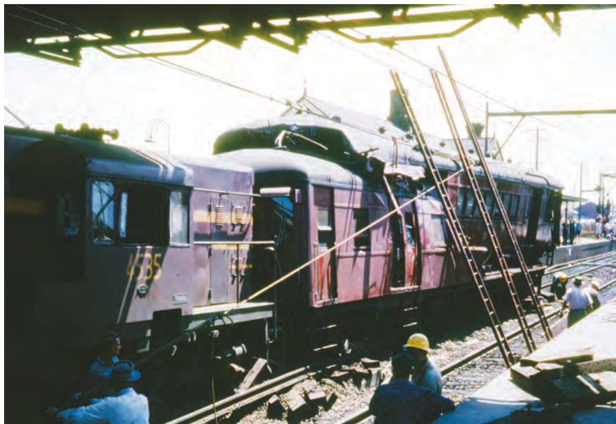
Telescoped suburban train carriages at Liverpool Station after the collision resulting in a freight train headed by locomotive 4535, which ran into the rear of the suburban train on 31 October 1965. R B CLARKE PHOTO, ARHSNSW RAILWAY RESOURCE CENTRE, 290867
