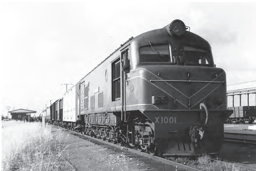
WAGR X Class 2-Do-2 locomotive X1001, YALAGONGA, heads a mixed train at Moawa Station on the Mullewa Line on 3 November 1970. X1001 was the first mainline diesel-electric locomotive to enter service in Western Australia on 8 March 1954. J BECKHAUS PHOTO, ARHSNSW RAILWAY RESOURCE CENTRE, 032031
