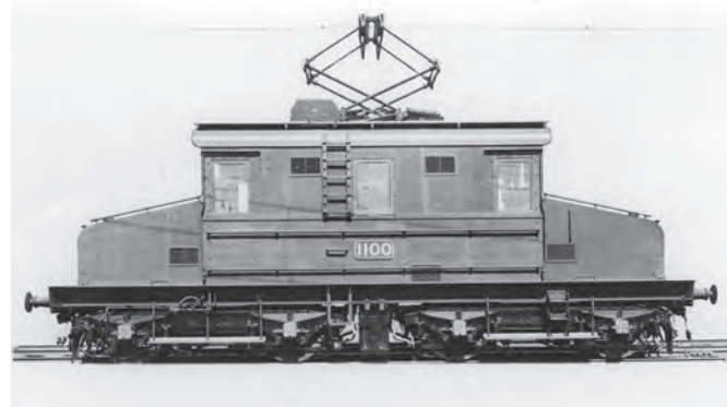
Victorian Railways publicity photograph of 1100 Class Bo-Bo electric locomotive No. 1100 that entered service on 20 July 1923. VICTORIAN RAILWAYS, ARHSNSW RAILWAY RESOURCE CENTRE, 021924A
