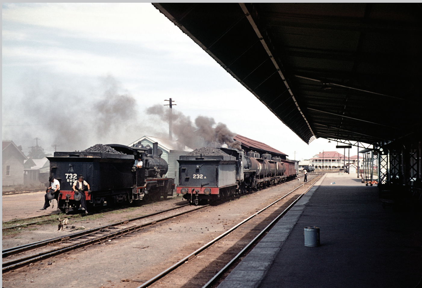
Queensland Railways steam locomotives in action as PB15 Class 4-6-0 No. 732 and AC16 Class 2-8-2 No. 232 A shunt wagons at Dalby Station on a lazy afternoon circa 1965. E G SKILLER PHOTO, ARHSNSW RAILWAY RESOURCE CENTRE, 090778
