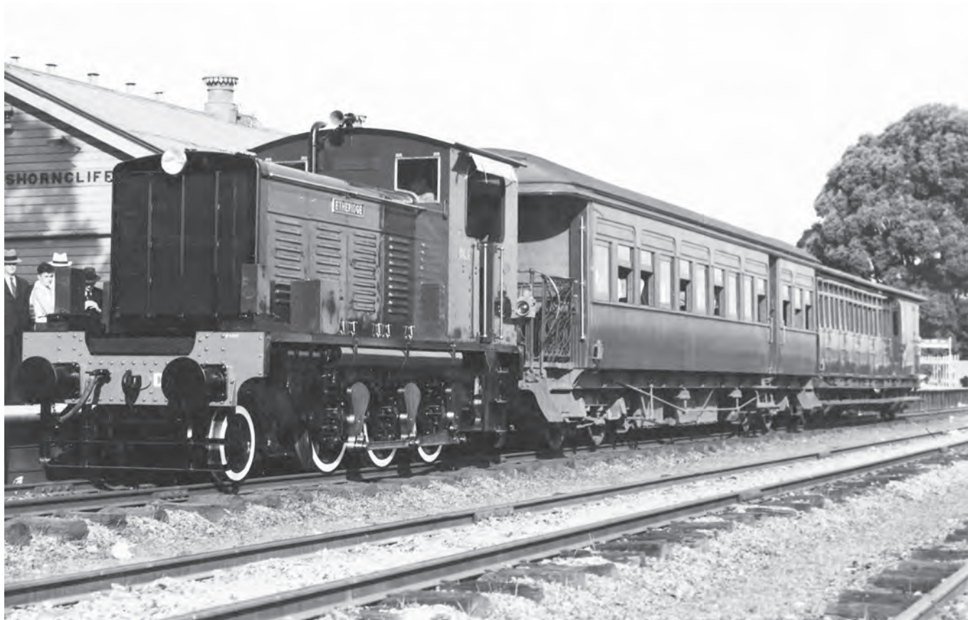
The Queensland Railways 2-6-0 diesel-mechanical locomotive DL1 ETHERIDGE on its trial run at Shorncliffe Station in Brisbane in 1939. This was an Australian pioneer diesel-powered locomotive. QR photo, ARHSNSW RAILWAY RESOURCE CENTRE, 025338
