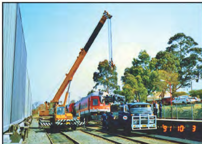
The mobile crane, having lifted the rear DEB motor car No. 958, is lifting the damaged motor bogie onto a SRA lorry at Nowra on 3 October 1991. BRIAN ARNDELL PHOTO
