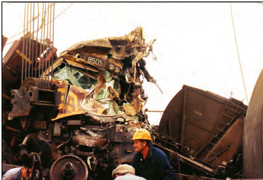
Rescue workers place the hook of a mobile crane to lift damaged wheat hopper wagons at Valley Heights on 19 July 1982. The tangled mess of electric locomotive 8505's driving cabin is evident. TED DIXON PHOTO
