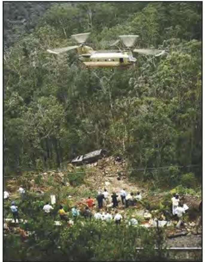
The RAAF heavy-lift helicopter preparing to raise a cut-up section of the V-set driving trailer car from the gorge adjacent to Glenbrook Tunnel in January 1976. CLIVE KEENAN PHOTO
