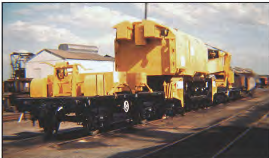
The Krupp crane at Enfield after upgrading to 150-tonne capacity. It was subsequently based at Lithgow Loco Depot. ALAN PARKINSON COLLECTION
