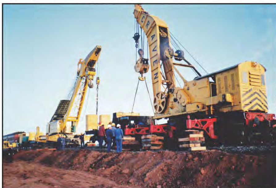
Setting up the heavy cranes by attaching concrete weights to balance both cranes prior to dragging each locomotive up to the track. BOB O'LOUGHLIN PHOTO
