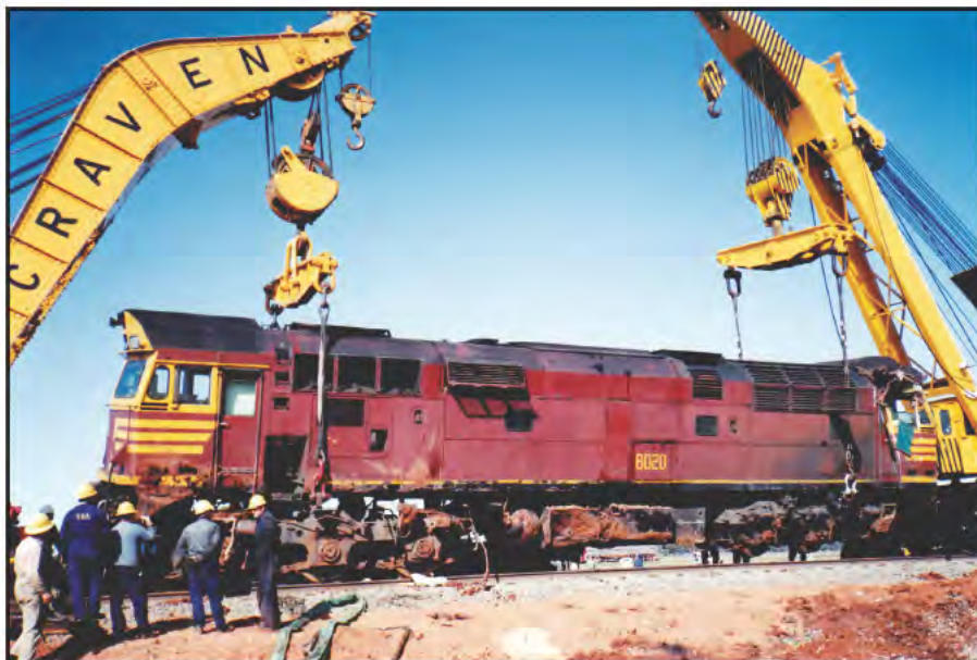
The Craven and Krupp the breakdown cranes lifting damaged locomotive 8030 onto the track near Yarrabandai in August 1992. BOB O'LOUGHLIN PHOTO
