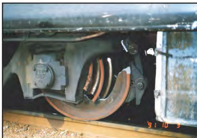
The shattered leading motor bogie driving wheel of trailing DEB motor car 958 at Nowra on 9 October 1991. BRIAN ARNDELL PHOTO
