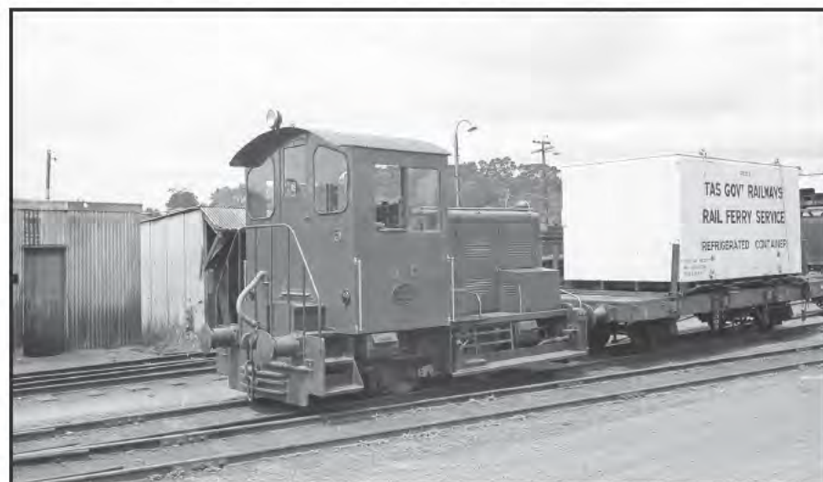
The six U Class diesel-mechanical locomotives were powered by a 102hp Gardiner engine, limiting them to light shunting duties. Here U5 shunts wagons for the TGR Ferry Service circa 1962. ARHSNSW RAILWAY RESOURCE CENTRE, 401329
