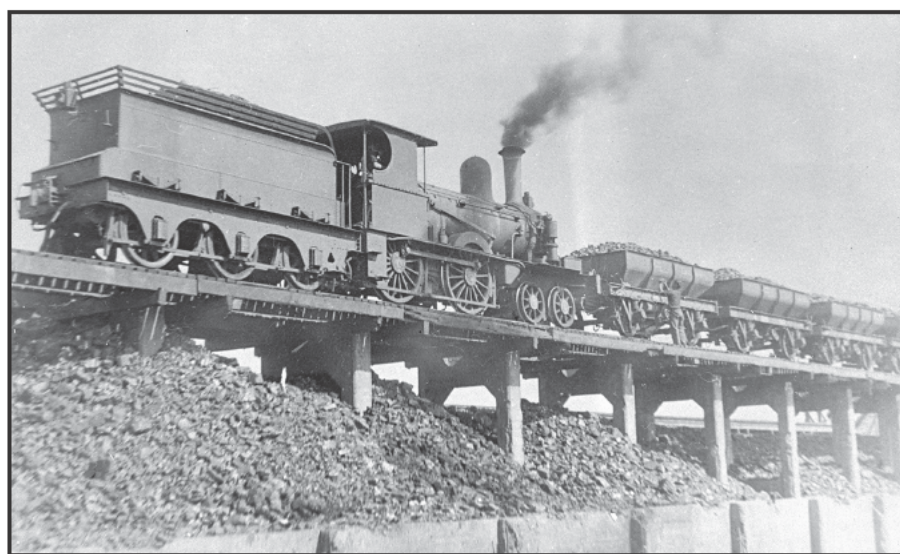
Following their use on construction trains, the six ex-NSWGR 4-4-0 D Class locomotives saw limited use on shunting and locomotive depot duties. Here an unidentified member of the class pushes BAS Class four-wheel bottom discharge hopper wagons over the coal unloading ramp at Port Augusta locomotive depot. NATIONAL RAILWAY MUSEUM, AN8804201-03
