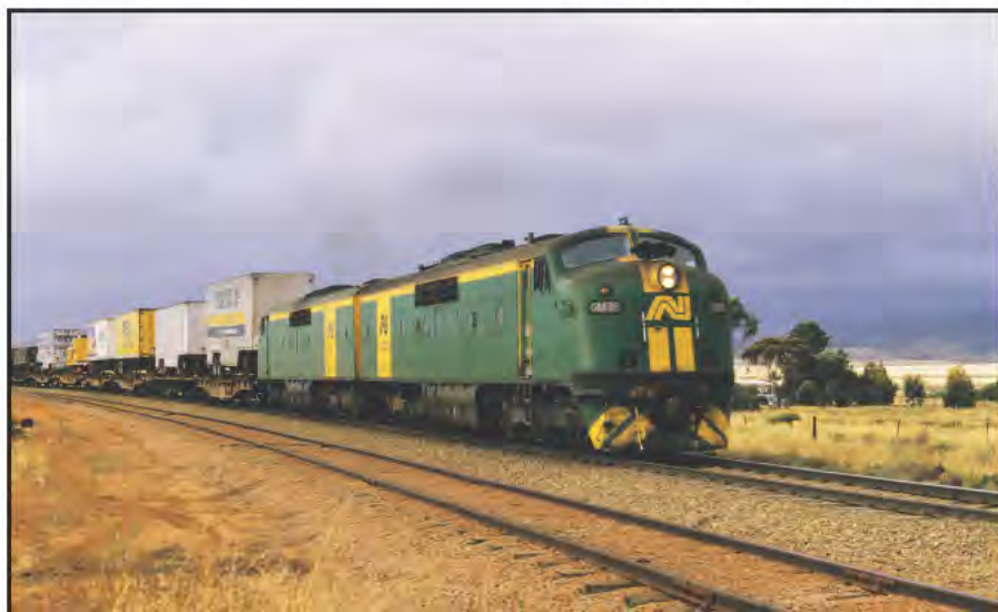
Commonwealth Railways GM12 Class 1340kW locomotives GM35 and GM32 head a south-bound train of piggyback road trailers from Port Augusta on 18 October 1981. J LUNT PHOTO, ARHSNSW RAILWAY RESOURCE CENTRE, 263752
