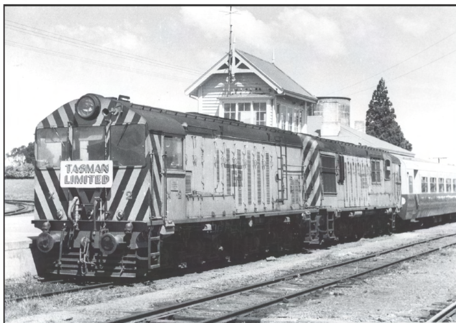
TGR pioneer diesel-electric locomotives X2 and X1 were still in active service on 27 April 1971 when they were photographed in charge of the Tasman Limited train at Western Junction. ARHSNSW RAILWAY RESOURCE CENTRE, 021432
