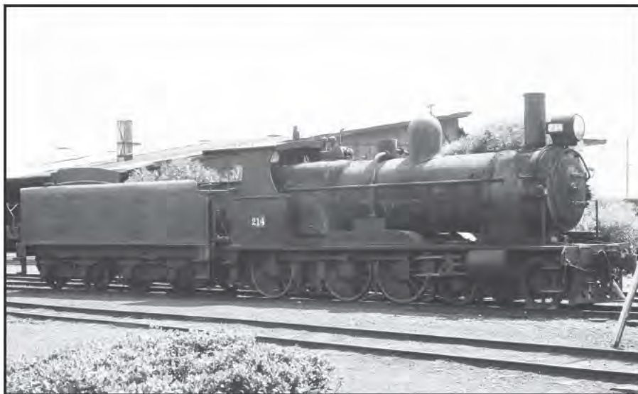
The SAR Rx Class 4-6-0 broad gauge locomotives introduced from 1909 remained in service until the end of steam, with Rx 214 being the last to operate at Tailem Bend on 1 December 1967. P LE ROUX PHOTO, ARHSNSW RAILWAY RESOURCE CENTRE, 242413
