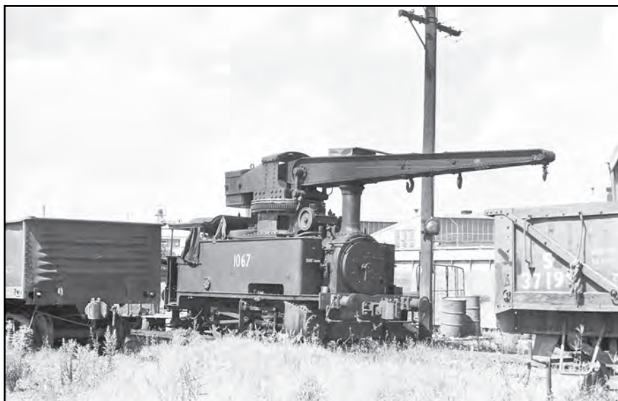
0-4-0T steam crane locomotive No. 1067 shunting at Clyde wagon workshops on 1 January 1972. A GRUNBACH PHOTO, ARHSNSW RAILWAY RESOURCE CENTRE, 206645
