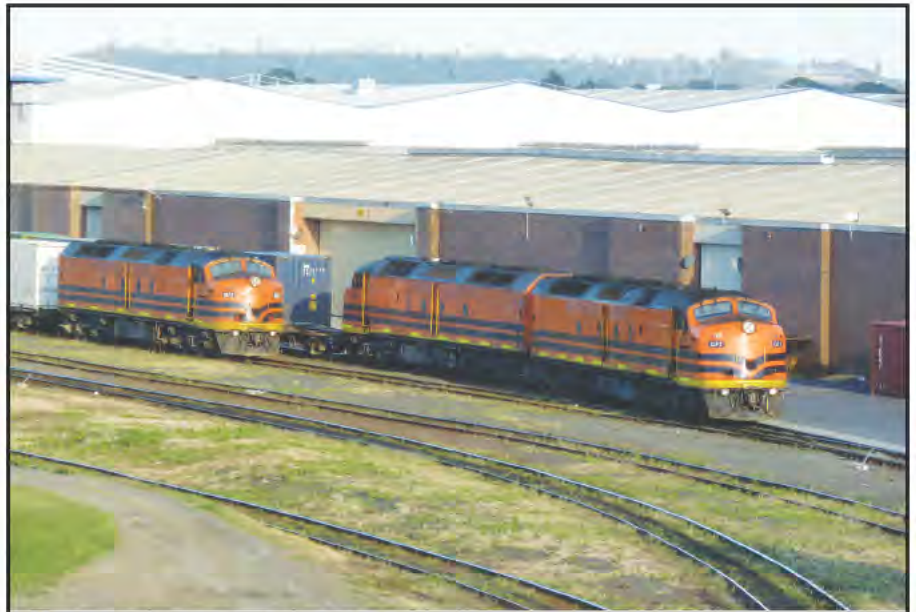
Under private ownership, CLF/CLP Class 2240kW diesel-electric locomotives travelled widely on the standard gauge Australian network. Here CLF locomotives 3, 7 and 2 head freight trains at Sydney's Yennora Terminal.
