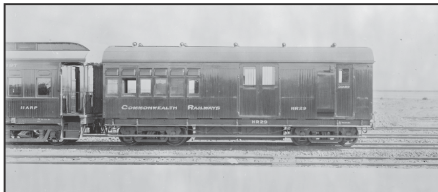
Guard / Crew Van HR29 was also photographed about the time of the opening of the Trans-Australian Line. Originally a guards van with two passenger compartments, they were rebuilt to provide crew accommodation when the through line opened (see p22). PHOTOGRAPH CHRIS DRYMALIK COLLECTION
