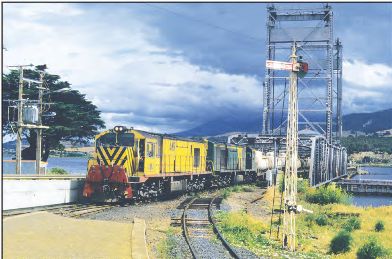
Storm clouds hang over Mount Wellington, but mainline Co-Co diesel-electric locomotives ZA3 and ZA2 are bathed in sunlight as they cross the lifting bridge into Bridgewater Station with a mixed freight train in the 1980s.
