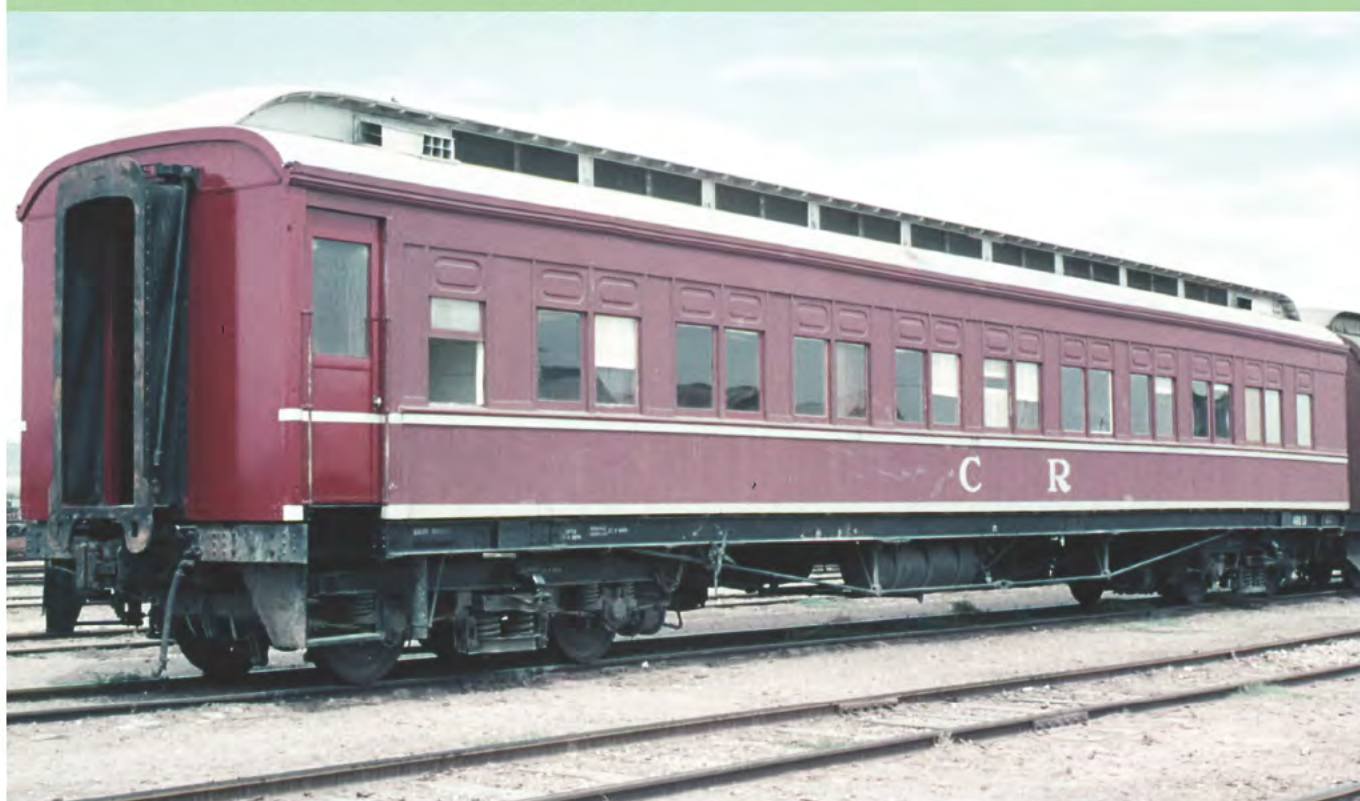
Commonwealth Railways car ARB 13, photographed on 7 March 1969, shows the changes that occurred to these vehicles in the half century following their construction. An early photograph is presented on page 21. The end platform at the right-hand end was enclosed early in its history to enable the installation of showers, Commonwealth Railways was the first to provide this facility for passengers. The opposite end-platform was enclosed on some of these cars when they were improved during the late 1940s. This carriage retained the moulded panels above the windows which were a feature, but they were replaced with plain panels on some cars during the 1960s. This carriage has the Minden Deutz bogies which replaced the original outside equalised bogies during the 1960s. These bogies were supplied with the cars built in Germany between 1952 and 1954, being replaced with Bradken-built Commonwealth bogies obtained for the steel carriages. PHOTOGRAPH BY JOHN BECKHAUS
