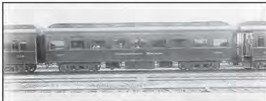
Lounge carriage AF24 was photographed about the time of the opening of the line. The lounge cars had wide windows with a long moulded wooden panel above each window. As they had to use existing R A flat wagon underframes which while lengthened were shorter than the underframes used for the other passenger cars, the lounge cars had only end doors to adjacent cars but no side doors. PHOTOGRAPH CHRIS DRYMALIK COLLECTION.
