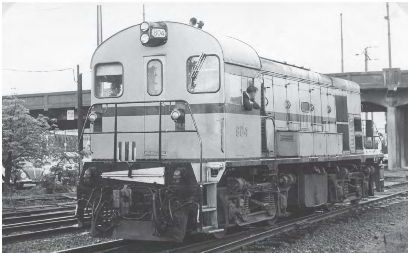
A very clean Bo-Bo diesel-electric No.804 is about to pass under the Bakewell bridge and past the Mile End North signal cabin en route to the Mile End Diesel Depot. The two vertical yellow lines on the train designator immediately above the coupling indicate that the loco has travelled 'light engine' from Port Adelaide. ARHSNSW RAILWAY RESOURCE CENTRE, 242646. Part 2 of David Matheson's 'From Steam to Diesel and Electric' article commences on page 4.
