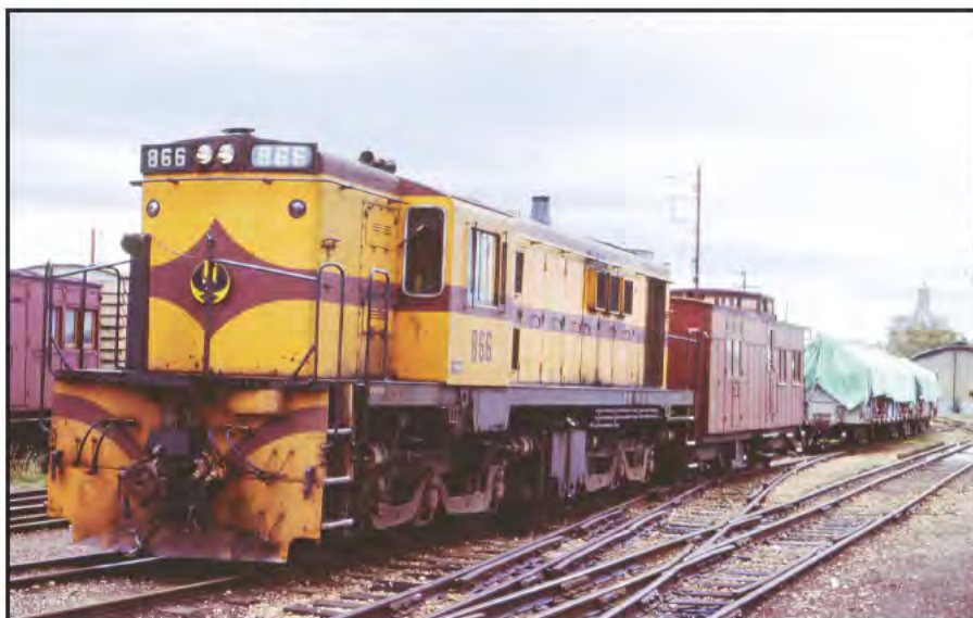
Narrow gauge SAR 830 Class Alco diesel-electric locomotive shunting a guard's van and freight wagons on dual-gauge track at Gladstone on 1 December 1977. R GRAF PHOTO, ARHSNSW RAILWAY RESOURCE CENTRE, 395661
