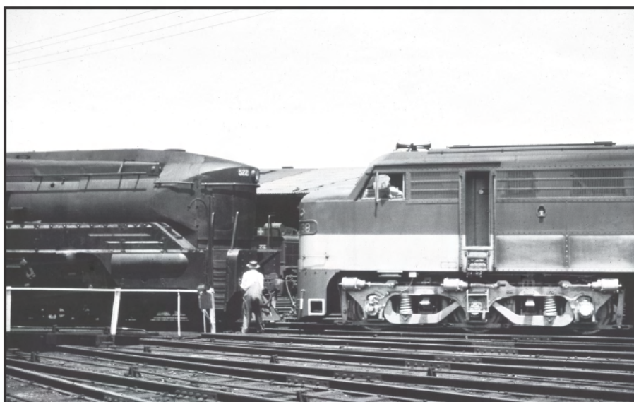
Transition from steam to diesel on the SAR. 520 Class 4-8-4 No. 522 being placed on the turntable at Mile End by 930 Class diesel-electric locomotive 938 in the early 1960s. K BOWEN PHOTO, ARHSNSW RAILWAY RESOURCE CENTRE, 169736
