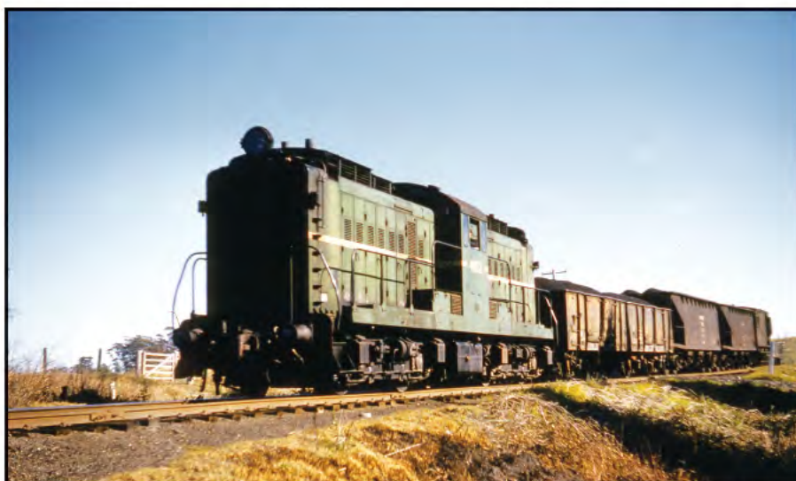
The British Thomson-Houston 41 Class diesel-electric locomotives were powered by two Paxman engines, but were ill-suited to Australian conditions and spent most of their time on secondary duties. Here 4102 heads a short coal train on the Campbelltown–Camden branch line circa 1961. I K WINNEY COLLN, ARHSNSW RAILWAY RESOURCE CENTRE, 161969
