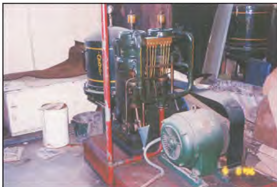
The electric powered two-cylinder pump for the carpet runner cleaning machine at Sydney Terminal Station, 9 August 1996. The machine was a British Vacuum Cleaner Company product. GARRY ARMSTRONG PHOTO
