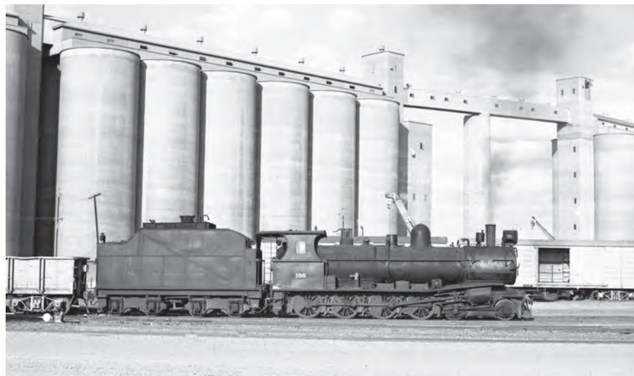
SAR 4-8-0 narrow gauge locomotive T186 shunting at Port Pirie with the wheat silos dominating the background. A GRUNBACH PHOTO, ARHSNSW RAILWAY RESOURCE CENTRE, 201523
