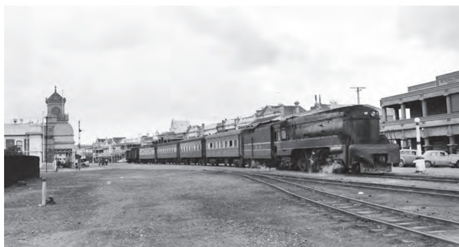
Broad gauge 4-8-4 locomotive No. 522 arrives at Ellen Street with the morning passenger train from Adelaide. The train stands on a single mixed gauge track and it will shortly propel back to Port Pirie Junction. All other tracks in Ellen Street are narrow gauge. To the left is the grand 'gingerbread' style street-facing station built that replaced a modest skillion roofed structure in 1902. Today the tracks have been removed from the street, and the building remains as a museum, but the tower never had its promised clock fitted. NATIONAL RAILWAY MUSEUM, AZ04913.
