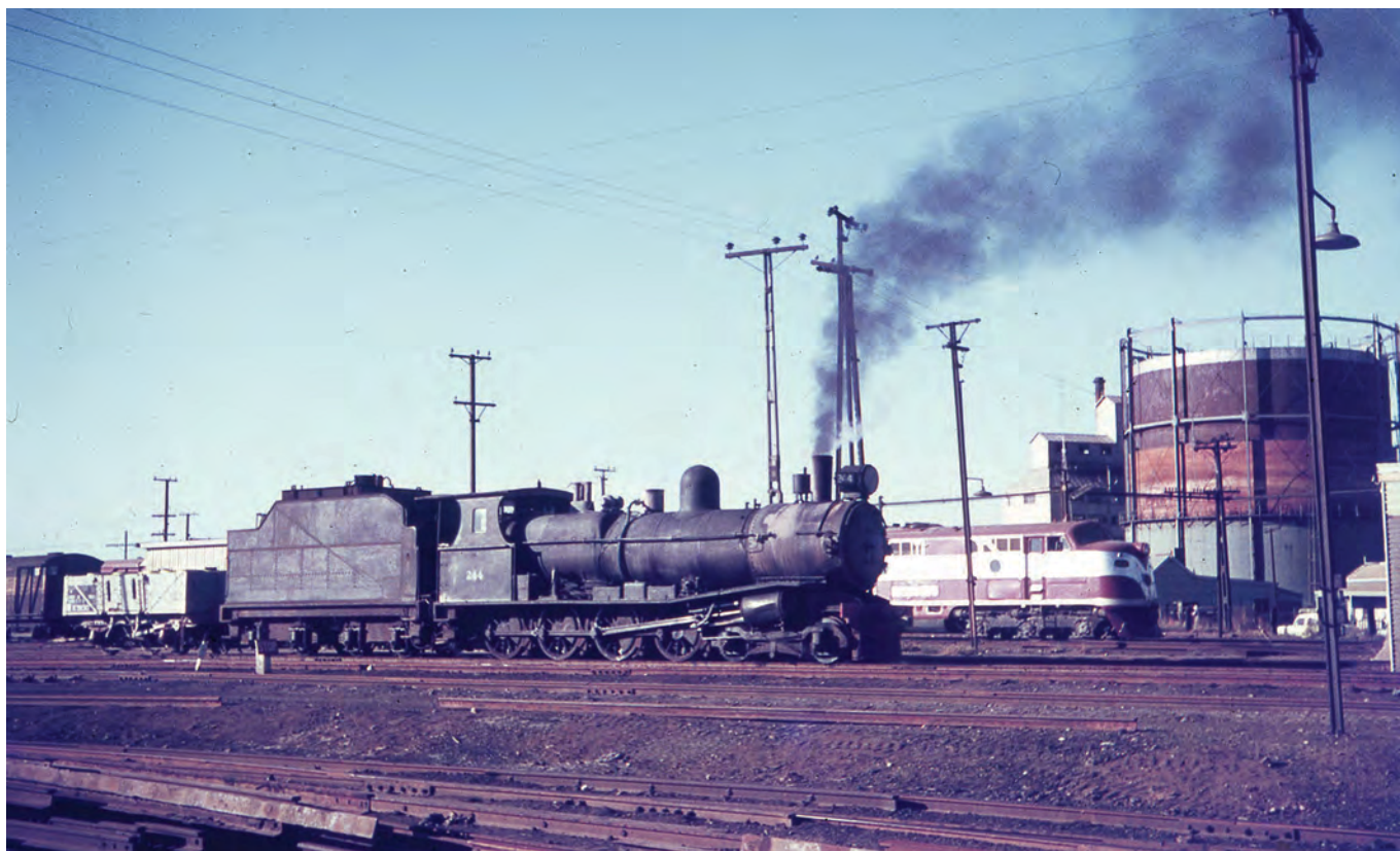
T Class oil-burning 4-8-0 No. 244 shunting in Port Pirie yard in May 1965 as a Commonwealth Railways GM Class diesel-electric locomotive idles in the background. RODNEY BARRINGTON PHOTO
