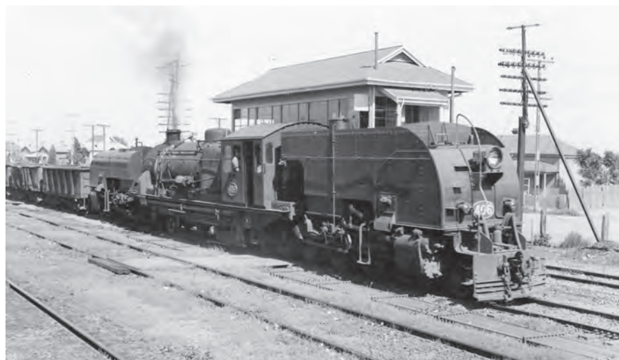
At around lunchtime, Garratt locomotive No. 406 clatters past the signal cabin into Port Pirie Junction with a freight train from Peterborough. The locomotive is running bunker first as it was most likely turned at Gladstone so that it could return funnel first, as the narrow gauge loco depot turntable at Port Pirie was too small for the Garratt locomotives. NATIONAL RAILWAY MUSEUM, AZ21641
