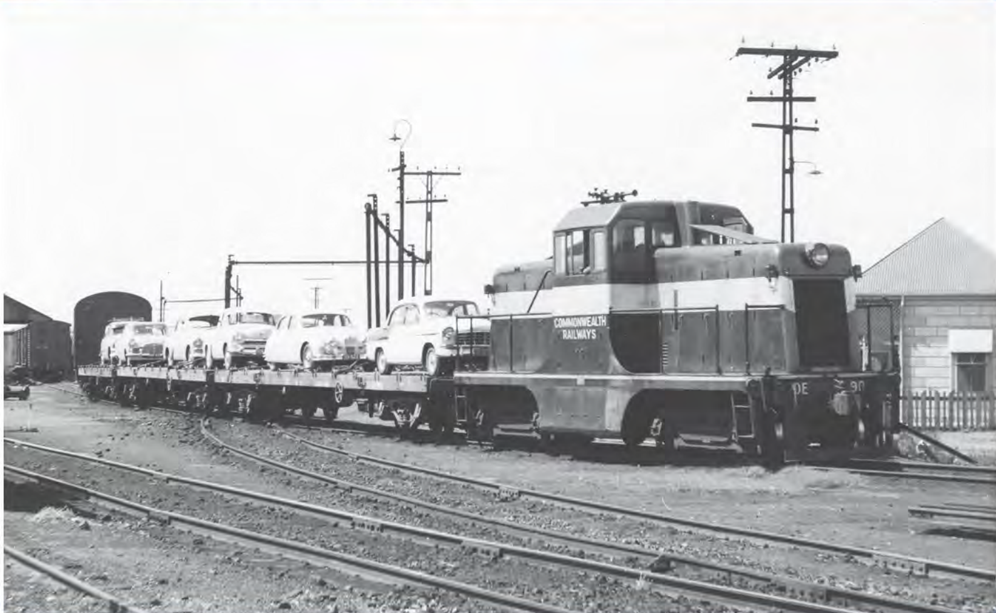
Former US Army diesel-electric Bo-Bo shunting locomotive DE91, now in the Commonwealth Railways maroon and silver colour scheme, shunting Commonwealth Railways flat cars carrying passengers' motor vehicles for attachment to the 'Trans' at Port Pirie on 29 December 1965. Only two cars per wagon! Rodney Barrington's memories of travel by rail to 'Pirie' in the 1960s commences on page 23. J BECKHAUS PHOTO, ARHSNSW RAILWAY RESOURCE CENTRE, 042617
