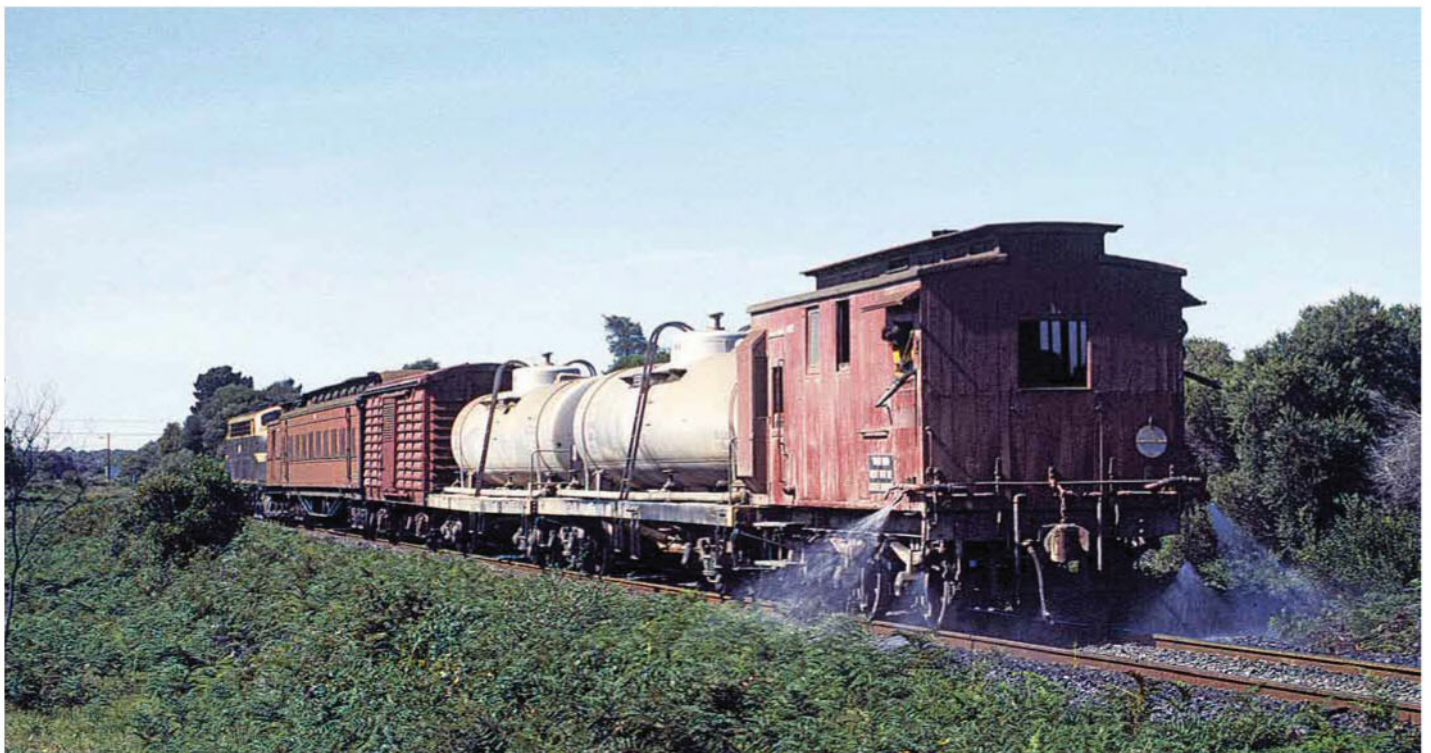
As the train passed, John Dennis also shot this view from the rear, showing the weed killing spray in use.
