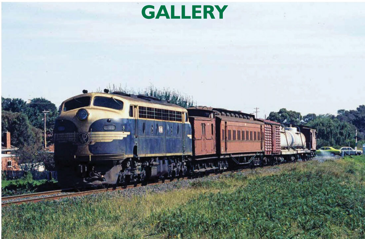
▲ John Dennis's photograph shows the prototype 'Weedex' train, hauled by B65, spraying the lineside growth near McMahon's Road, Frankston, on Wednesday 5 April 1978. Other than the replacement of crew accommodation car 1HW with a repurposed passenger car, the train is substantially as modelled by Don, though this run only required two WA tank wagons, rather than the four Don is in the process of constructing.
