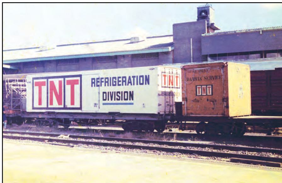
Thomas Nationwide Transport refrigerated container, compared with a standard 'Darwin Service' container photographed at Hamilton, QLD. IMAGE ERIC LYON, COURTESY AMRA QLD BRANCH COLLECTION
