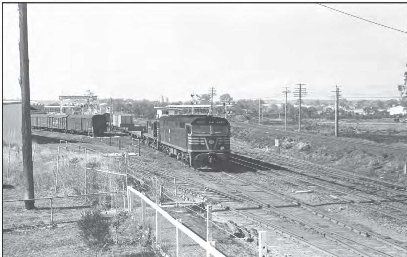
Standard gauge Alco 'Jumbo' mainline locomotive 44211 and a 48 class branchline locomotive shunt a container train into the TNT Alltrans Salisbury container depot in mid-1978, while three bogie box cars sit in the adjacent siding. The weather protection awning constructed in 1974 is behind the electricity pole. GREG CASH IMAGE
