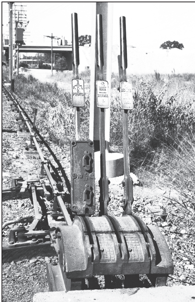
The signal levers at Salisbury with a Duplex Annett lock on No. 1 lever with two key slots in 1982. P BARKER IMAGE
