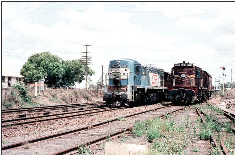
Clyde-built 1502 class diesel-electric locomotive 1526 heads a Beenleigh bound suburban train through Salisbury as NSW branch line locomotive 4847 shunts vans on the standard gauge in the late 1970s. GREG CASH PHOTO
