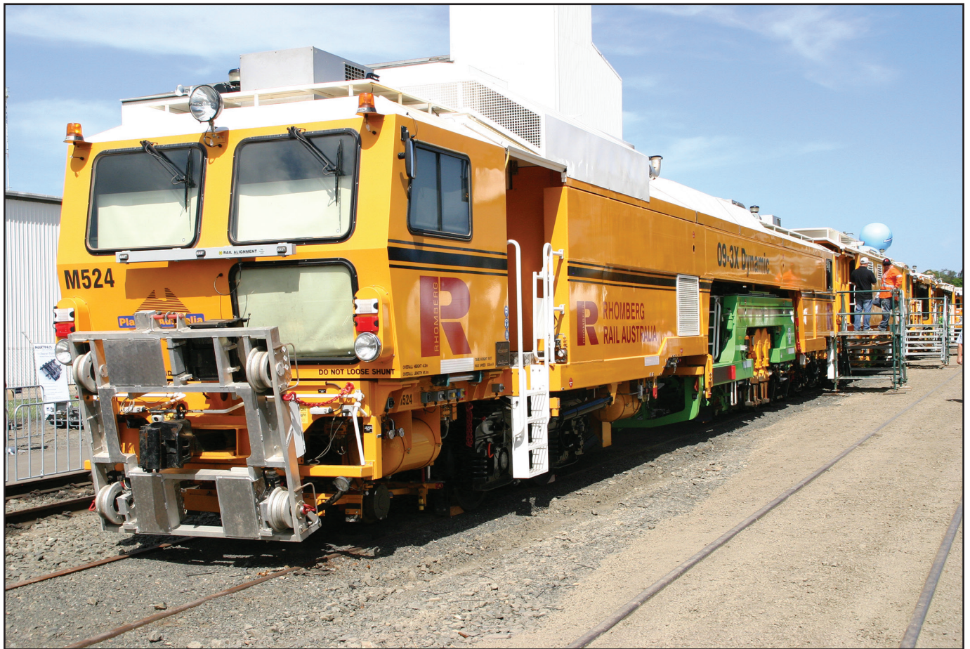
Mechanised track maintenance has come a long way since the 1960s, as evidenced by this Plasser Australia 09-3X Tamping Express machine on display at the Rail Track Association of Australia exhibition at Clyde on 27 February 2013. JOHN BECKHAUS PHOTO
