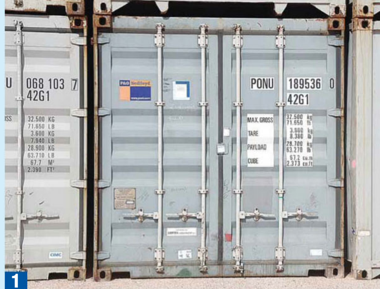
1 The end doors on containers show the container code (PONU), number (189536) and check digit (0), as well as the container type (42G1) and all the vital statistics for weights and capacity. This container was in a Maersk container stack at Kelso on 2 March 2015.
