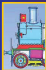
Superheated built-up smokebox
