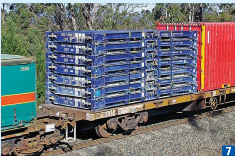
7 No fewer than seven Cronos 22P3 'flat racks' have the ends collapsed and are nested to almost 9' high on transfer from Perth to the east coast. The straps are used to ensure the folded down ends on the top container do not accidentally fly up during transit on RQCY863-Q on 23 July 2016.
