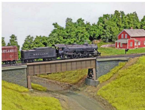
5. United States Railroad Administration 2-8-2 light Mikado no. 37 rolls southbound freight No. 20 over the Neshobe River and into Brandon, Vt. Many deck-girder bridges had distinctive "legs" to cope with masonry approaches designed originally for wood spans.
