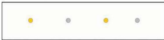
Wide, deep baseboards with two alignment dowels and two coach bolts
