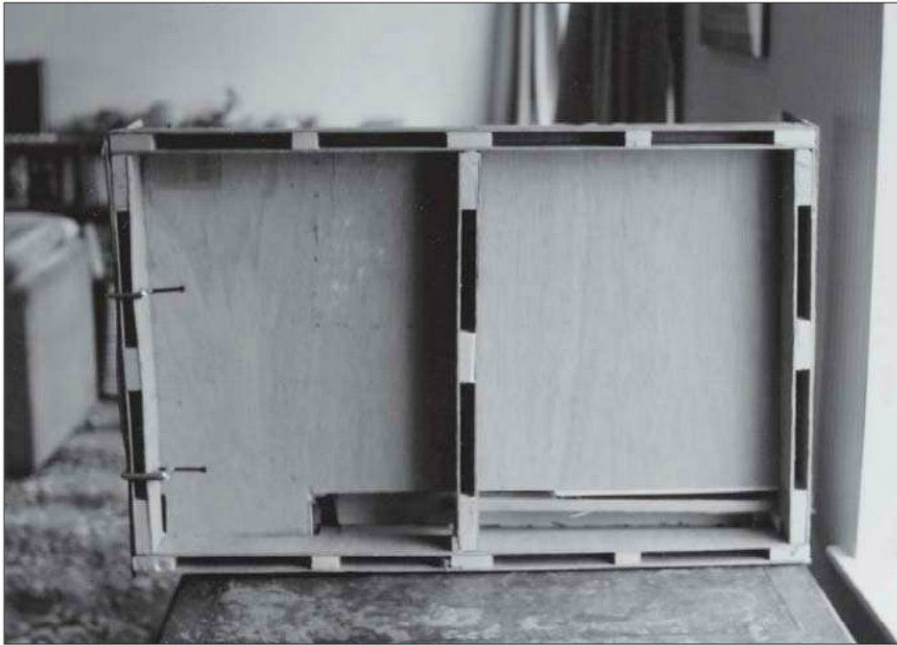
Ply beams used as a conventional frame for a solid-top baseboard.
