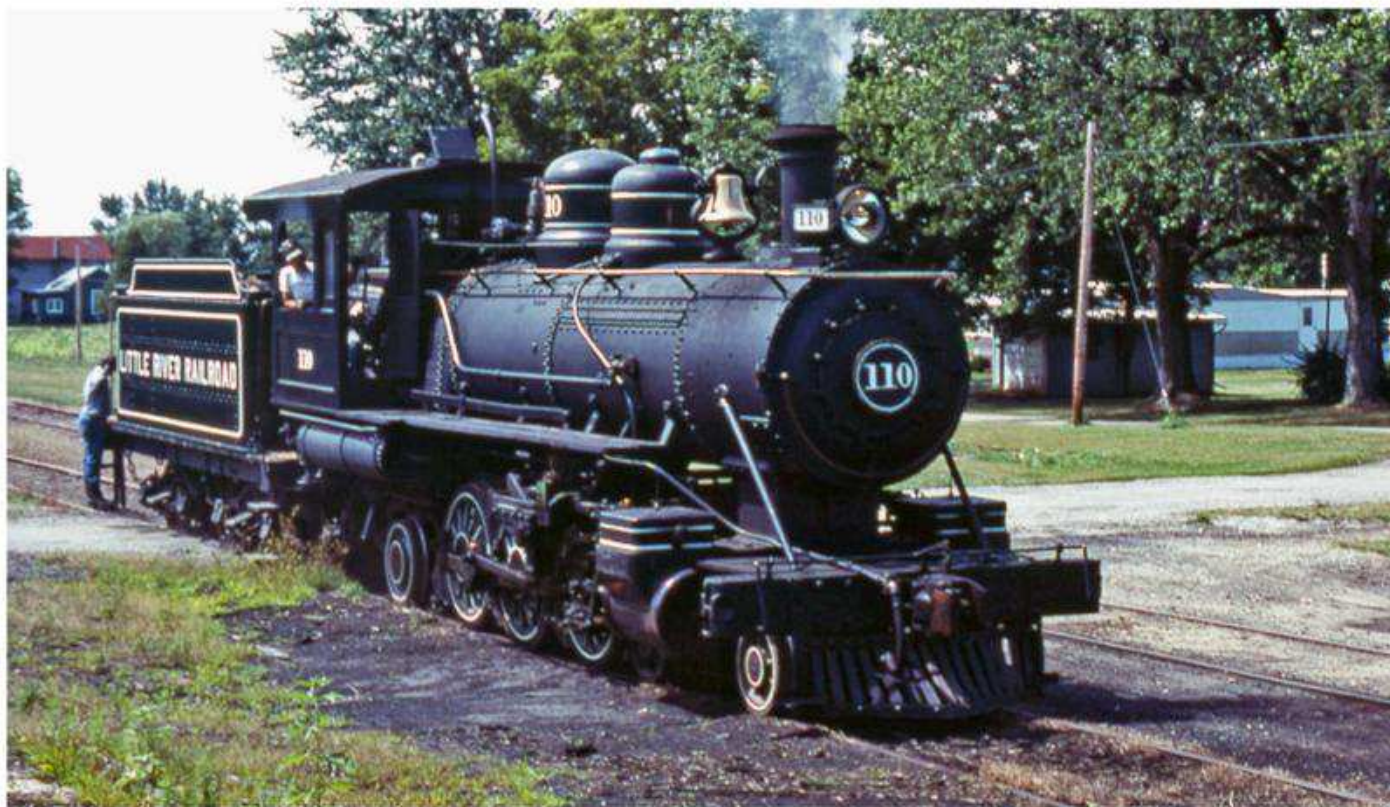
Avert your eyes – this smallest of standard gauge Pacifics isn't properly attired for public viewing! Lacking lagging to retain boiler heat and jacketing to dress it up, the 4-6-2 was ready for another workday in 1978. Fully dressed, no. 110 continues in steam in 2018. Doug Leffler photo
