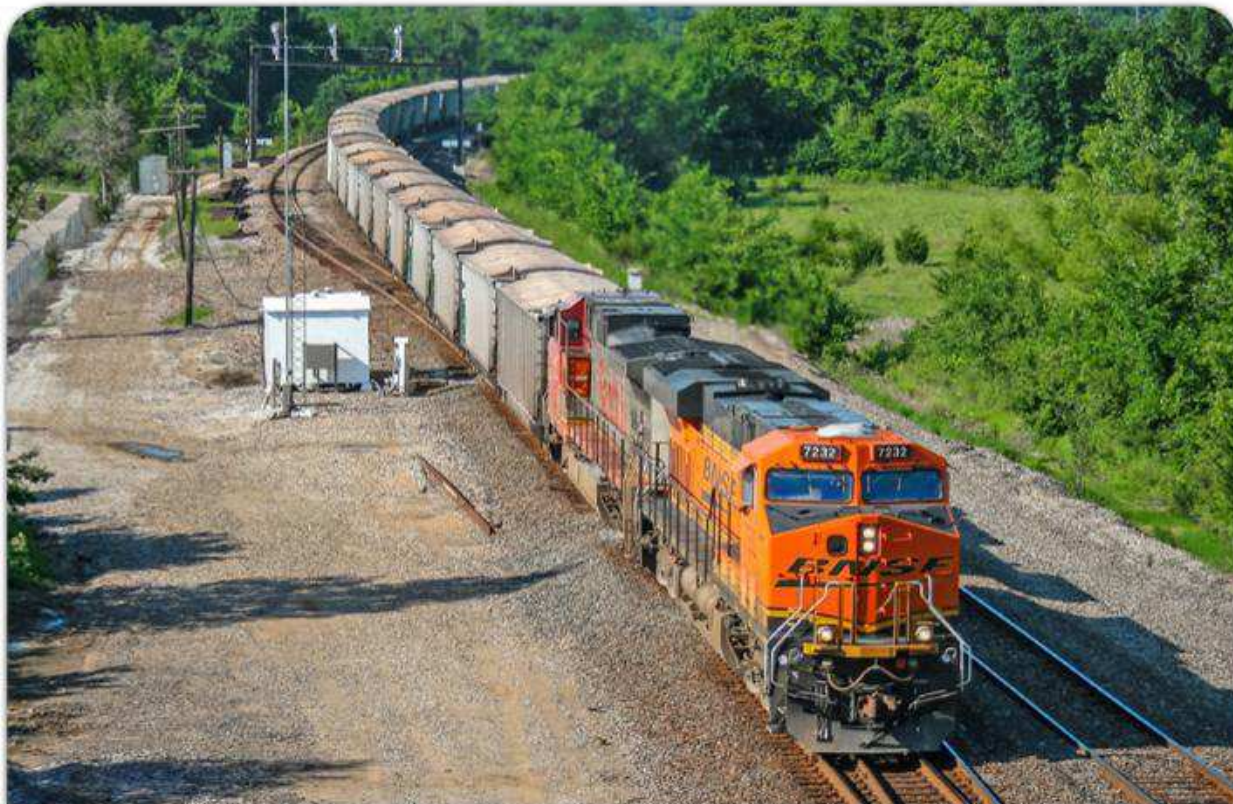
A BNSF Ry. unit train of protein gondolas – former BethGon Coalporter bathtub gonds fitted with Shur-Lok brand roll tarps – rolls south through Shawnee, Kan., in June 2009. The lading is Cargill Sweet Bran animal feed. Zach Pumphery photo
