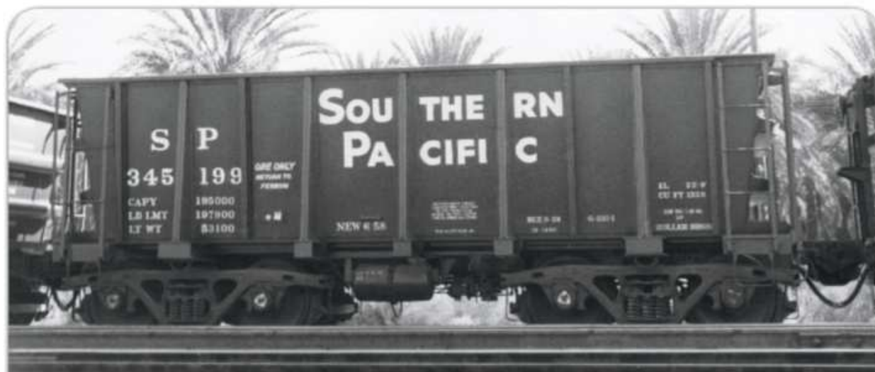
The Southern Pacific added 600 of these 26-foot house-built ore gondolas to its roster in 1958. Later, Model Die Casting would add an HO scale version to its Roundhouse line. Ray Savage photo
