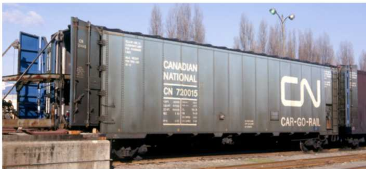
③ Canadian National began using double-deck boxcars for carrying autos in 1957. The cars, which could be loaded and unloaded circus-style, foreshadowed the auto racks that were soon to come. J. David Ingles collection
