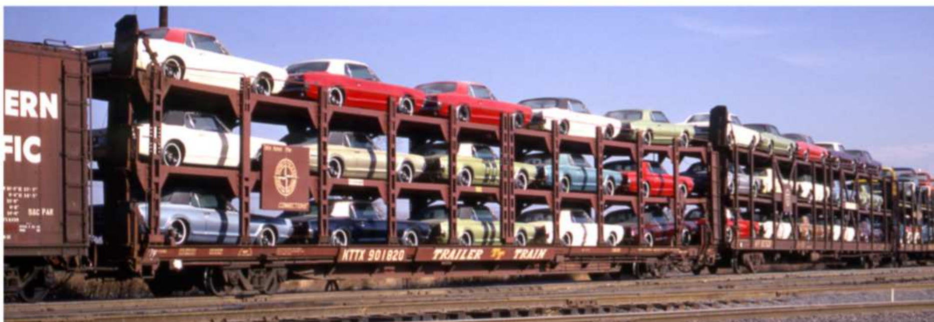
7 The KTTX reporting marks indicate a tri-level with hinged deck ends. The Paragon “ladder-style” rack rides on a low-level American Car & Foundry flatcar; note the deck level compared to the standard “Western” rack at right. J. David Ingles collection
