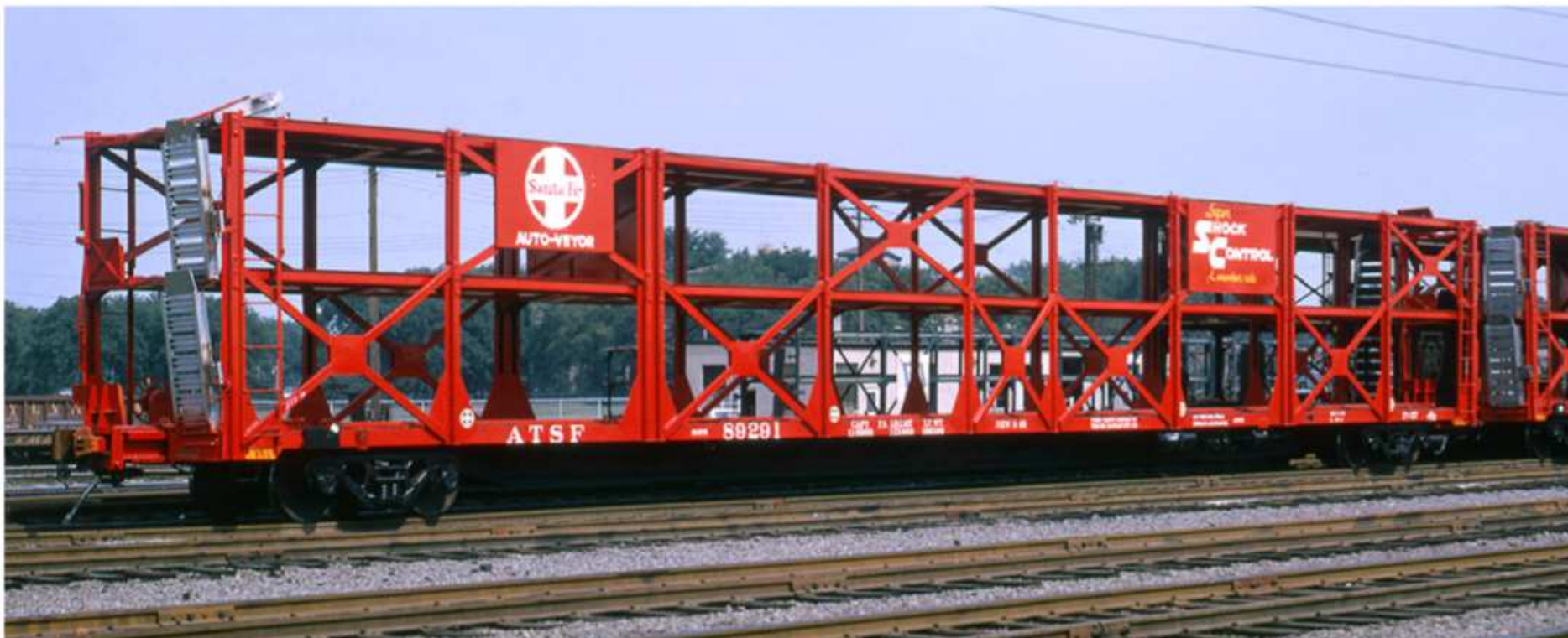
8 The Atchison, Topeka & Santa Fe Ry. built many of its own auto racks and flatcars. This 87-foot class Ft-27 tri-level car with cushion underframe was built in 1963. J. David Ingles collection
