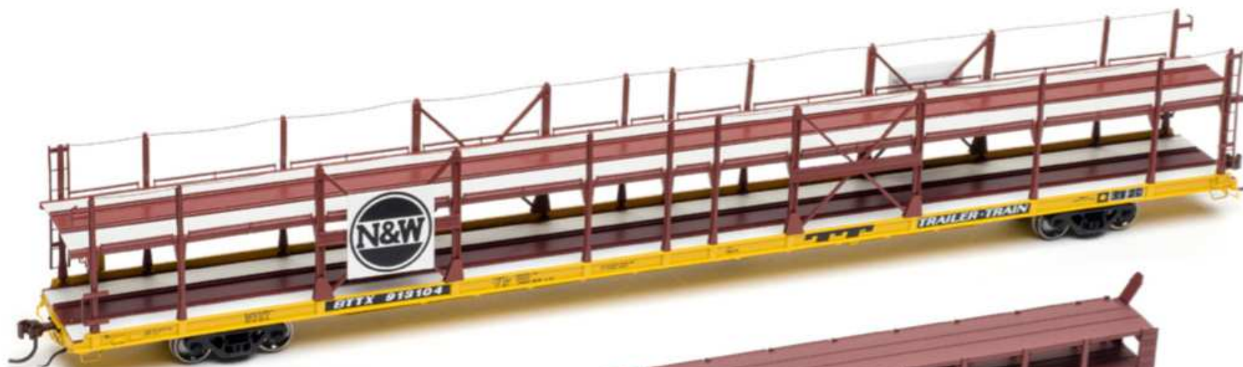
Athearn made a bi-level auto rack in HO (top), and Micro-Trains made a tri-level car in N (bottom). Bill Zuback
