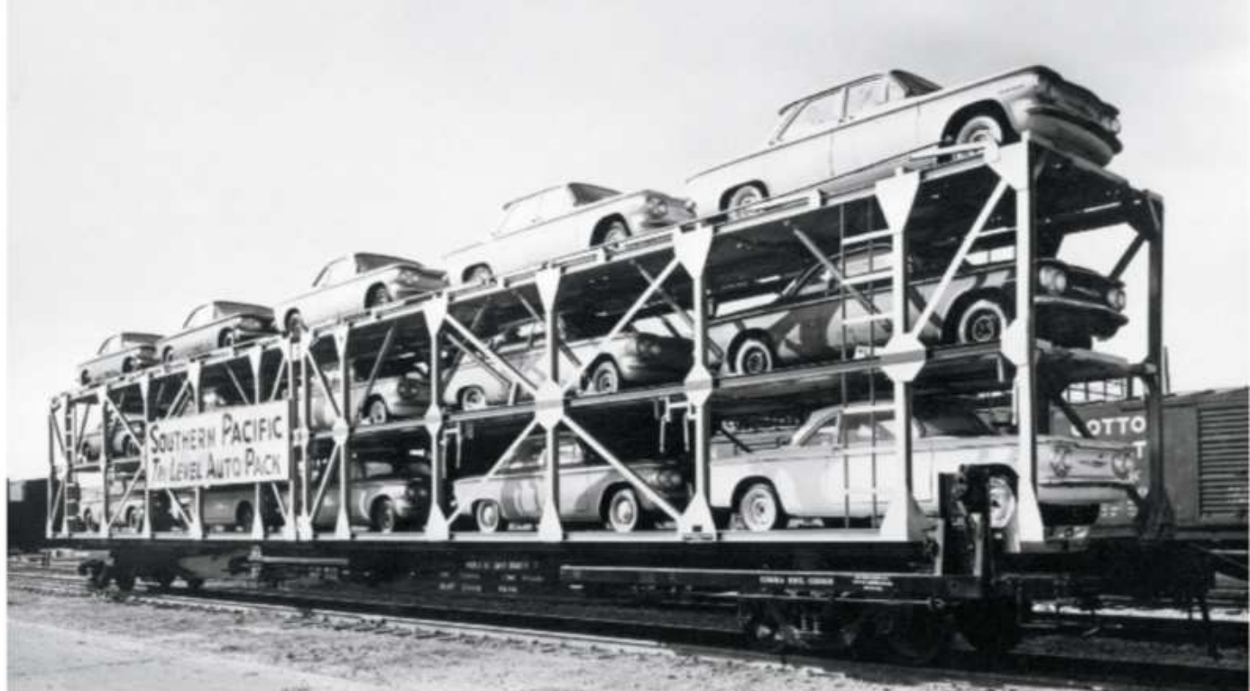
5 Whitehead & Kales, which would become the dominant rack builder, delivered its first production racks to Southern Pacific in 1960. The 85-foot car carries a load of 15 new Corvairs on its first run. Southern Pacific
