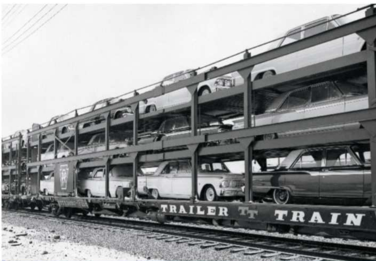
8 The Atchison, Topeka & Santa Fe Ry. built many of its own auto racks and flatcars. This 87-foot class Ft-27 tri-level car with cushion underframe was built in 1963. J. David Ingles collection
