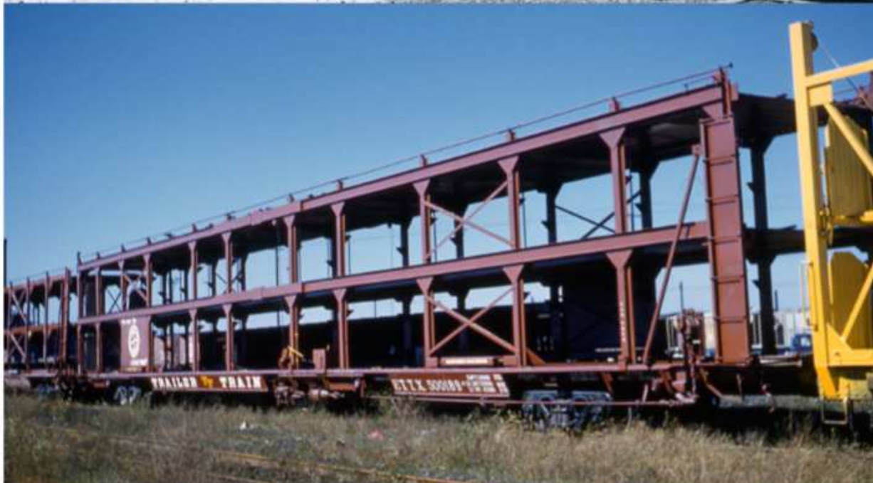
9 The middle and upper decks of this loaded Pennsy elevating rack car (a Paragon Lo-Hi-Tri) have been lowered for transit (top photo). For loading and unloading, the decks are at the levels of the horizontal framework, as on the empty Detroit, Toledo & Ironton Lo-Hi-Tri (bottom photo). Pennsylvania RR; J. David Ingles Collection
