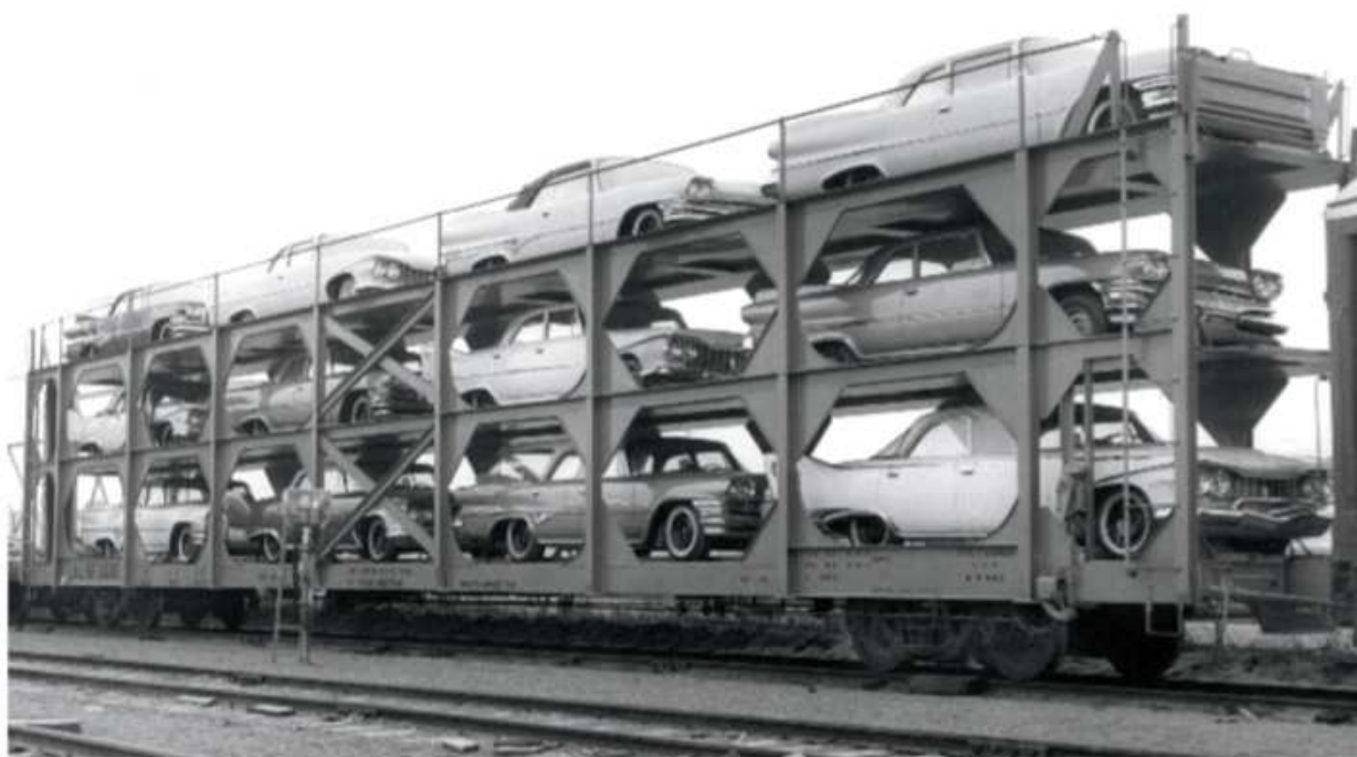
④ Shown with a load of new Fords, Frisco no. 3000 was the prototype long (83-foot) tri-level auto rack, built by Pullman-Standard in January 1960. Later production cars didn't have the curved and angled gussets. Pullman-Standard
