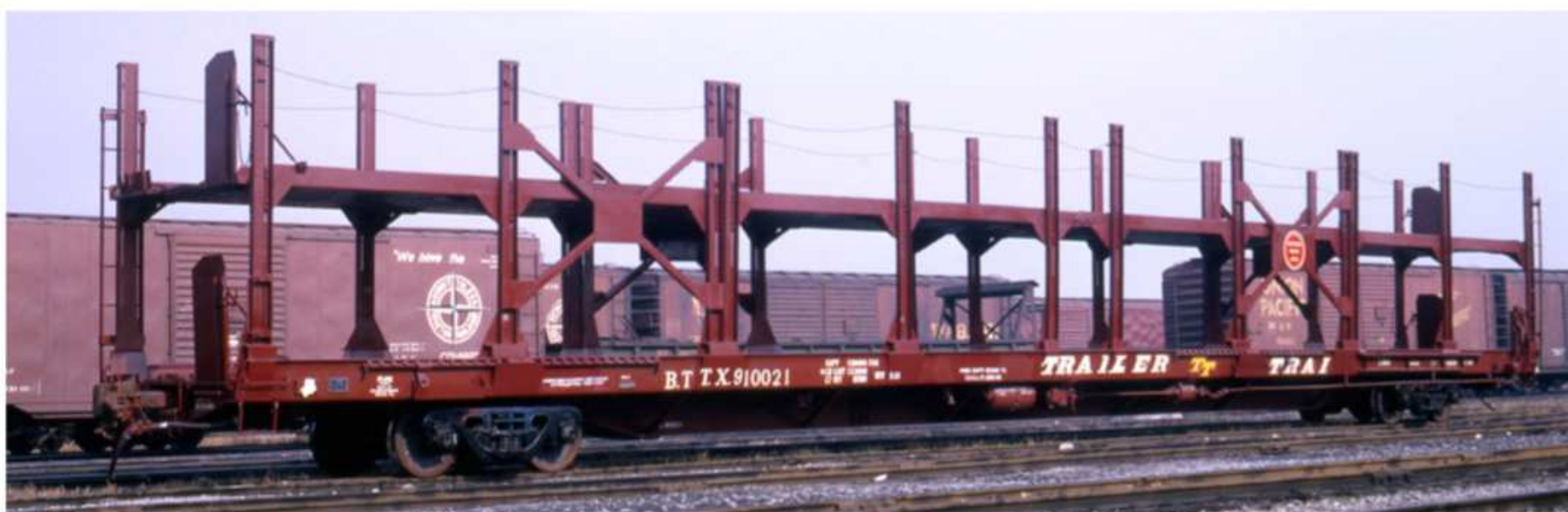
6 This 89-foot Missouri Pacific Paragon bi-level rack was mounted on a Trailer Train Pullman-Standard flatcar in 1963. Bi-levels were outnumbered by tri-levels more than 3:1 through the mid-1960s. J. David Ingles collection
