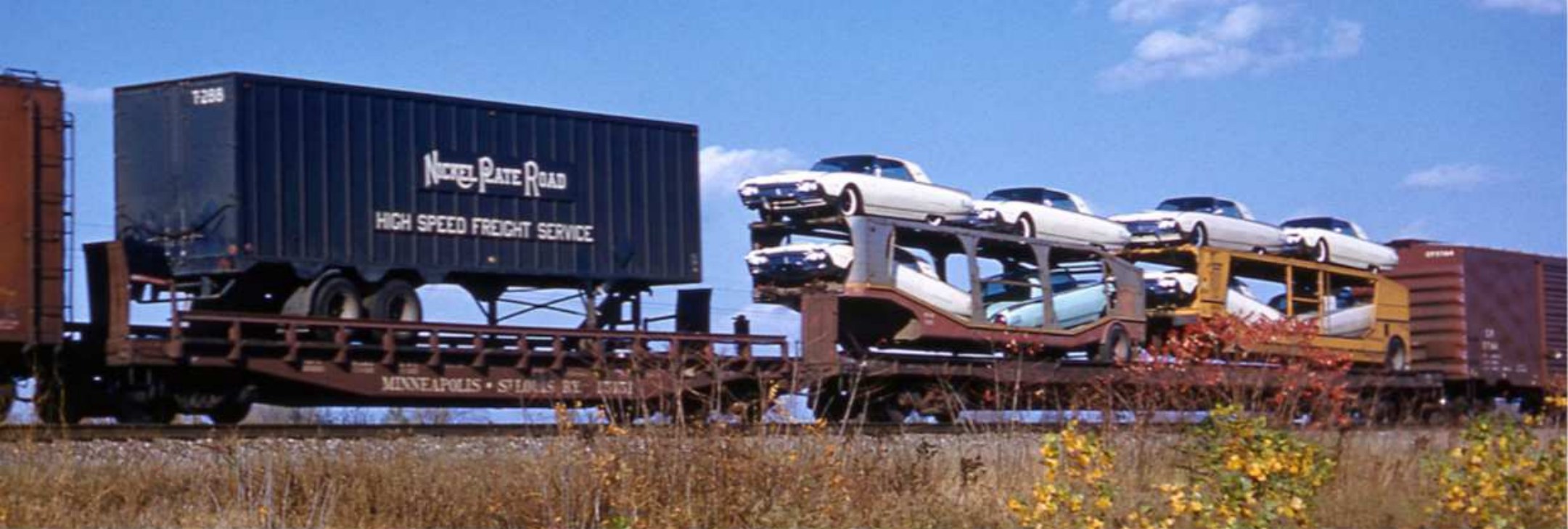
② Carrying autos by piggyback was the railroads' first attempt to regain the business from the trucking industry. "Haulaway" trailers on flatcars, such as this one carrying Ford Thunderbirds, were common from 1960 to about 1963. J. David Ingles collection
