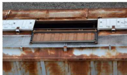
14 A close-up shot of the prototype shows that the corrugated metal hatch has ridges on the inside and a gasket around the rim.
