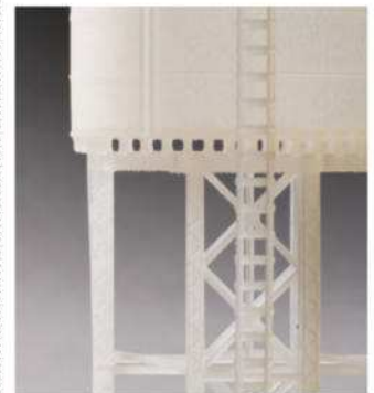
See-through detail such as the joists supporting the tank are possible in one piece with 3-D printing.
