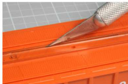
⑤ Several light passes of the hobby knife separated the edges of the area to be opened without damaging the sides of the trough.
