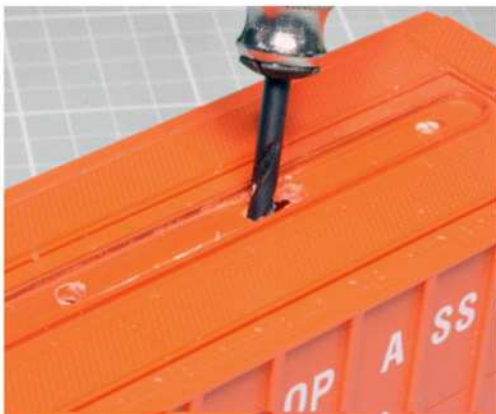
6 M.R. drilled out the ends of the trough area he intended to open, then used a hobby knife to scribe the sides of the opening.
