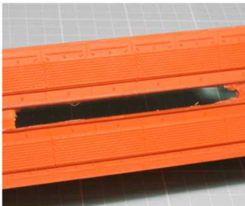
7 The hobby knife and drill M.R. used to remove a section of the trough floor left a rough opening.
