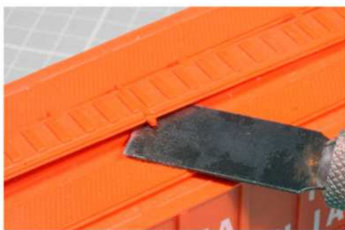
② M.R. used a chisel-bladed utility knife to carefully pry off the separately molded trough hatch cover.
