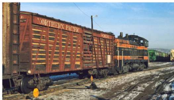
The new plywood attached from the inside stands out against the weather-beaten slats on Northern Pacific stockcar no. 83034. Bill Bedell photo, Bob Wazniak collection
