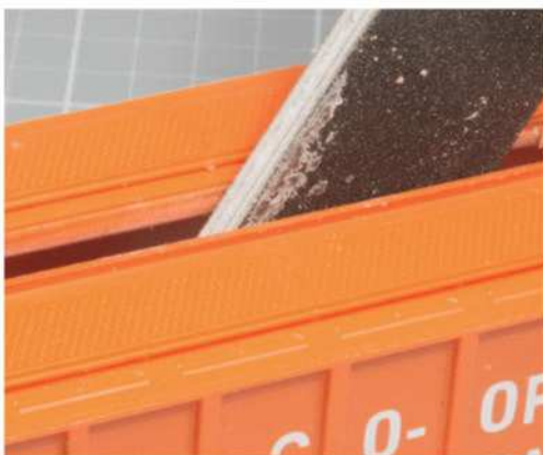
8 M.R. used a succession of increasingly finer-grit files and sanding sticks to clean up and square off the opening.
