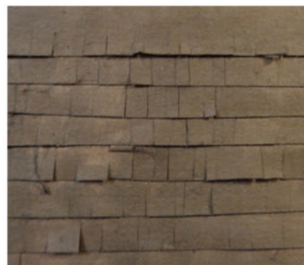
② Random widths. Varying the number of washers between each blade results in shingles with random widths.
