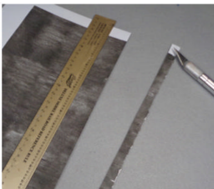
5 Slice and dice. Use a straightedge and a hobby knife to cut the shingles into strips.
