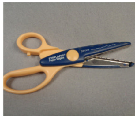
③ Deckle scissors. A pair of craft scissors cuts a ragged edge that makes more rustic-looking shingles.
