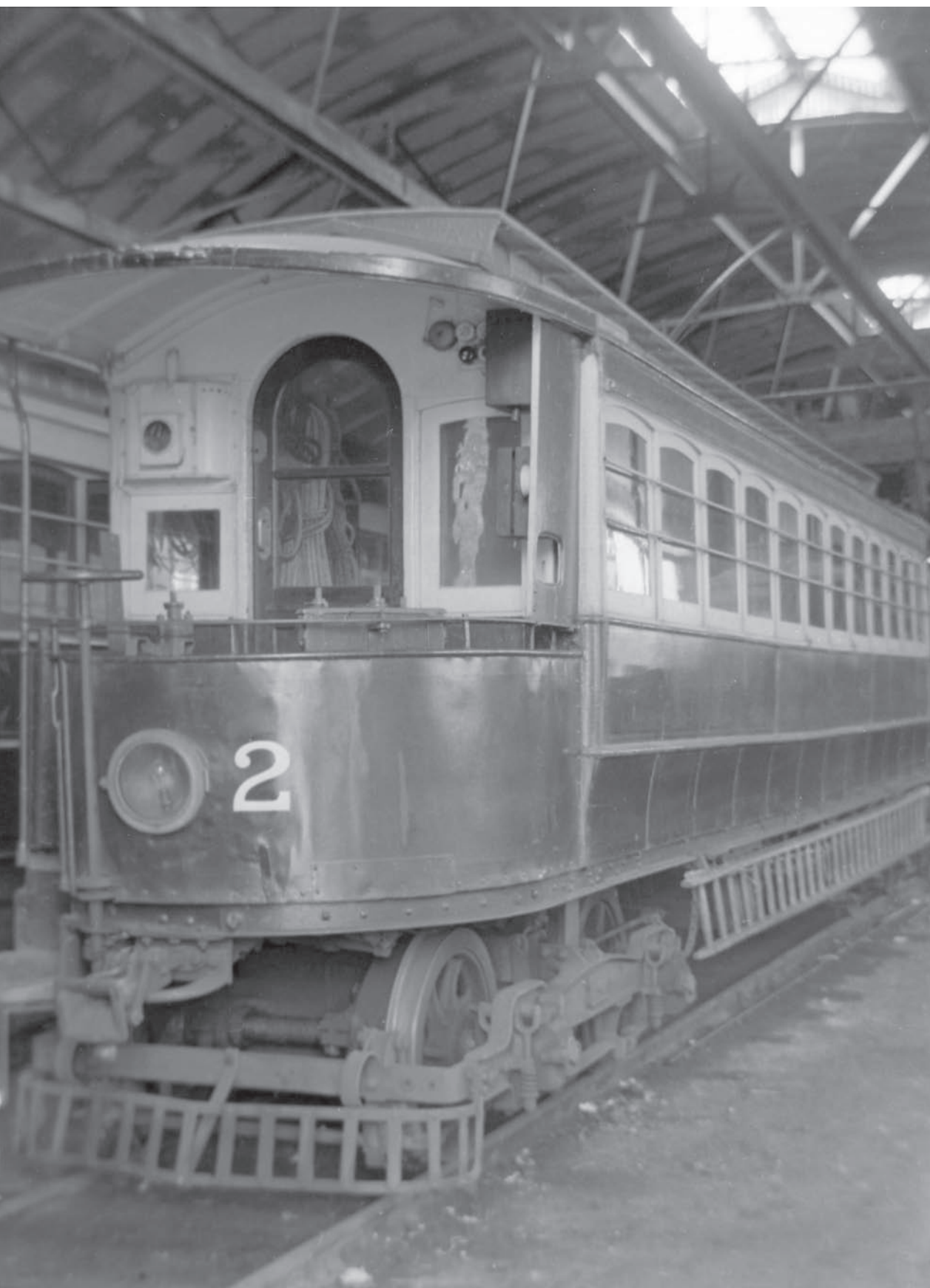
MER No 2 was one of three trams supplied in 1893 for the opening of the first section of the line; it is seen here inside the depot at Laxey on 9 April 1950. Note the ladder carried on the side; this was needed when the car was used by the overhead line department for work duties. Tony Wickens/Online Transport Archive
