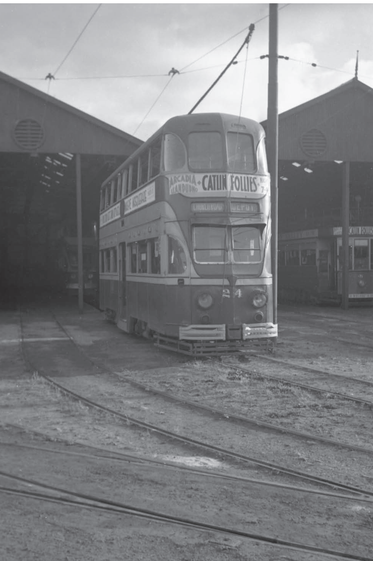
Undoubtedly the most modern 4ft 0in gauge trams built, Darwen Nos 23 and 24 were to have their numbers switched when converted to operate on the 3ft 6in gauge L&CBER. Here No 24 stands outside the depot at Rhos-on-Sea. R.W.A. Jones/ Online Transport Archive
