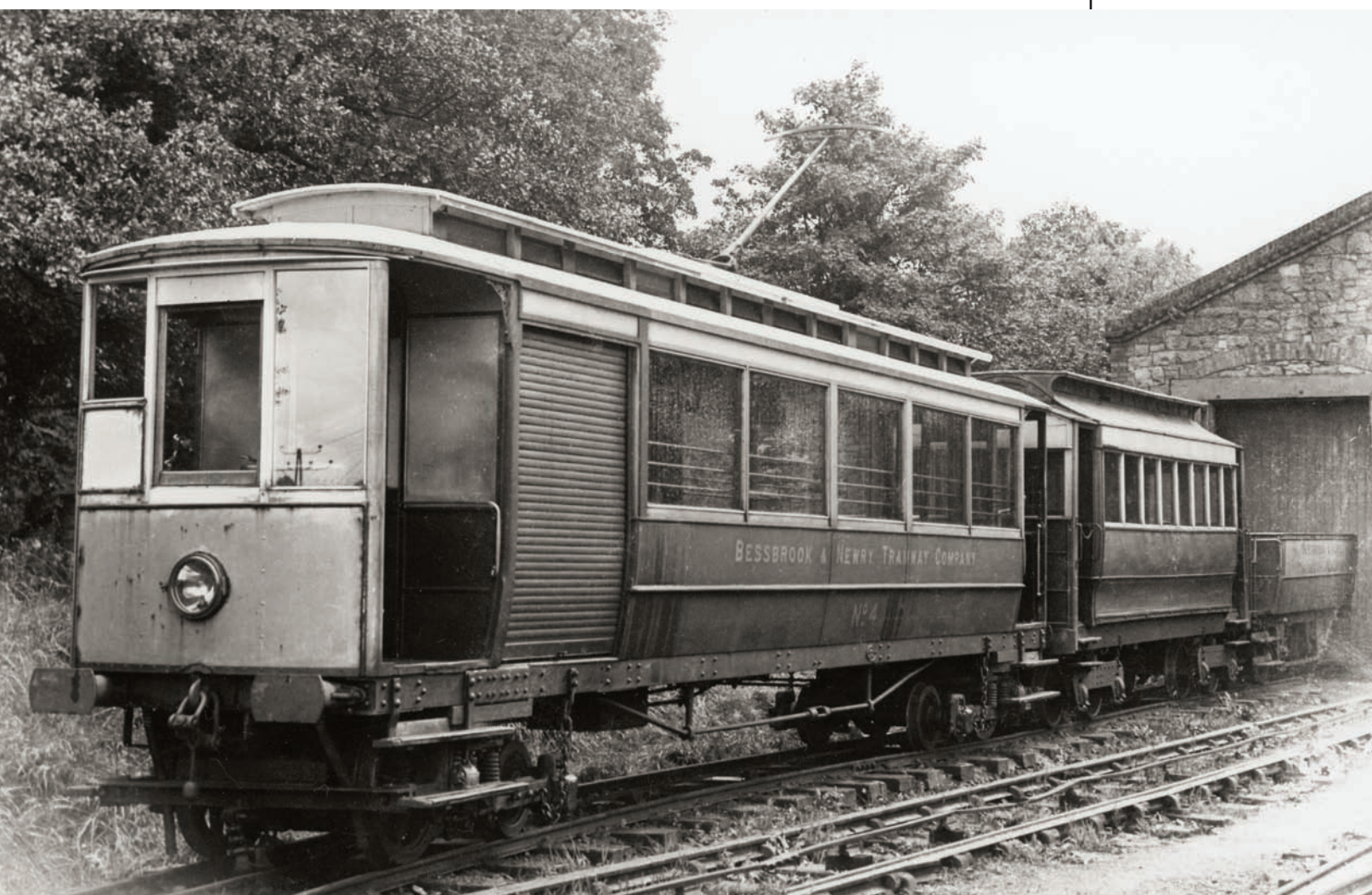
Bessbrook & Newry No 4 was originally built by Hurst Nelson in 1920; it received replacement maximum traction bogies seven years later. Barry Cross Collection/Online Transport Archive
