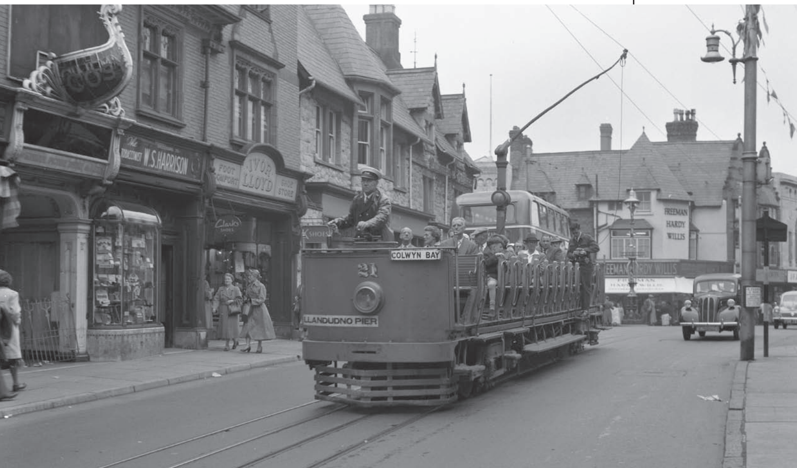
Part of the street section through Colwyn Bay was provided with interlaced track; here one of the quartet of toast-rack cars supplied in 1920, No 20, heads west from the Colwyn Bay terminus over this section. Phil Tatt/Online Transport Archive
