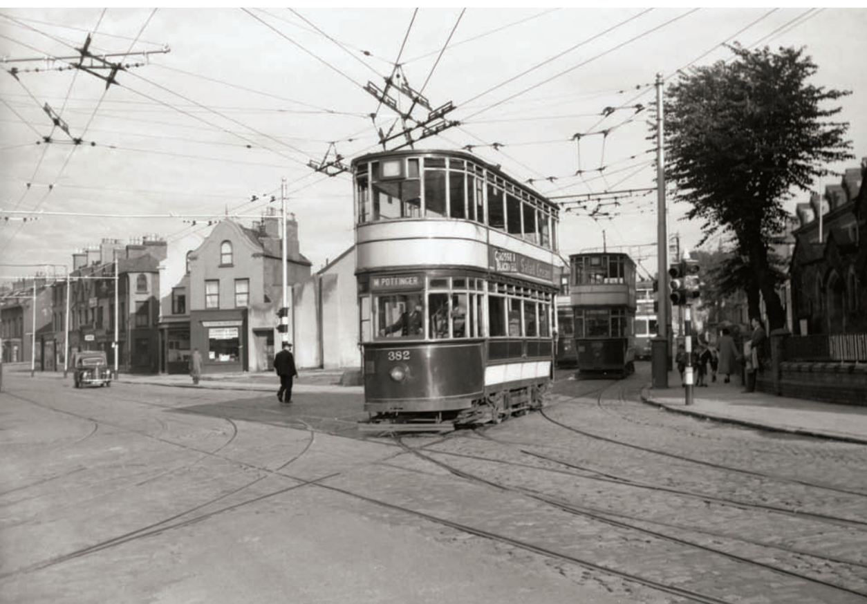
The first of the Service Motor Works-built 'Chamberlain' cars, No 382, crosses the complex but partly disused junction at Mountpottinger heading into Mountpottinger Road from Castlereagh Street. At this point, the trams used the trolleybus overhead. R.W.A. Jones/Online Transport Archive
