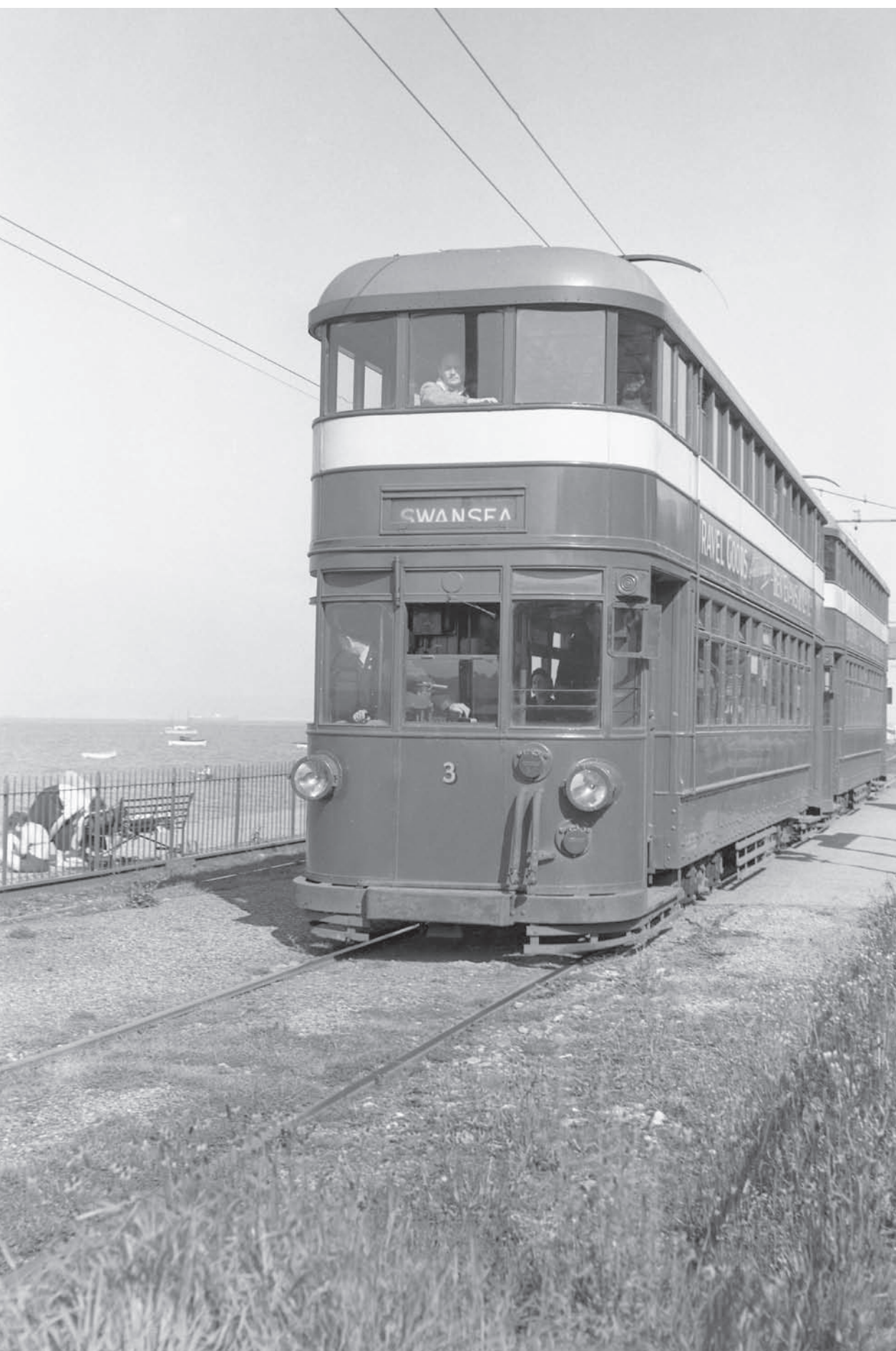
Swansea & Mumbles No 3 was one of 13 massive double-deck cars supplied by Brush for the electrification of the line. D. Kelk/Online Transport Archive
