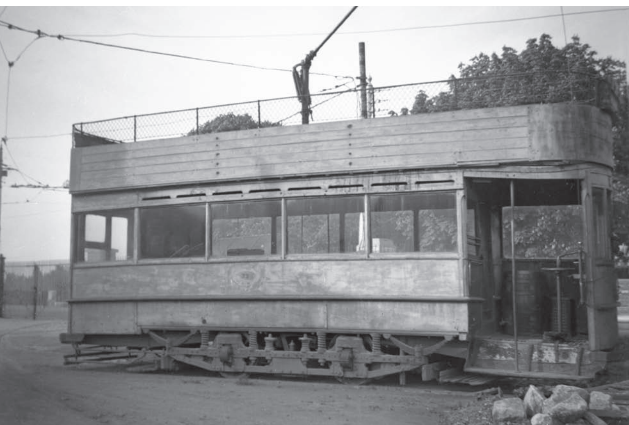
The history of Dublin's works fleet is complex but the majority had been withdrawn before CIÉ acquired DUT. One of the survivors was No 73; this was a railgrinder that had been converted from one of the late nineteenth century Milnes-built cars. Phil Tatt/Online Transport Archive
