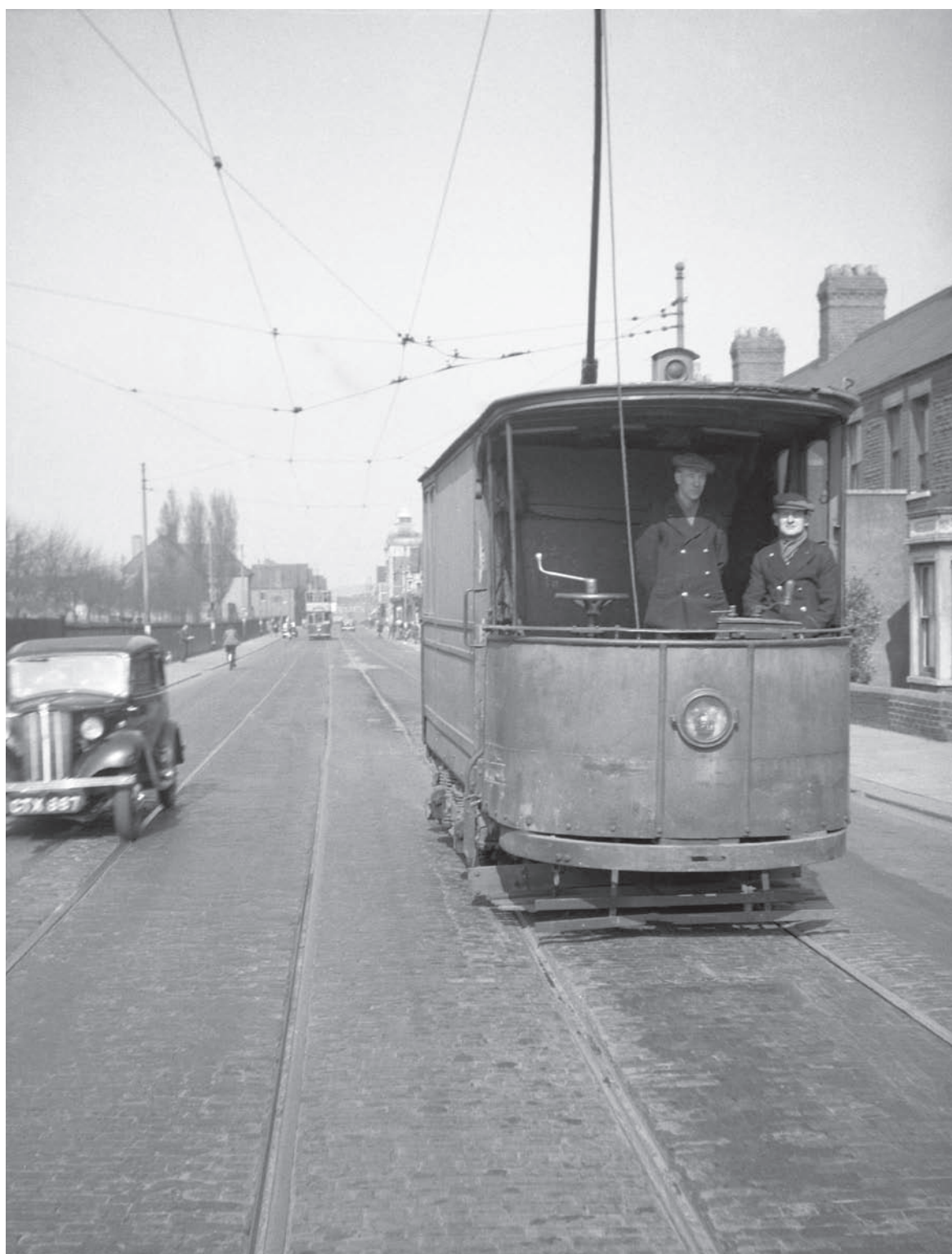
Works car No 131 dated originally to 1902. Preserved following withdrawal, it is seen here at the Talygarn Street crossover on Sunday morning whilst undertaking railgrinding duties on 31 March 1946. Ian L. Wright/Online Transport Archive
