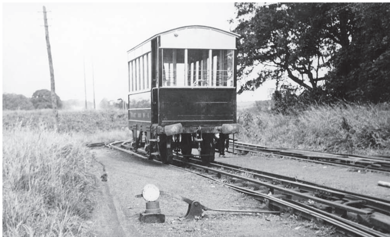
Acquired from the Dublin & Lucan line in 1928, Bessbrook & Newry No 5 was a trailer car. It is pictured here still in its Dublin & Lucan livery of green and cream, in which it operated for a number of years and prior to modification in which alternative windows were blanked out. W.A. Camwell/NTM
