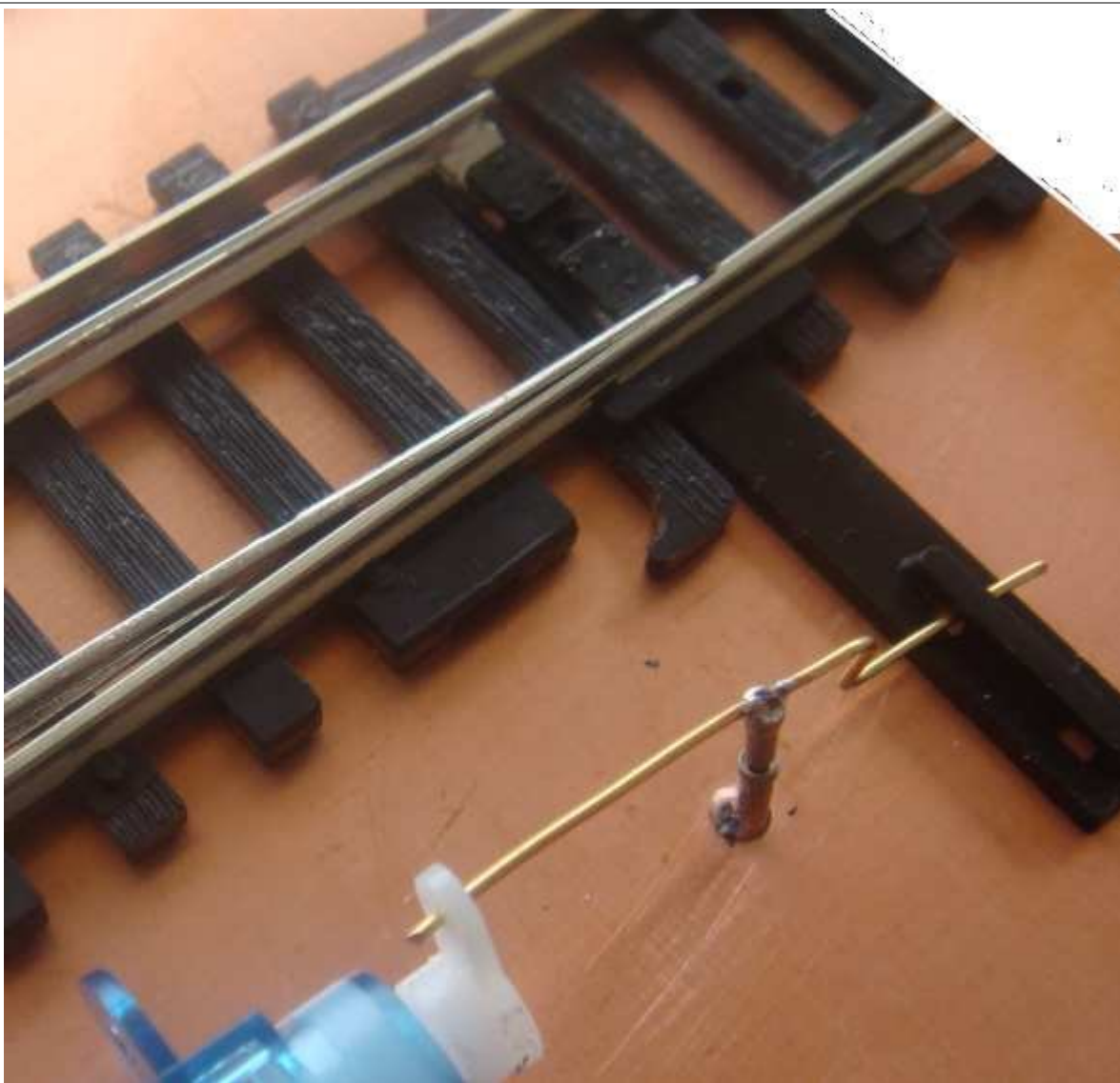
The Machine pin in the centre of the linkage acts as a pivot and the "crank" in the lever is simply to align the activating arm to the lever on the track.
