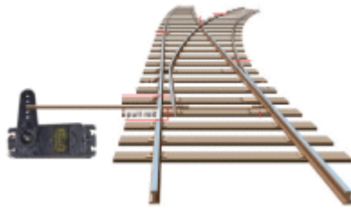
Fitting the Servo to the track
