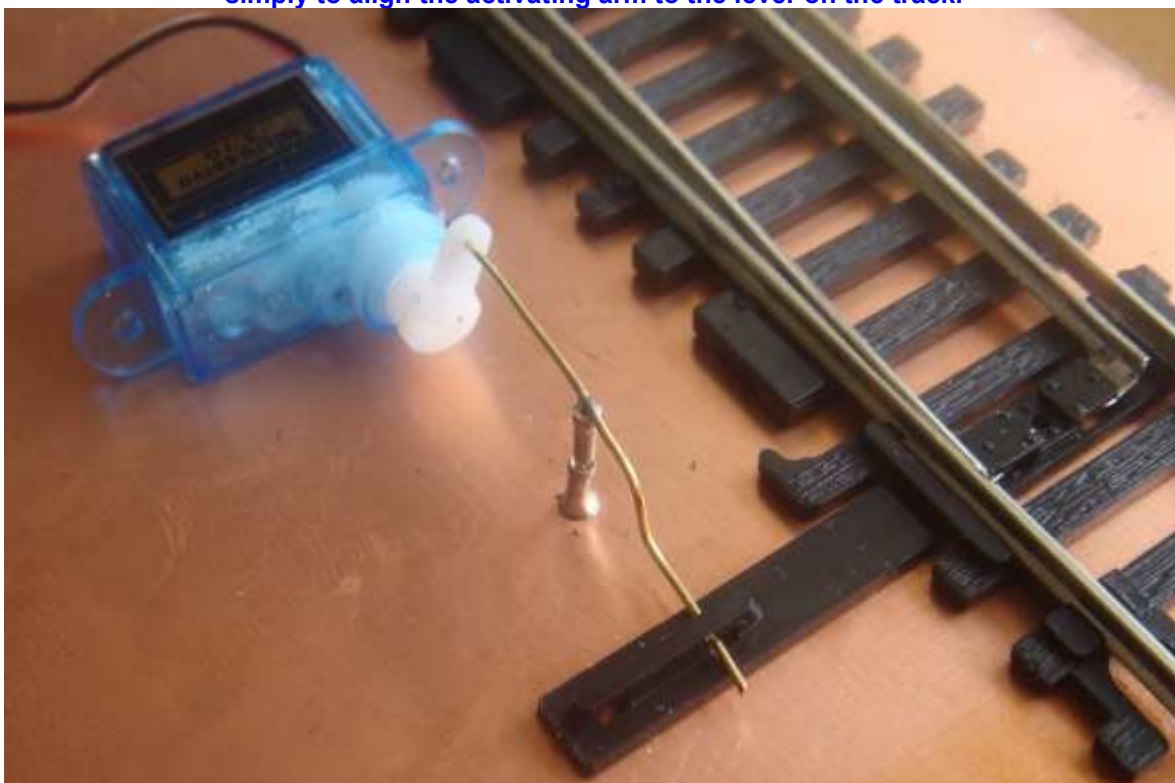
The Machine pin in the centre of the linkage acts as a pivot and the "crank" in the lever is simply to align the activating arm to the lever on the track.
