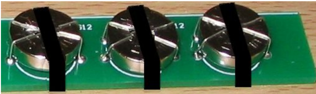
The 3 button cells are held in place with narrow heatshrink after soldering fine tinned copper wire over the cells. You can then cover the cells with duct tape.
