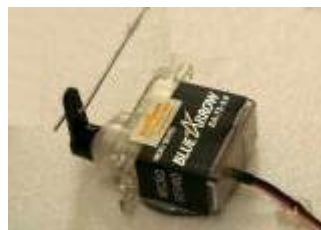
Connecting the push-rod
