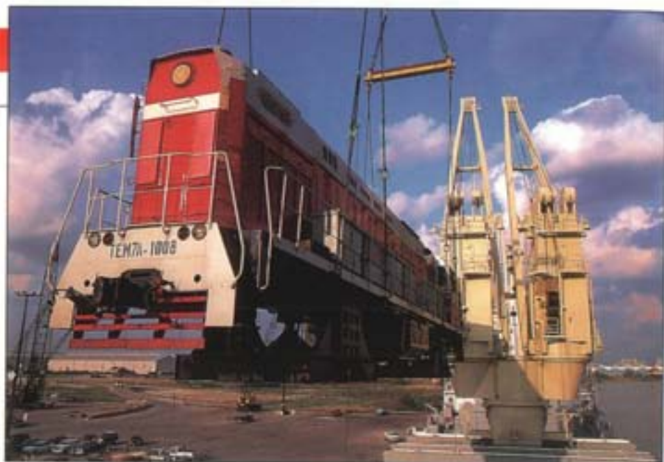
Big John, a floating derrick crane, lifts one of 11 Russian-made locomotives from a vessel at Wharf 32 in the Turning Basin. This discharge demonstrated the versatility of the terminal.
