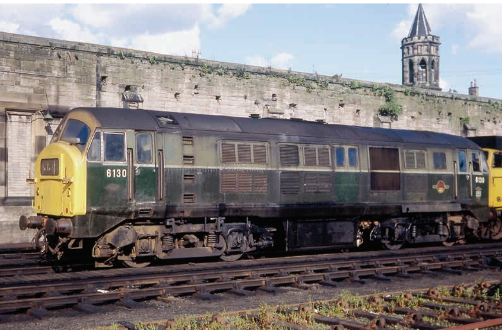
6130, Perth Stabling Point, 29 May 1971. A St.Rollox Works conversion – horn cover plates attached by rivets, thick main radiator grille strap. Note the total lack of 25kV warning signs and the roof-mounted rotating extractor fans to enhance engine cooling. (RCTS Archive)
