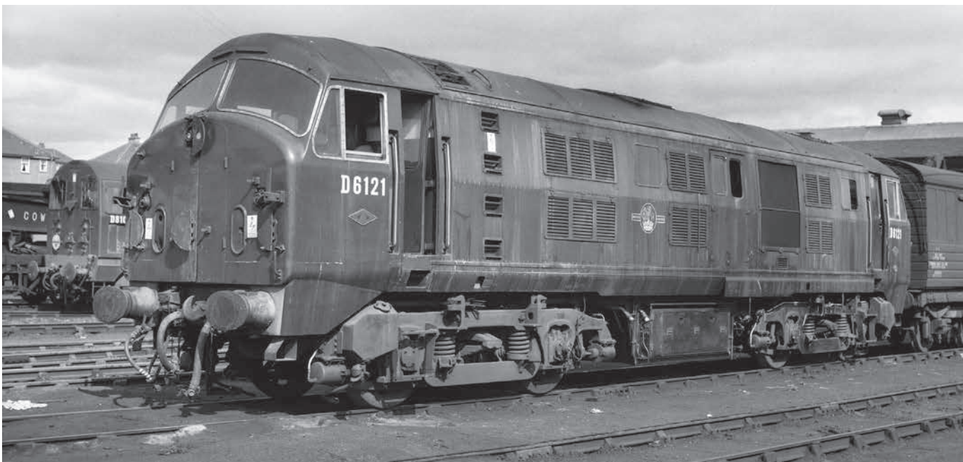
D6121, 65A Eastfield, 6 August 1963. The original D6121, and the last Class 21 built with cab roof air vents. (David Dippie)
