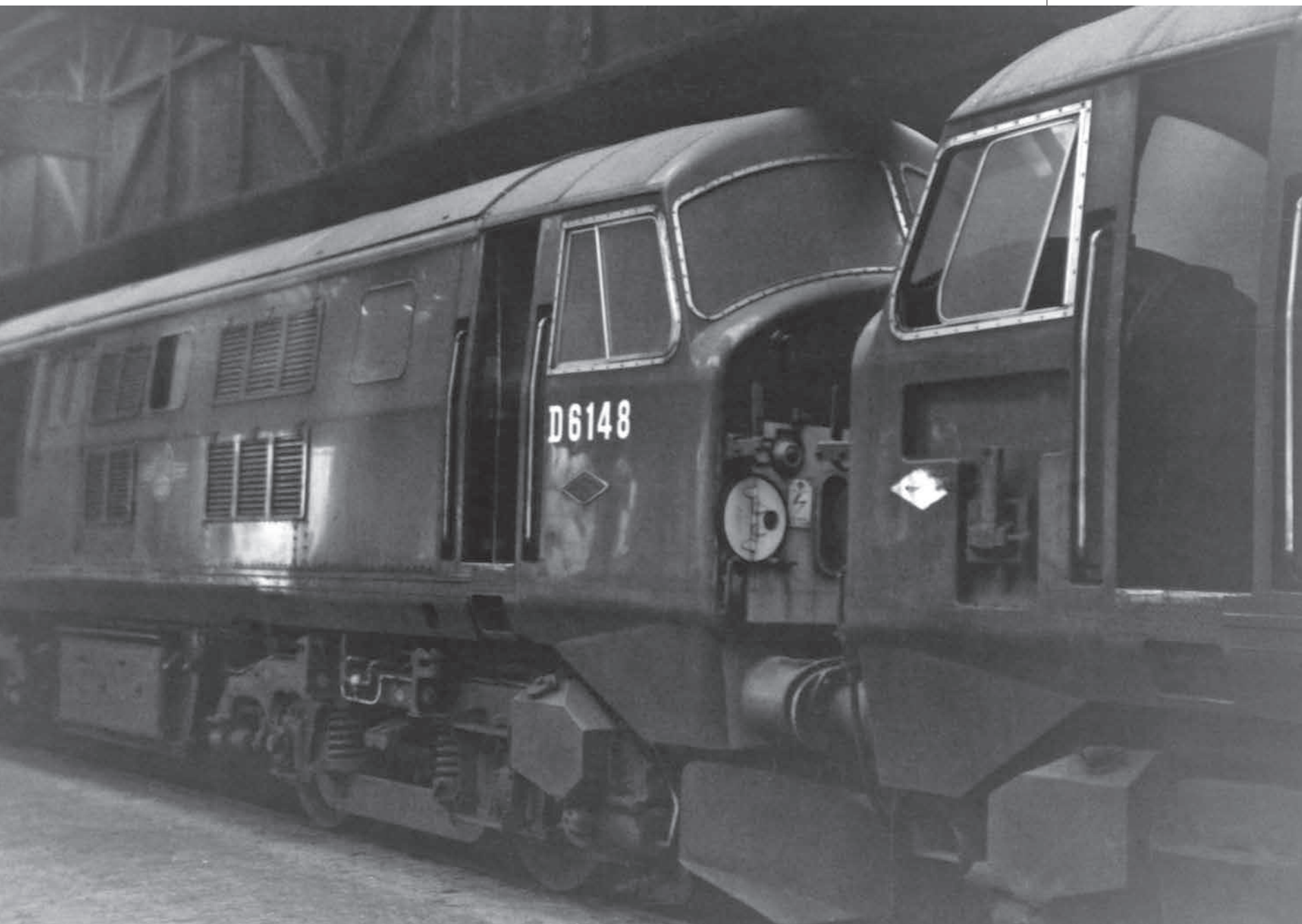
D6148, 63A Perth, 2 March 1968. Compare the footsteps on the GNoS Class 21 above with the triangular footsteps when fitted to the D6100-37 series; the orientation is reversed to allow miniature snowploughs to be accommodated. (Rail-Online)
