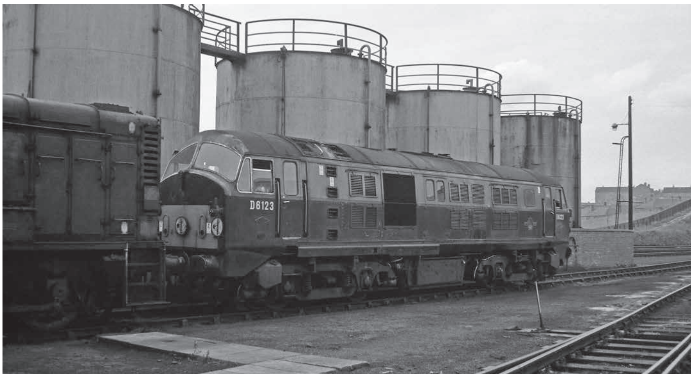
D6123, Location unknown, Undated. Somewhat ironically, the lion and wheel emblem has reverted to the as-built D6100-2 position, necessitated by the fitting of additional bodyside grilles. Black line just visible above the bodyside 'crease' line. (Rail-Online)
