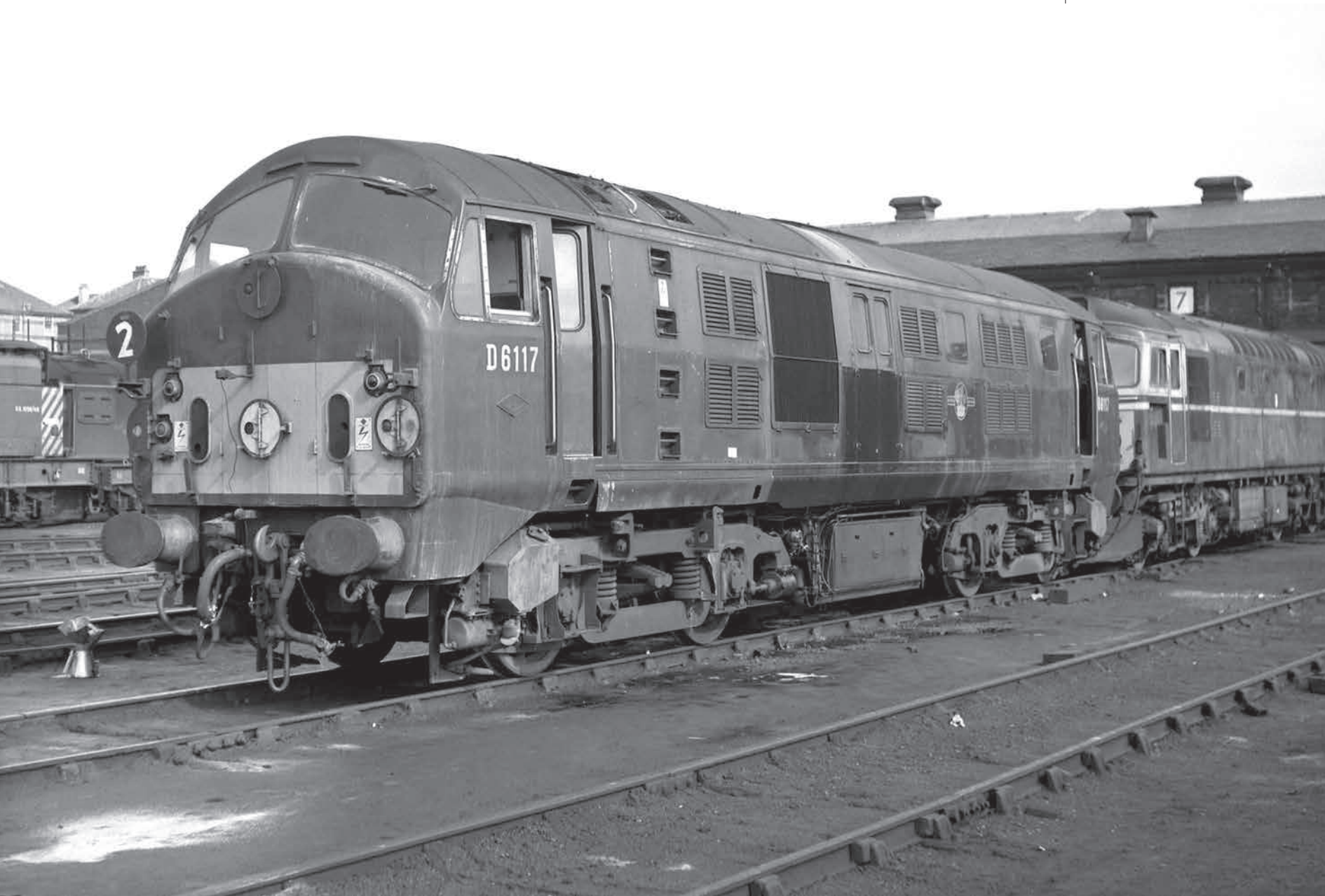
D6117, 65A Eastfield, 25 July 1968. D6117 with the remnants of the Cowlairs Bank slip-coupling system on the front ; see photograph of D6115 on page 71 for comparison. This locomotive was another member of the Class to receive a refurbished MAN engine at Inverurie in 1967. Along with D6111 and D6152, final withdrawal came in August 1968, rendering Class 21 operationally extinct. (RCTS Archive)
