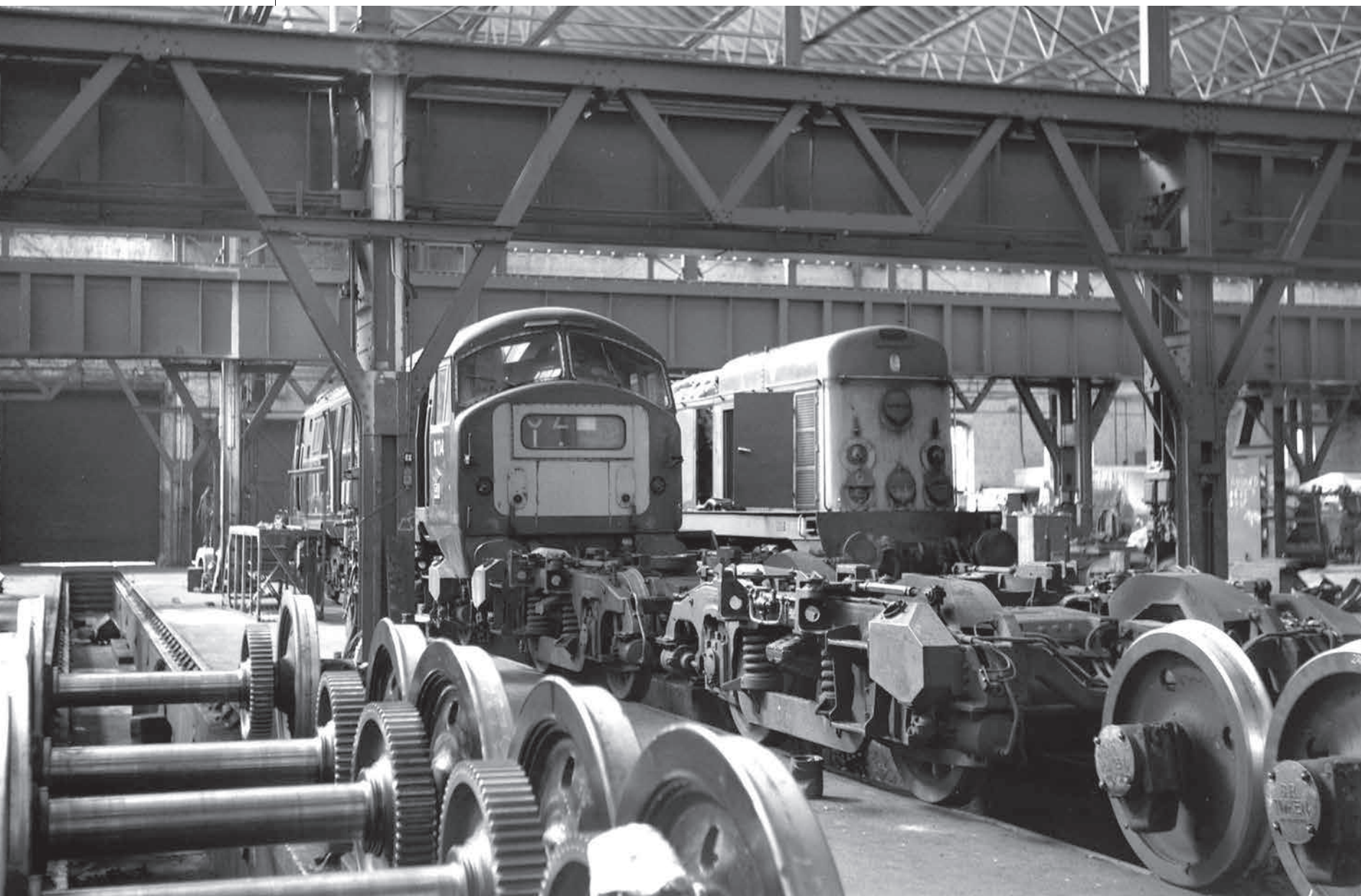
D6114, Inverurie Works, 15 July 1969. The DLRC for this loco indicates a period in works 24/04/69-07/08/69 for an Unclassified Repair. Note the two Class 29 bogies in the foreground; maybe a bogie swap for D6114 before final release back into traffic? (RCTS Archive)
