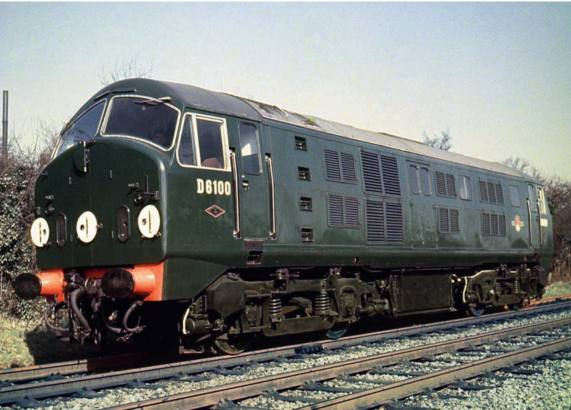
D6100, Royston, 1959. D6100 in original condition with first design of radiator grilles (applied to D6100-9 only), and the first style of the green livery with the emblem at the right hand end of the bodyside (D6100-2). From D6103 the emblem migrated to a more central position. The NBL diamond works-plate is evident at No.1 end, but not at the No.2 end. This little indiosyncrasy appears to have been the situation for D6100 upto at least D6103; two plates, one under each No.1 cab side window, subsequently became four works-plates one under every cab side window and D6100-3 (maybe higher) were modified to four retrospectively. (Colour-Rail)
