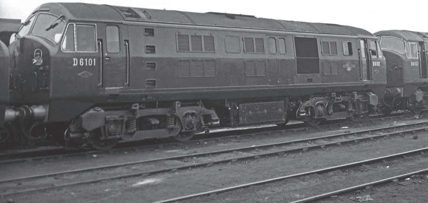
D6101, Hornsey MPD, 6 September 1959. The original radiator grille has already been replaced to improve engine cooling. (Colour-Rail)
