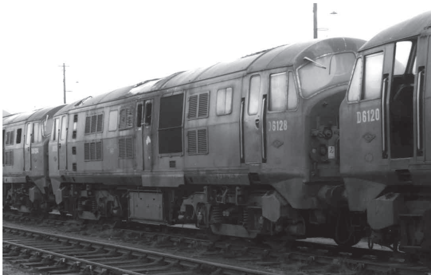
D6128, 61A Kittybrewster, 22 September 1966. The fire damage sustained by this locomotive adjacent to the MAN engine is clearly apparent. (Geoff Sharpe)
