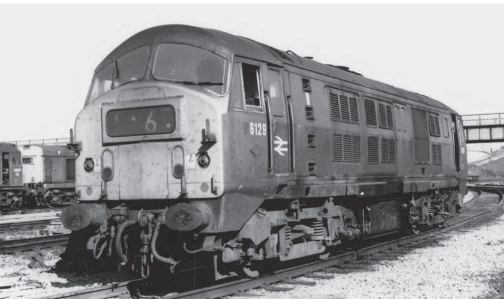
6129, 65A Eastfield, 11 September 1971. An Inverurie Works conversion – horn cover plates attached by grommets, thin main radiator grille strap. Standard set of six 25KV warning signs (three visible). (Norman Preedy)
