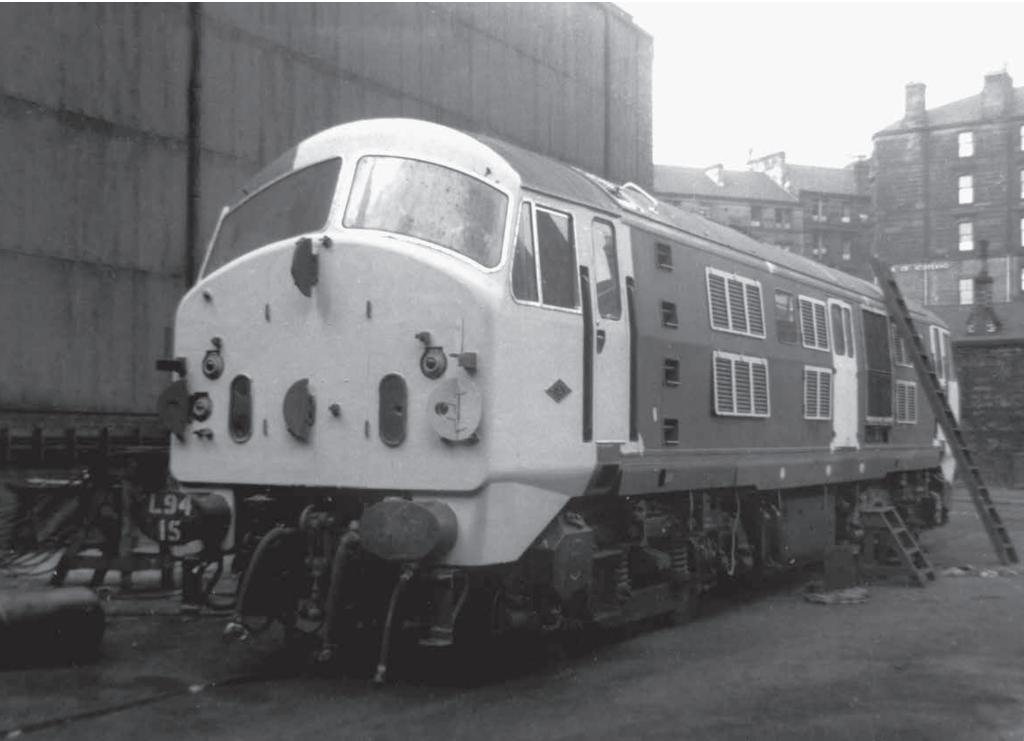
D6124, NBL Co., Hyde Park Works, Undated. 'L94 15' identifier on the left buffer i.e. 15th locomotive of Order L94. (Bill Hamilton)
