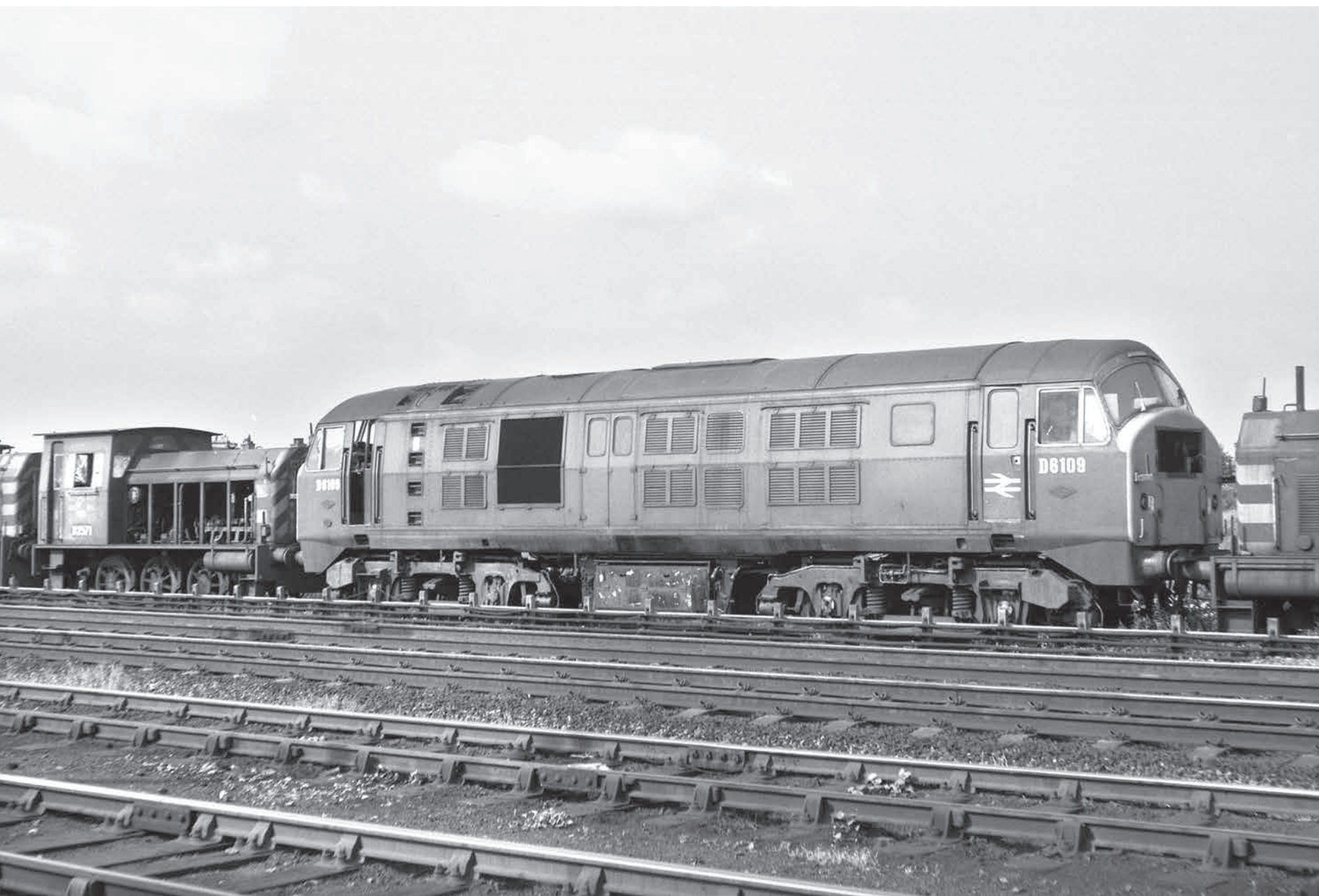
D6109, 65A Eastfield (Cowlairs Triangle), 25 July 1968. Another Class 21 which received a refurbished MAN engine in early 1967, the unique blue D6109 awaiting a tow to the scrapyard. Note the removal of the headcode box (actually removed from both ends). (RCTS Archive)
