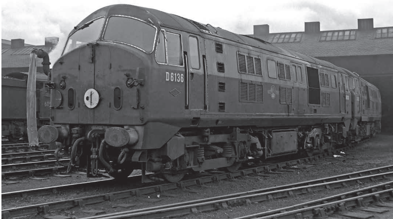
D6136 (with D6130), 61B Aberdeen Ferryhill, 8 July 1962. D6136 with the main radiator grille arrangement which became the standard for the whole class once D6100-9 had been upgraded. Note the Red Circle MW equipment on the buffer beam and the Beclawat droplight windows. (R. Conway [Rail-Online])
