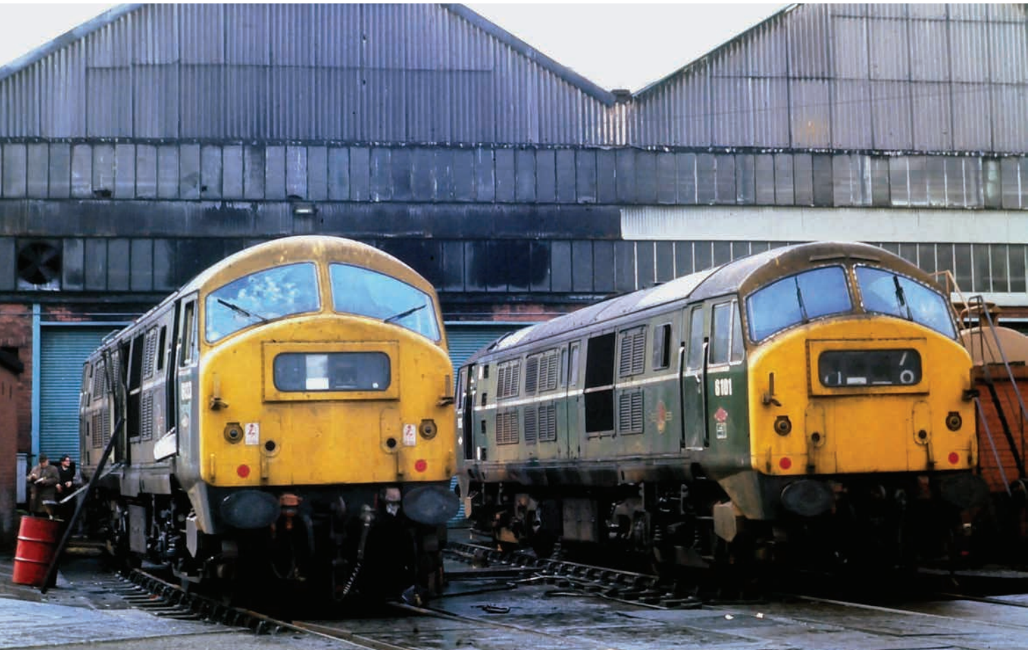
6133 and 6101, Glasgow Works, Erecting Shop Yard, 10 June 1972. Undergoing fluid removal prior to scrapping (lubricating oil, coolant and fuel). (Keith Holt)
