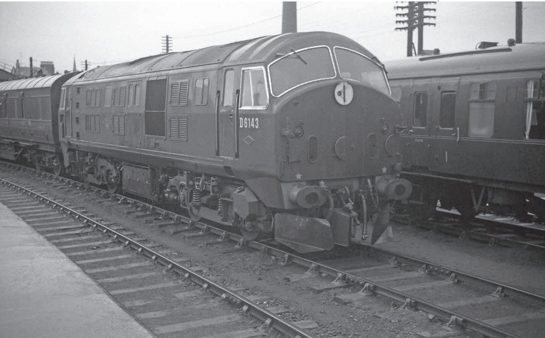
D6143, Inverness, 10 March 1962. Full complement of miniature snowploughs but no Manson tablet catcher in the recess. (Rail-Online)
