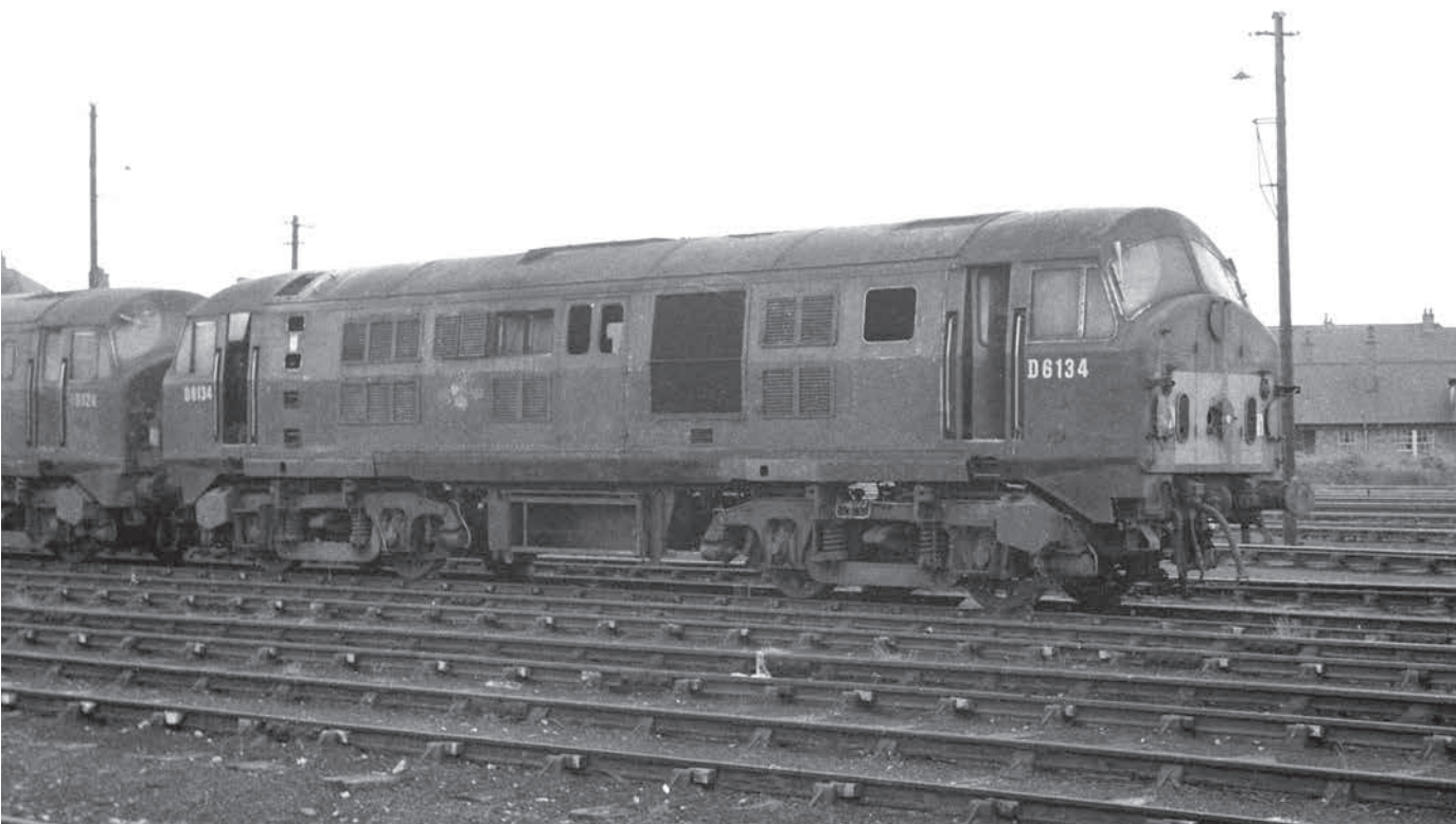
D6134, 61A Kittybrewster, Undated. The cut away corners to the buffer beams would suggest that this loco had been derailed with the holes cut to facilitate subsequent re-railing, presumably at some point after the fire damage sustained in February 1966. (Author's Collection)
