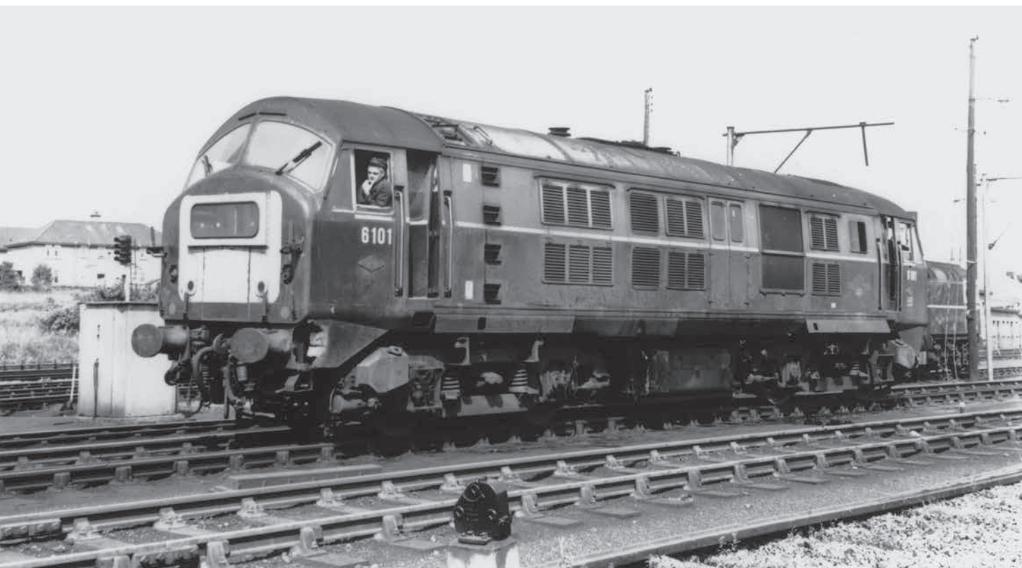
6101, 65A Eastfield, 10 March 1969. Over three years out of shops following Class 29 conversion and 6101 looks distinctly uncared for, with what appears to be a hole in nearest buffer valence and various pieces of metalwork missing from the lower bodyside. According to the DLRC, 6101 had to wait another year for further Works attention. As was frequently the case for St.Rollox Works converts, the 25kV signs were to be found in strange places; on 6101 there were none on the front and two on each bodyside to the left of the top and bottom boiler water tank access steps. (Norman Preedy)
