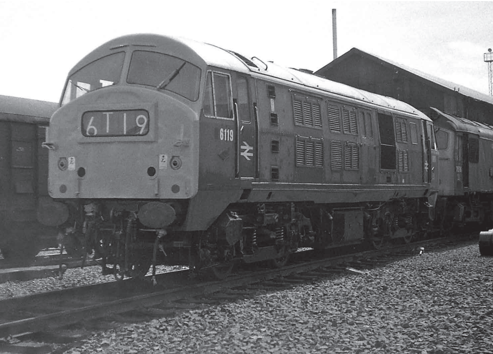
6119, 65A Eastfield, 4 September 1971. In ex-works condition and believed to be the last Class 29 to receive works attention. Note the repainted and slightly extended yellow ends, spruced up Inverurie-blue livery, and refurbished bogies. Ex-works in August 1971 and withdrawn four months later, but at least its works attention ensured survival to the end of Class 29 operational history. (Dave Jolly)
