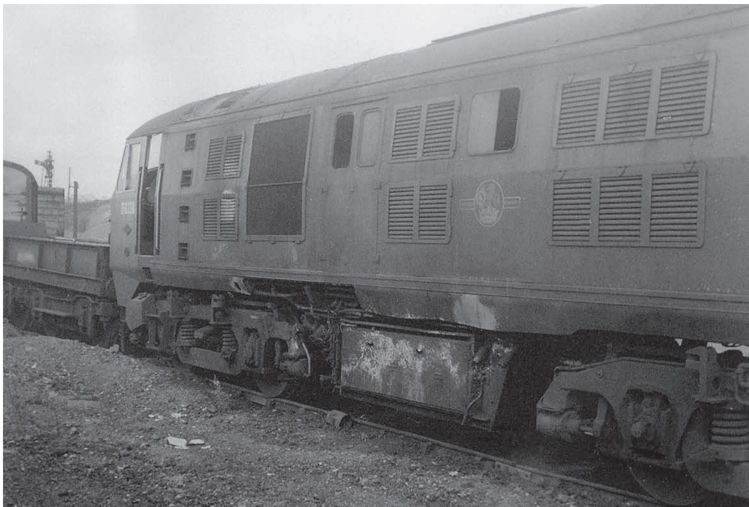
D6136, 65B St.Rollox, 28 July 1962. Close-up of the fire-damage sustained by D6136 at Forteviot on 14 July 1962. According to the DLRC repairs were undertaken at St.Rollox Works during the period 16 July to 18 August 1962, although clearly the early part of this period was actually spent "Waiting Works" at St.Rollox shed. (Bill Hamilton)
