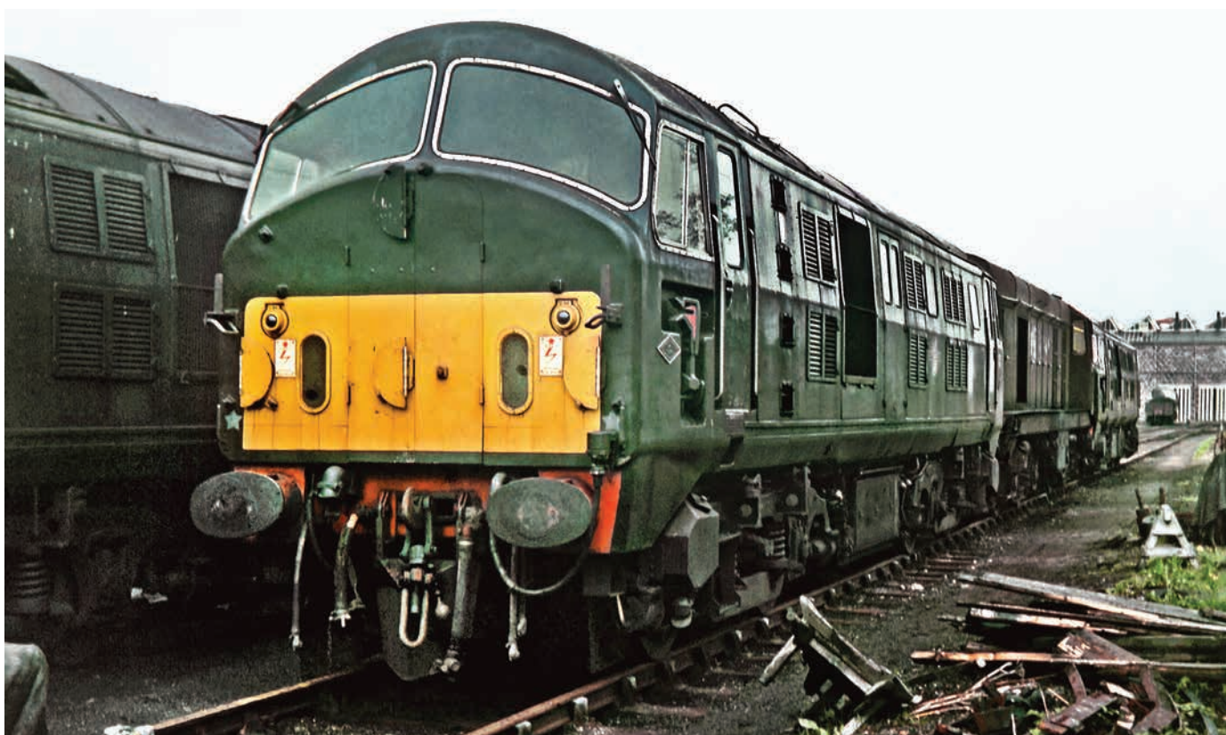
D6143, Inverurie Works, May 1966. D6143, one of the GNoS batch, featuring Blue Star MW equipment, sliding cab side windows and tablet catcher recesses (complete with Manson catcher). (G. Edgar [Rail Photoprints])
